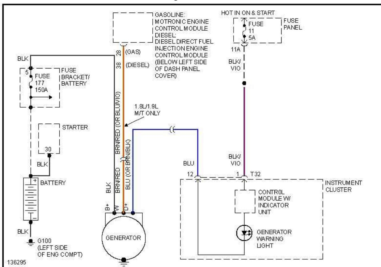
**BEETLE 1.9L L4 TURBO DIESEL 2001****Diagrama 1 de 1**
