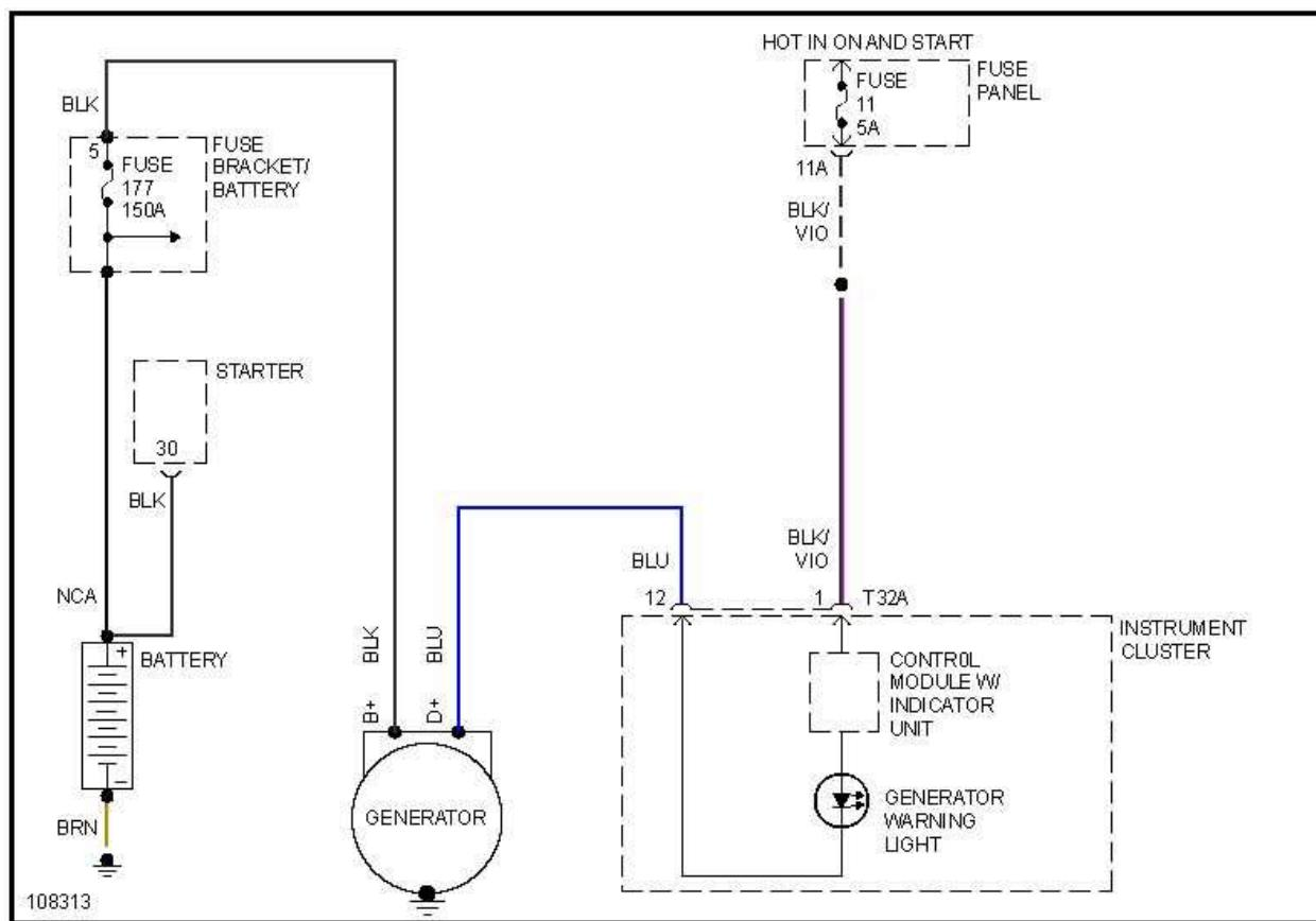
**BEETLE 1.9L L4 TURBO DIESEL 1999****Diagrama 1 de 1**
