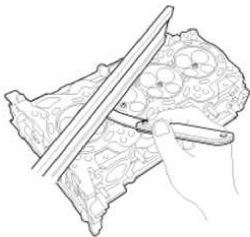
Fig. 71: Inspecting For Flatness
