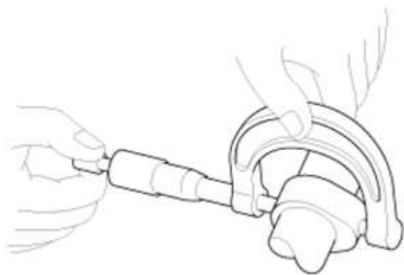
Fig. 78: Measuring Cam Lobe Height Courtesy of HYUNDAI MOTOR CO.
