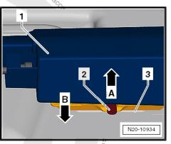
Disconnect lines from connections -T- ⇒ Item 4 (page 34) and -A- ⇒ Item 5 (page 34). Separate plug-in connectors ⇒ "3.1 Separating plug-in connectors", page 29.
