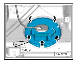
Check that connector -1- is fitted securely by pulling connector without pressing catch. If connector was not inserted correctly, repeat functional check of fuel pump.
