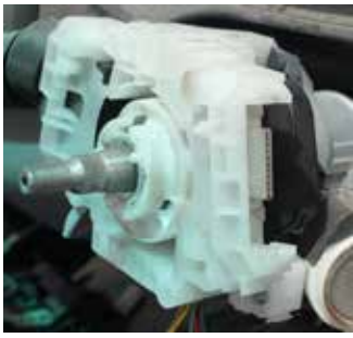
Steering Angle Sensor (ASTC only, behind steering wheel)
