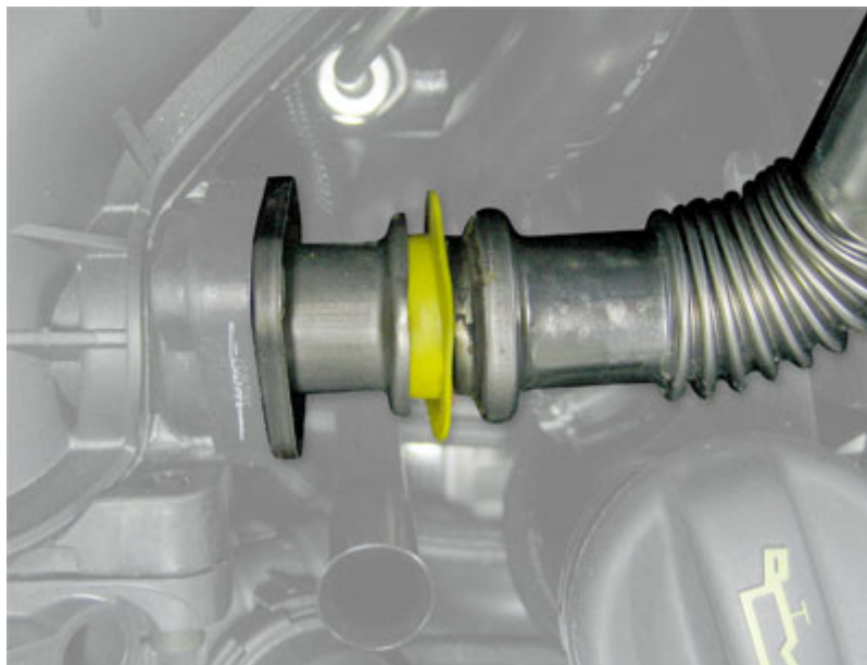
Figure 12: Isolation of the EGR pipe (SID 803 / 803A)
