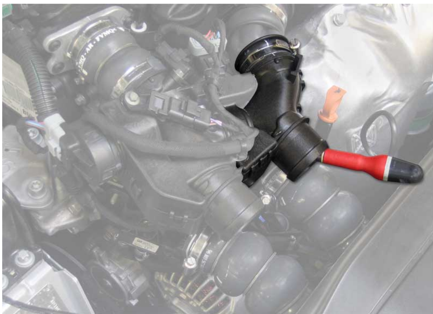
Figure 17 : inlet air heater throttle valve (RAA) operation (EDC16 C34)
