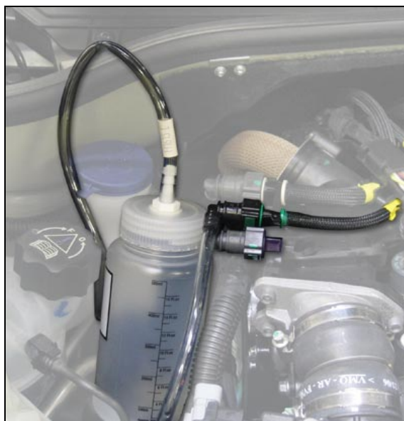
Figure 5 : Checking HP pump flow (EDC16 C34)
