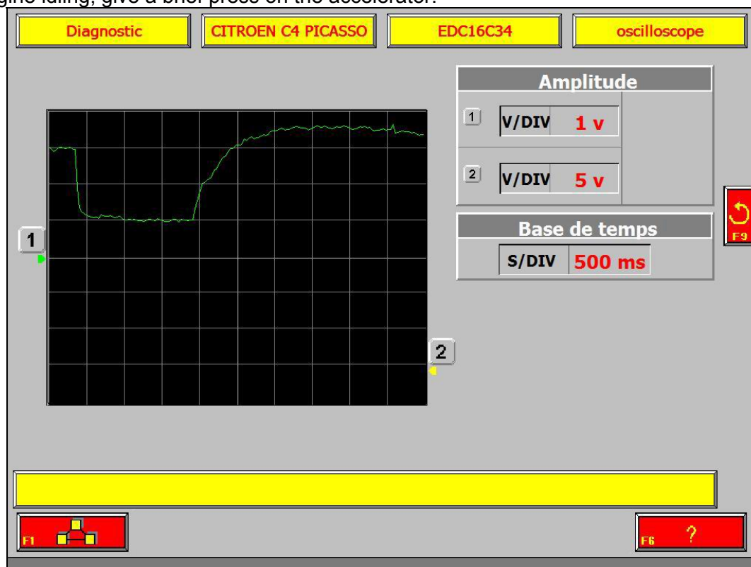
Figure 13 : Signal measured on valve feedback (EDC16 C34)
