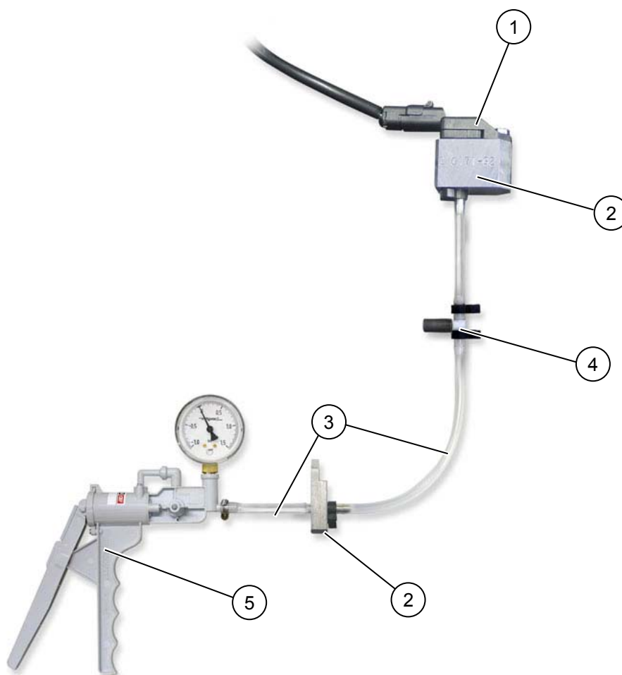
Figure 15 : Connection diagram for turbo pressure sensor check (EDC16 C34)
