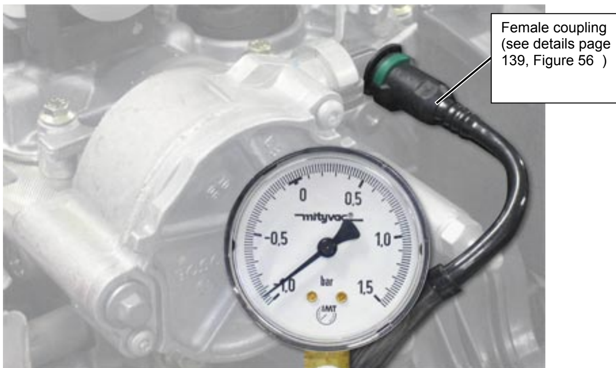
Figure 37: Vacuum pump check (EDC16 C34)
