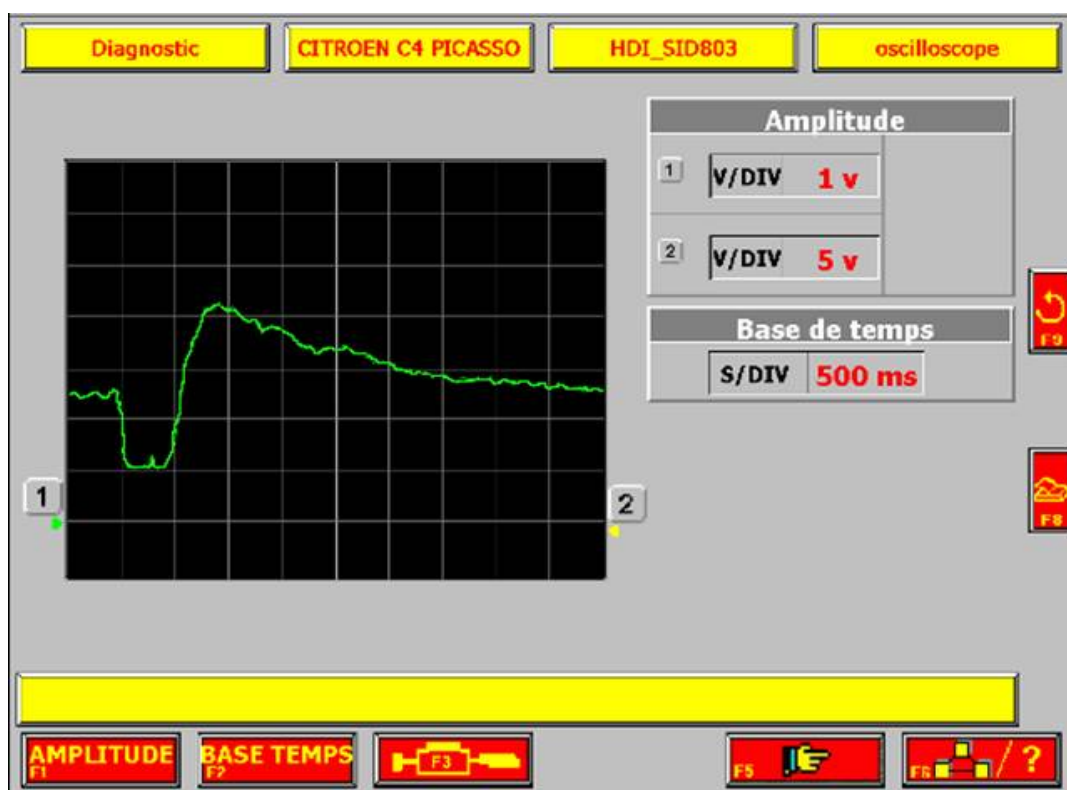
Figure 13: Signal measured on valve feedback (SID 803 / 803A)
