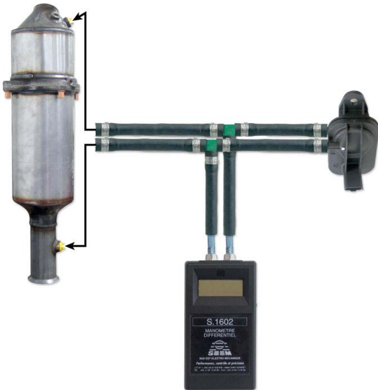
Figure 53: Illustration of the differential pressure sensor check
