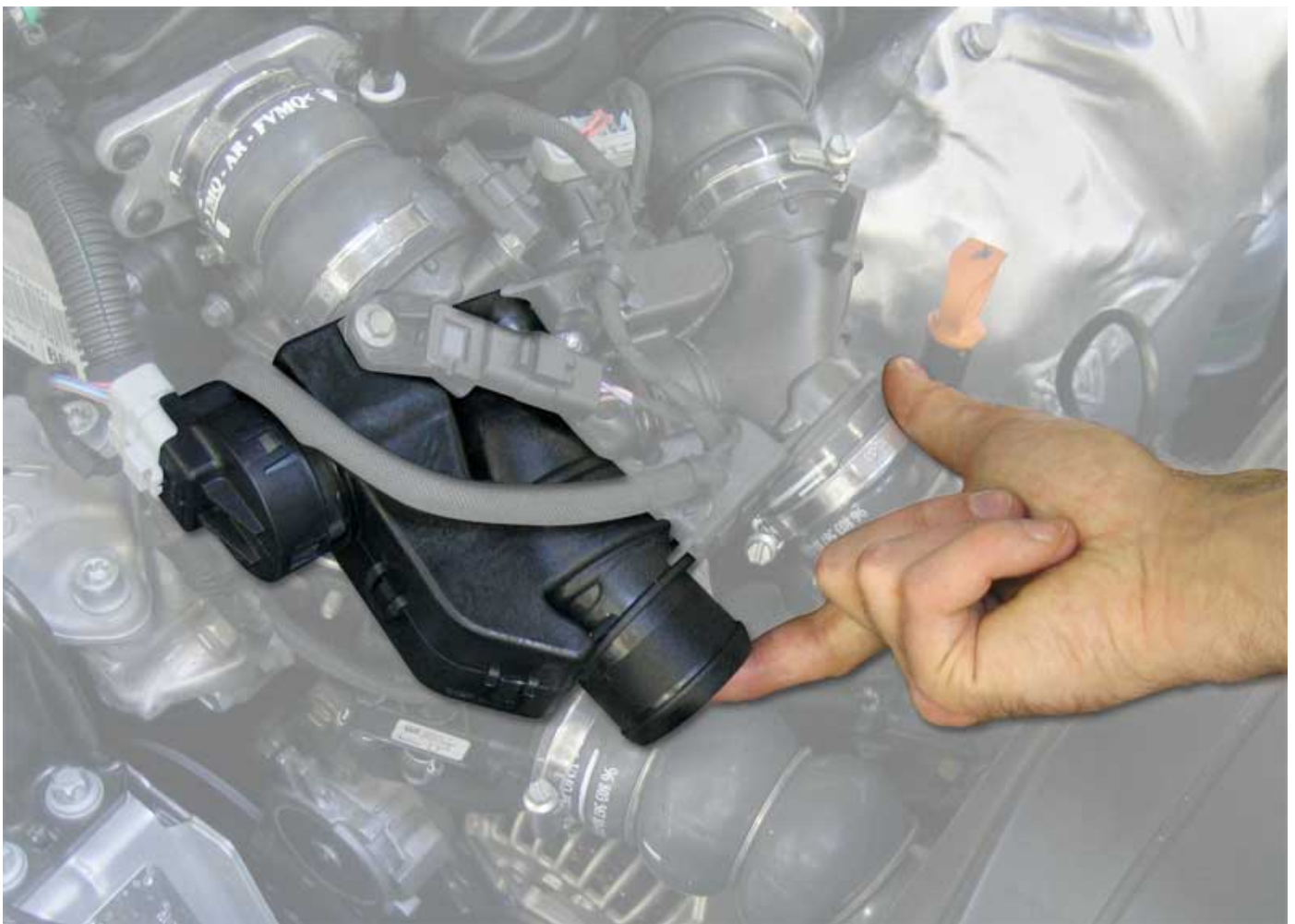
Figure 16 : Manual operation of the EGR flap (EDC16 C34)
