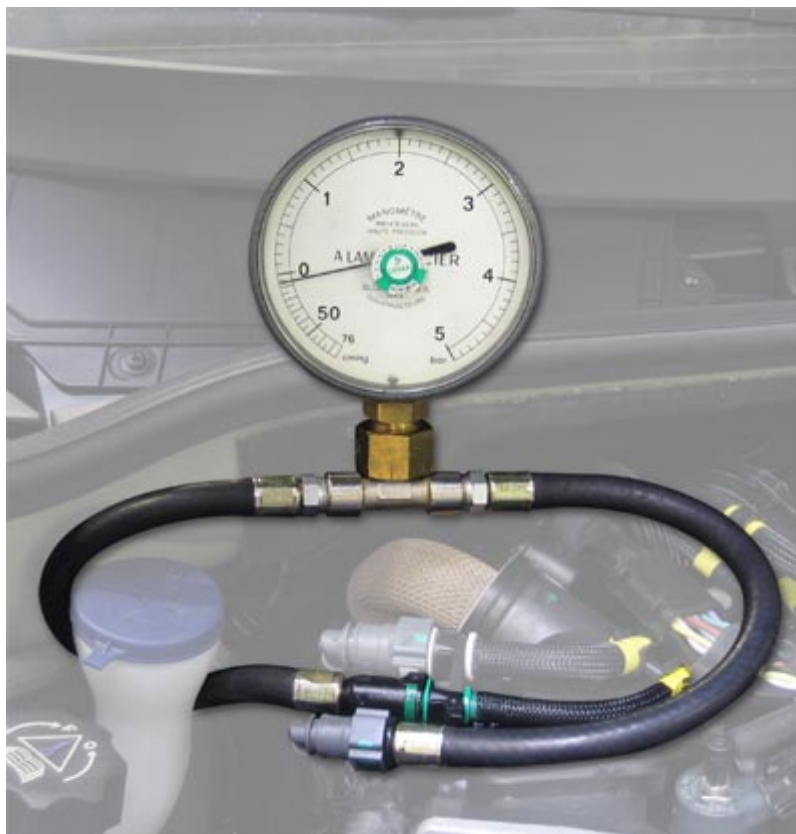
Figure 9: Fuel return pressure check (EDC16 C34)
