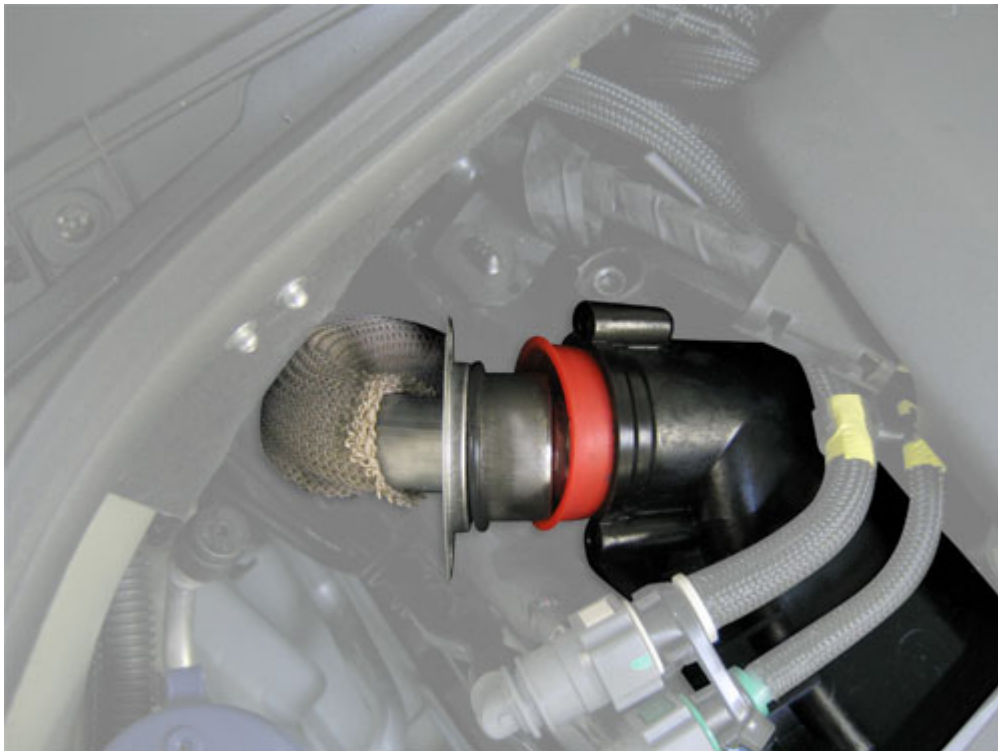
Figure 12: Plugging the EGR tube (EDC16 C34)
