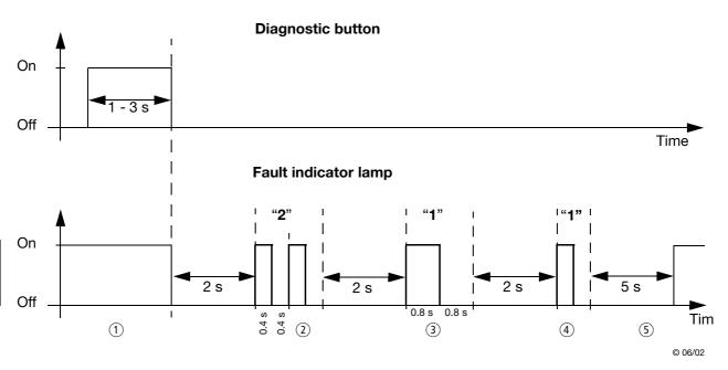
In the following the steps for reading out the first blink code are shown:
