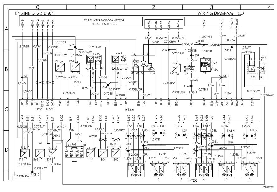
NOTE: D12D Interface connection is Interface Connection Box A14A (see also "Preheat Schematic, CB" page 13).
