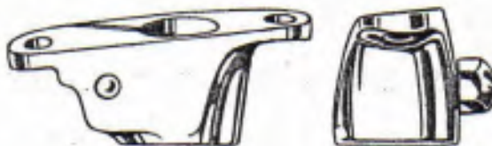
B-18573-A SPORTLIGHT BRACKET AFTER GRINDING FOR B68 CABRIOLET
