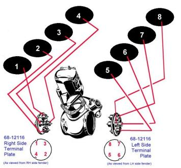
This view is from the front of the engine, but "left" and "right" are always from the perspective of the driver's seat (regardless of whether RH or LH drive vehicle). Firing order: 1-5-4-8-6-3-7-2
