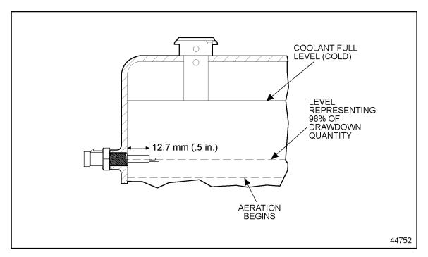
Figure 2-32 Engine Coolant Level Sensor Location - Top of Radiator Tank
