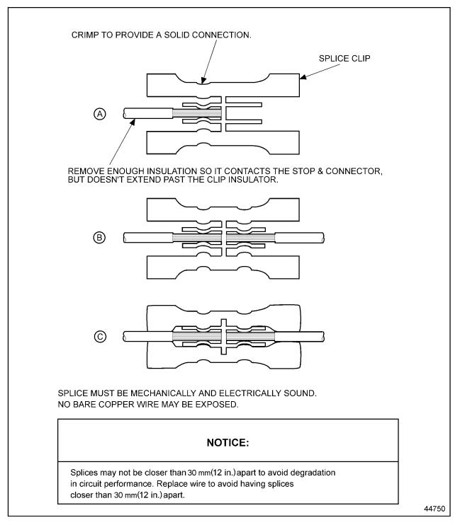
Figure 2-25 Splicing Straight Leads - Alternate Method 1
