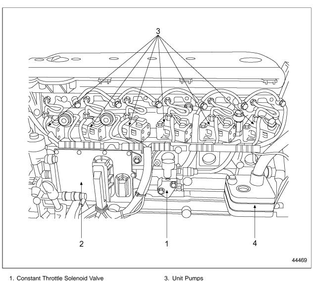
The engine brake function is activated by the constant throttle solenoid valve mounted on the side of the block. See Figure 21-1.
