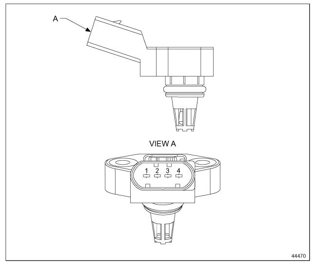
Figure 10-1Turbo Boost Air Combination Sensor
