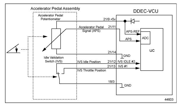
Figure 26-2 Typical Accelerator Pedal Installation
