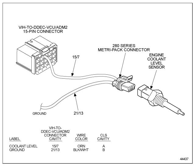
The OEM must connect the ECL Sensor probe as shown in the next illustration (see Figure 2-31). Polarity of the ground and signal must be correct for proper operation.
