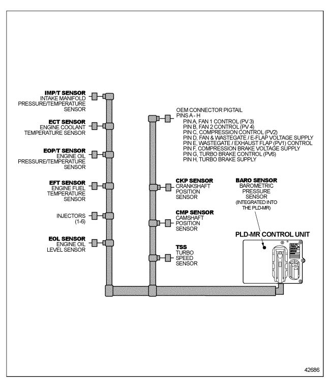
Figure 2-5 Typical MBE 4000 Engine Harness — Non-EGR Engine
