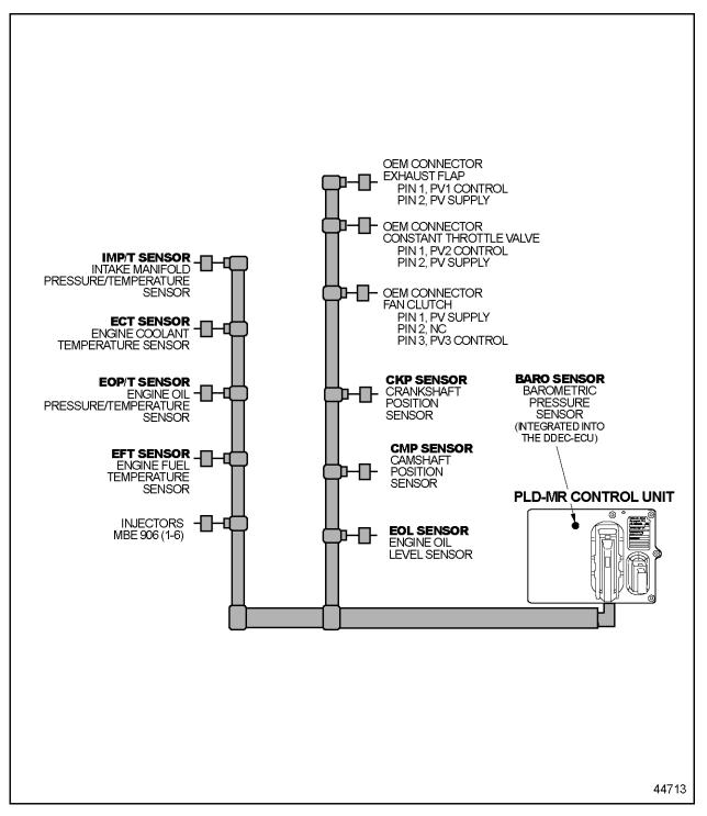
Figure 24-2 Typical MBE 900 Engine Harness
