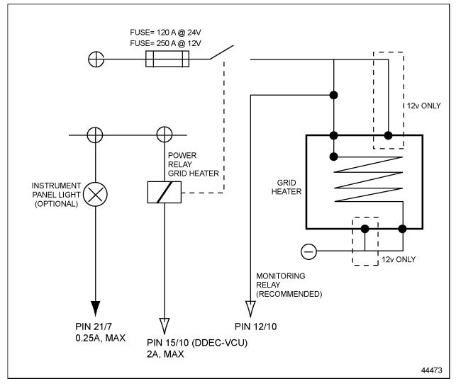
Figure 4-2 DDEC-VCU Grid Heater Wiring
