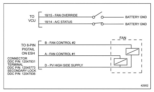
Figure 2-39 Two-Speed Fan on an MBE 4000 Engine
