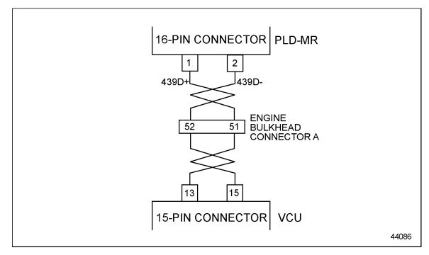
Figure 31-4 PLD-MR Engine Bulkhead Schematic — Acterra
