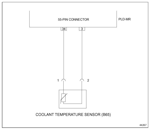
Figure 11-4 Engine Coolant Temperature Sensor Wiring
