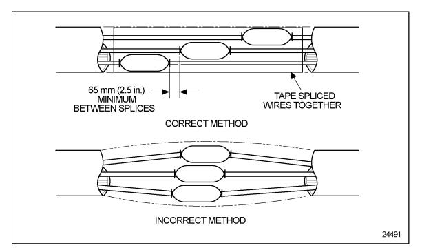
Figure 2-27 The Correct and Incorrect Method of Staggering Multiple Splices
