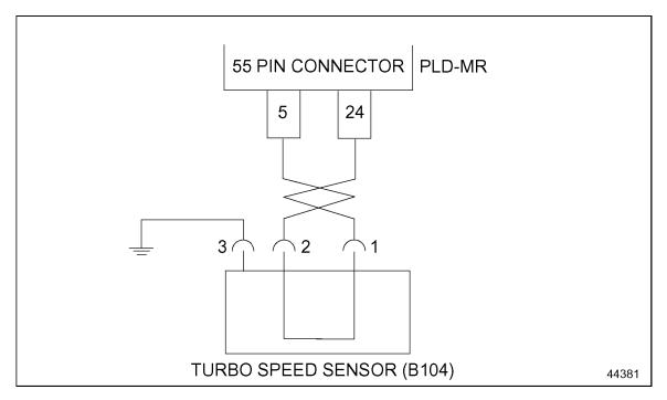
Figure 9-2 Turbo Speed Sensor Terminal and Wire Locations
