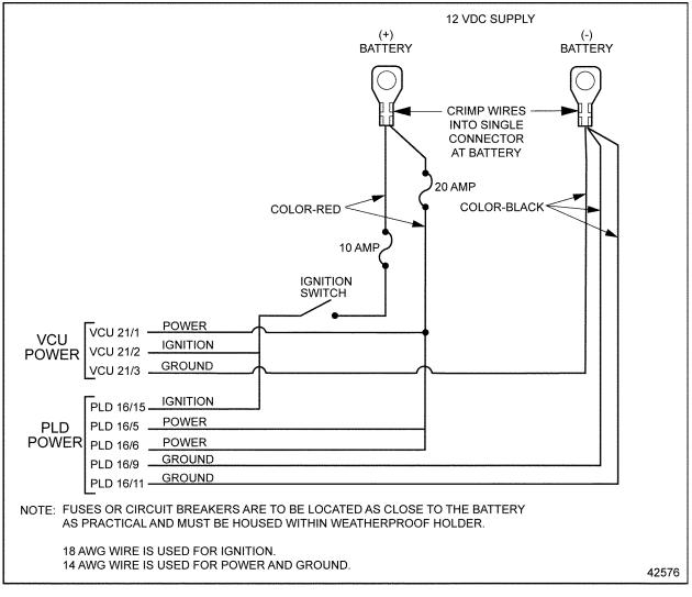
Figure 14-2 Power Wiring
