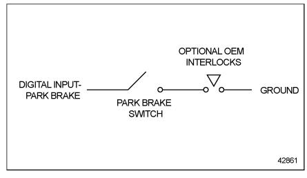
Figure 2-42 Parking Brake Digital Input
