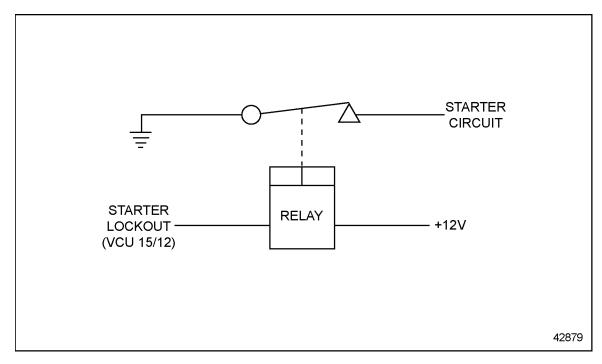
Figure 2-44 Starter Lockout
