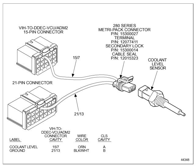
Figure 12-2 Engine Coolant Level Sensor Installation
