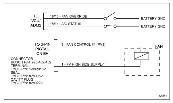
Figure 2-37 Single-Speed Fan on an MBE 900 Engine
