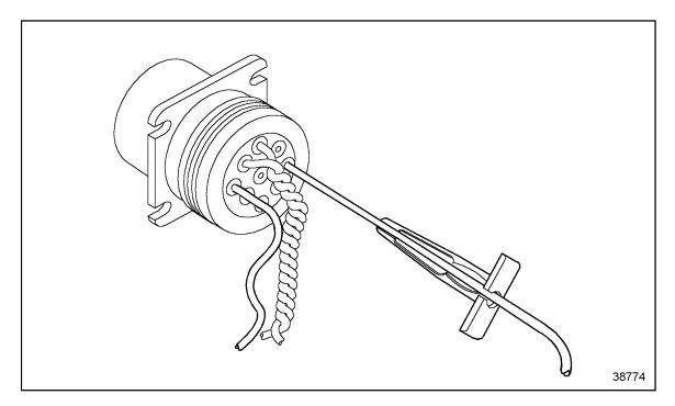
Figure 2-20 Removal Tool Position
