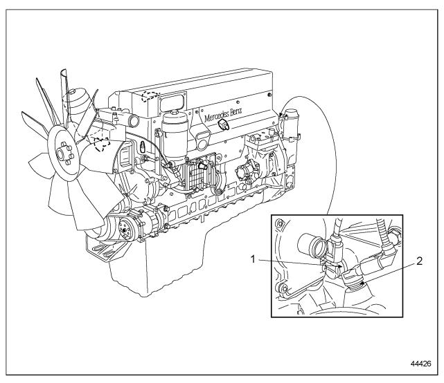
1. Camshaft Position Sensor (magnetic pickup)
