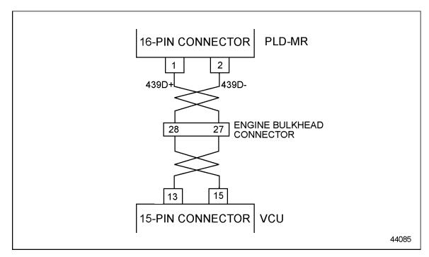
Figure 31-3 PLD-MR Engine Bulkhead Schematic — Business Class
