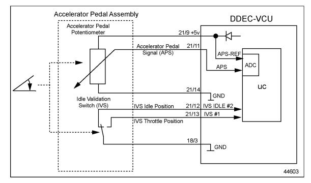
Figure 2-45 Accelerator Pedal Installation
