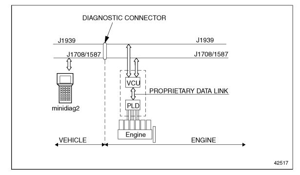
The DDEC-VCU also communicates over the J1587 and J1939 Data Links to the vehicle (see Figure 2-8).
