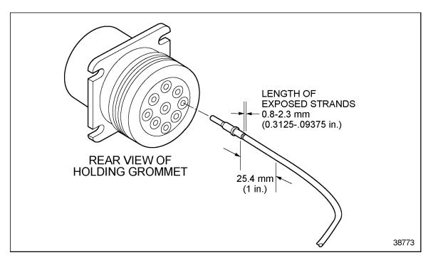
Figure 2-18 Pushing Contact into Grommet
