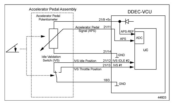
Figure 6-1 Accelerator Pedal Installation
