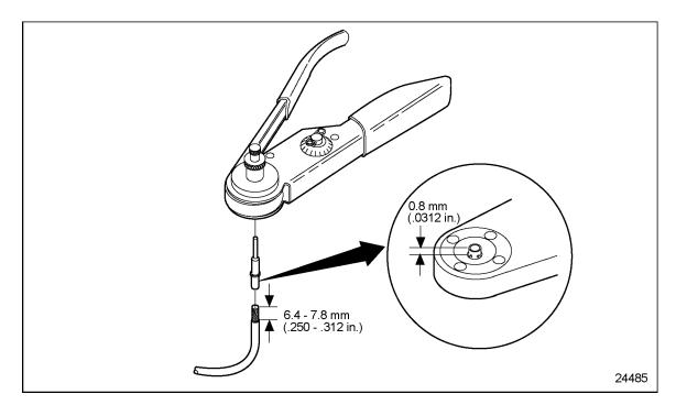
Figure 2-17 Setting Wire Gage Selector and Positioning the Contact
