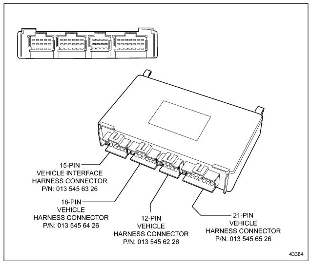
Figure 4-1 The DDEC-VCU
