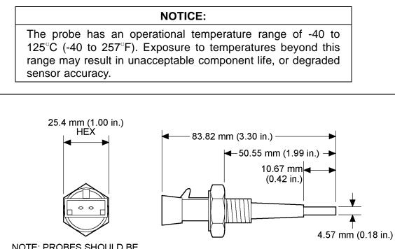
NOTE: PROBES SHOULD BE<br/>TORQUED<br/>ACCORDING TO THE FOLLOWING:4.57 mm (0.18 in.)PIPE THREAD<br/>1/4 in. NPT<br/>3/8 in. NPTTORQUE<br/>20.3 N·m (15 ft·lb)<br/>24.4-27.1 N·m (18-20 ft·lb)COOLANT LEVEL SENSOR<br/>3/8 in. NPT DDC P/N: 23520380<br/>9/16 in. UNF DDC P/N: 2352285538310
