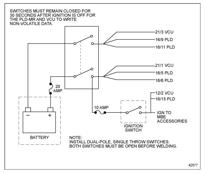
Figure 2-14 Main Power Supply Shutdown 12 or 24 Volt Systems
