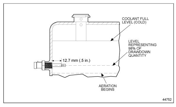
Figure 12-1 Engine Coolant Level Sensor Mounted in Radiator Top Tank
