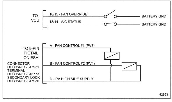
Figure 2-38 Dual Fan on an MBE 4000 Engine
