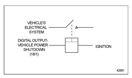
Figure 2-43 Vehicle Power Shutdown Relay
