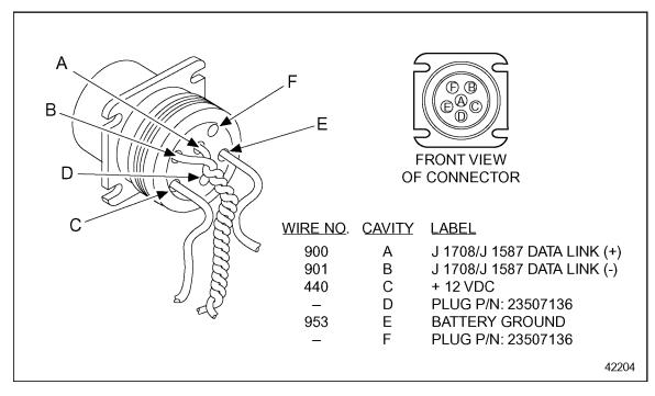
Figure 2-16 Wiring for 6-Pin Data Link Connector
