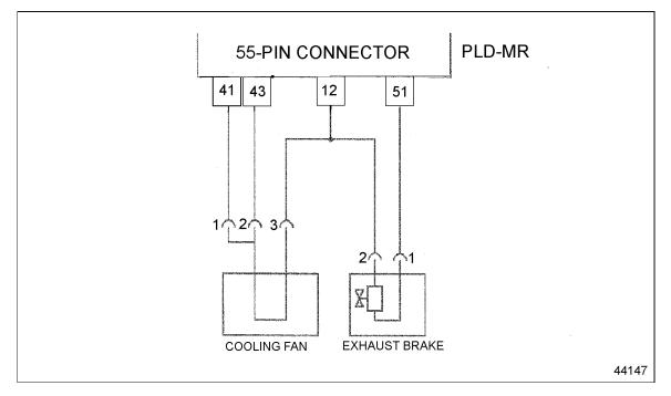
Figure 20-3 Exhaust brake and Cooling Fan Wiring
