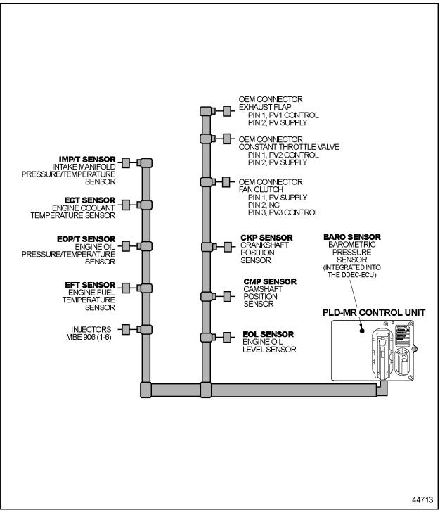
Figure 19-2 Typical On-Highway Six-Cylinder Engine Harness
