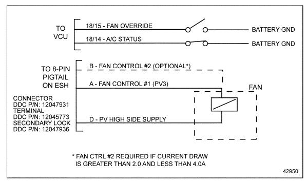
Figure 2-36 Single-Speed Fan on an MBE 4000 Engine
