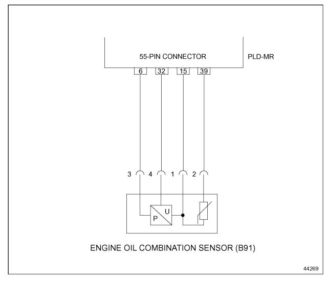
Figure 16-3 Engine Oil Combination Sensor Wiring Harness Connections
