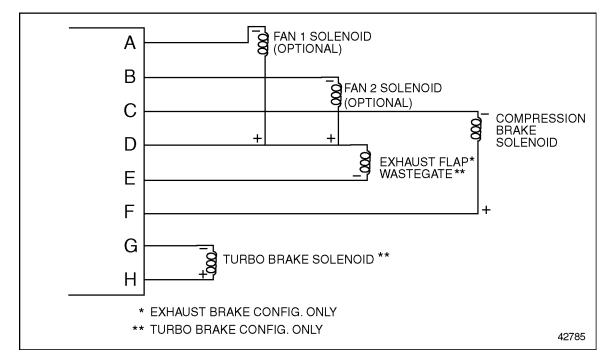
Figure 2-10 MBE 4000 Non-EGR Engine Brake
