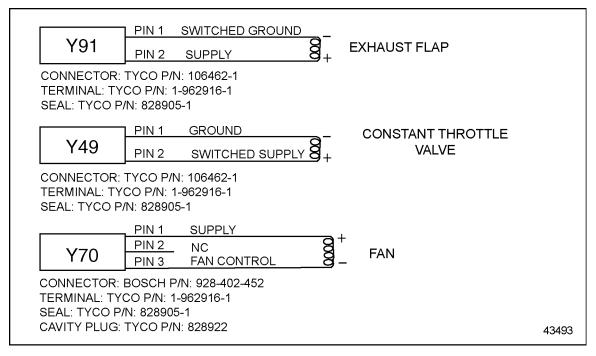
Figure 2-12 Engine Harness Connector for MBE 900 EGR Engine
