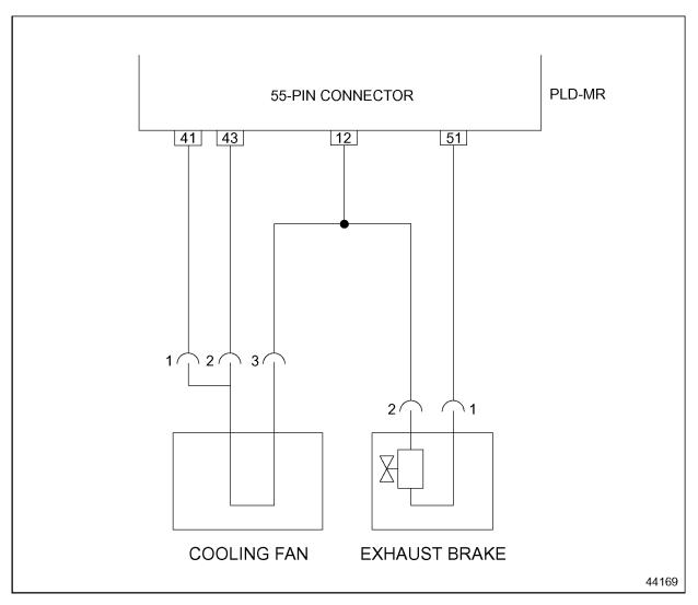
Figure 23-4 Location of Fan Control Wires
