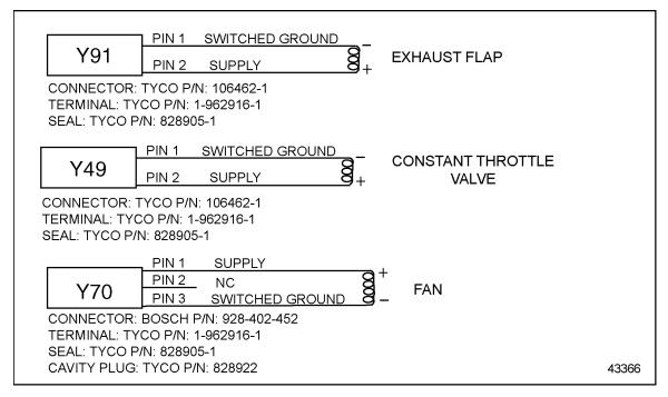
Figure 2-11 MBE 900 Non-EGR VIH to Engine Harness Wiring
