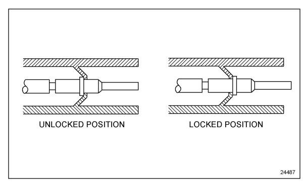
Figure 2-19 Locking Terminal into Connector
