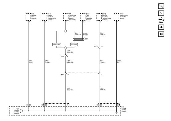
Fig. 3: Low Reference Bus (2 Of 2) Wiring Schematic Courtesy of GENERAL MOTORS COMPANY
