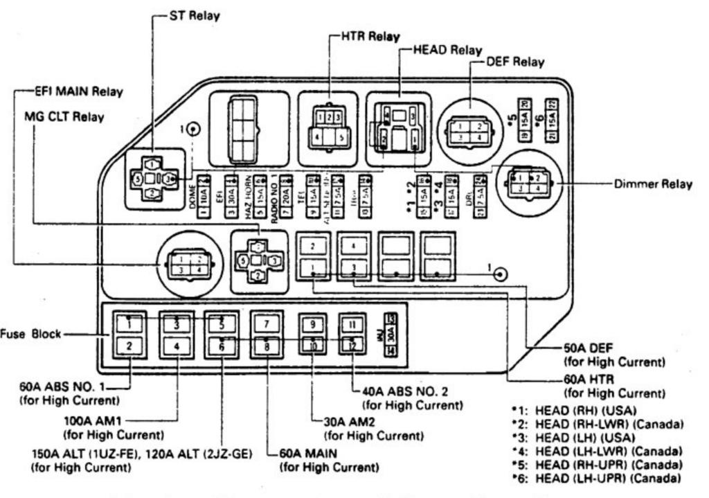
**Engine Compartment Fuse Panel**
