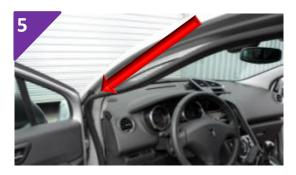
Run the cable replacing the seal on the driver's side door.
