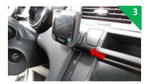
Stick the bracket supplied to the left of the WARNING button after having cleaned the surface. Then re-fit the screen and the air vents. (BE CAREFUL not to cut the cable)
