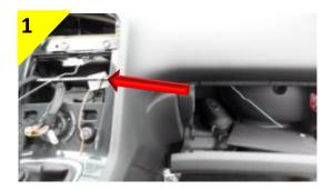
Pass a guide from the glove box towards the radio housing.
