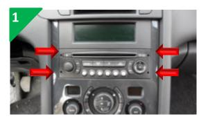
Insert the removal tools into the slots on each side of the radio.
