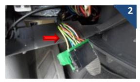
Using a jumper or a pigtail connection connect a wire to the YELLOW wire on the top left.
