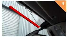
Using the plastic trim tools, run the cable under the headliner and into the windscreen post on the driver's side.
