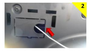
Pass the cable through the hole at the bottom inside the glove box.
