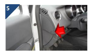
Using the plastic trim tools, unclip the clip located on the left of the dashboard.
