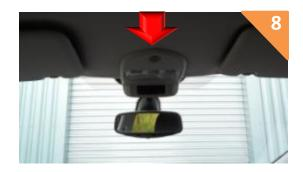
Using the plastic trim tools, release the cabin light without disconnecting it.
