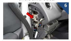
Pass the cable into the dashboard on the left side.
