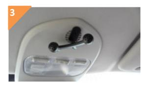
Stick the bracket (supplied) to the windscreen after thoroughly cleaning the surface.
