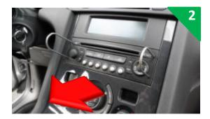
Unclip, pull and lift the radio making sure you properly disconnect the connector and the antenna.
