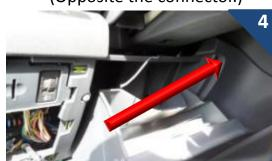
Pass the wire from underneath the steering wheel towards the radio housing.
