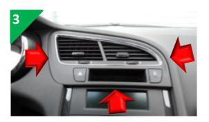
Using the plastic trim tools, unclip the display and the air vent.
