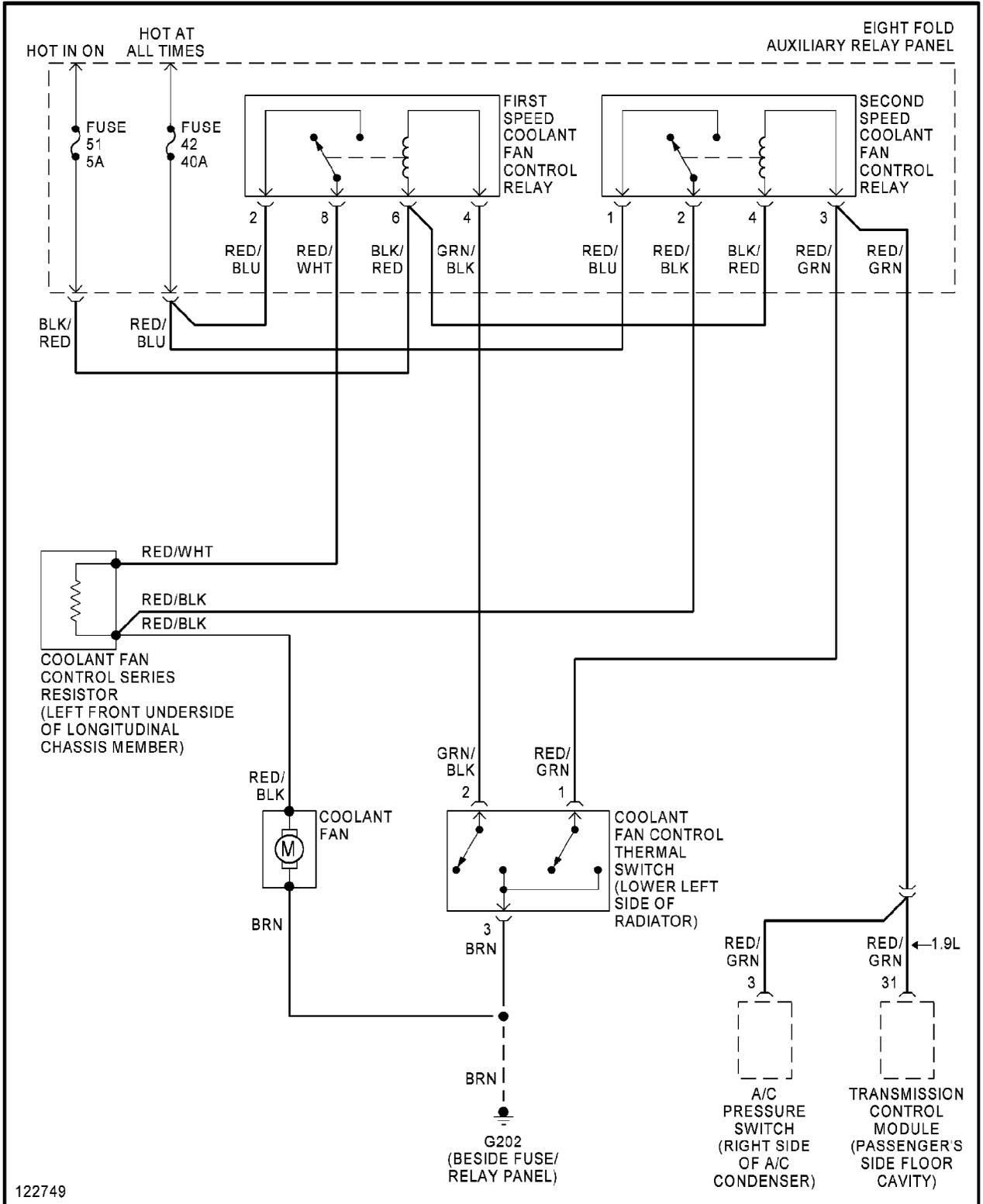
Dual Speed Cooling Fan Circuit, Manual A/C
