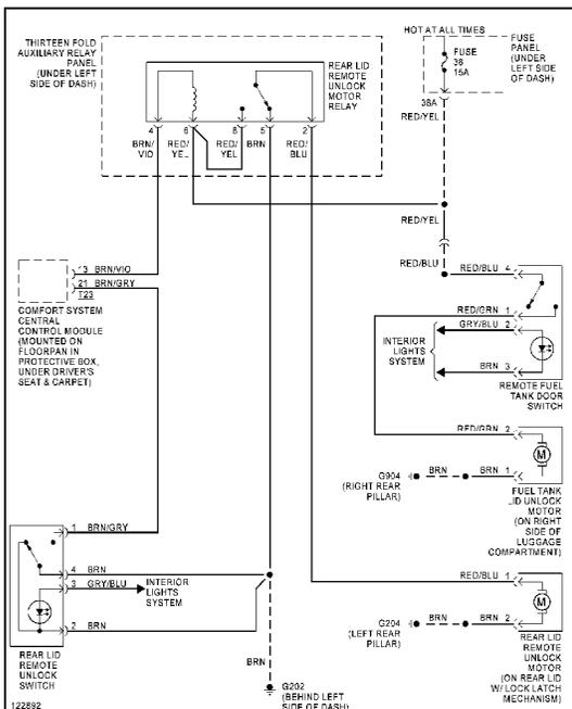
Trunk & Fuel Door Release Circuit
