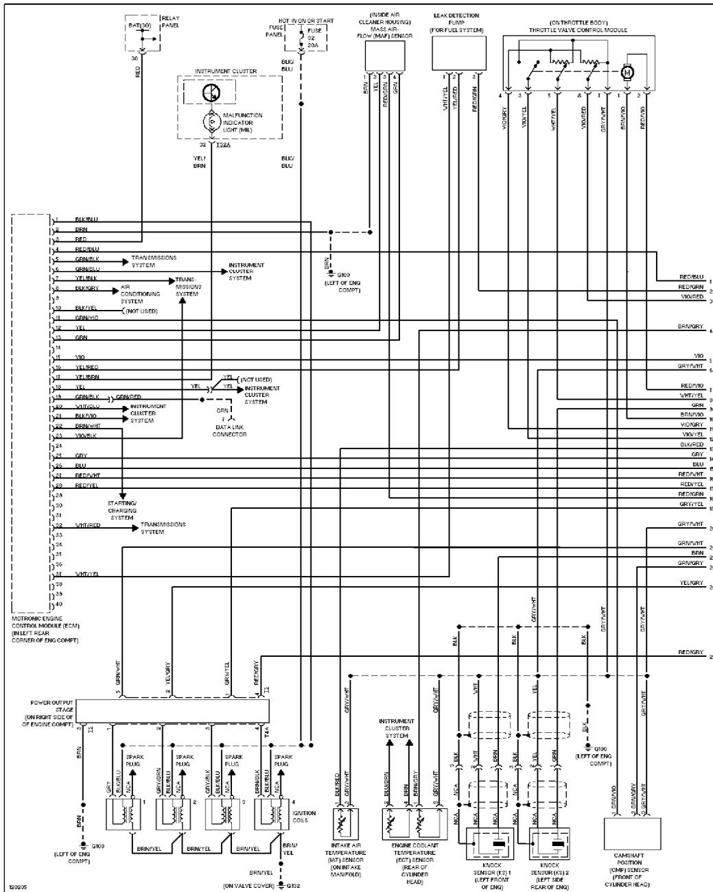
1.8L Turbo, Engine Performance Circuits (1 of 2)
