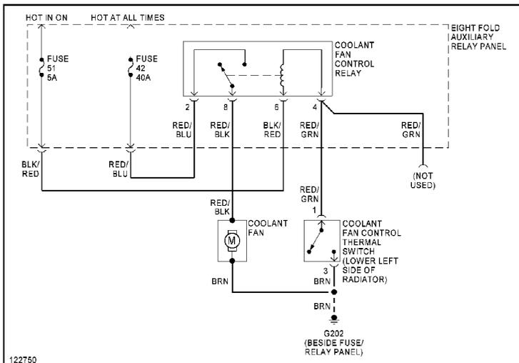
Single Speed Cooling Fan Circuit, Manual A/C
