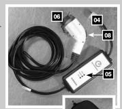
If the EVSE connector fits loosely to your power outlet, attach string to the connector and hang it on a hook near the outlet.
