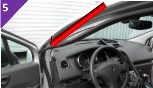
5 Run the cable replacing the seal on the driver's side door.
