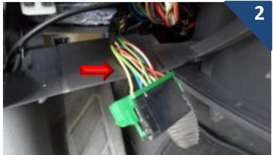
Using a jumper or a pigtail connection connect a wire to the YELLOW wire on the top left. (Opposite the connector.)
