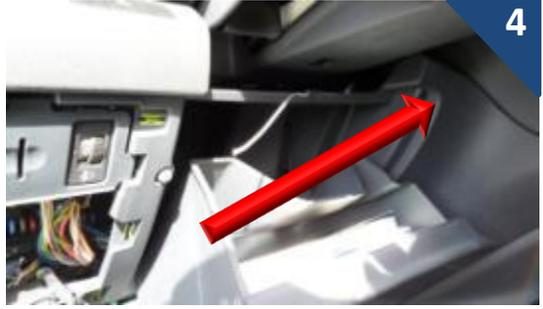
Pass the wire from underneath the steering wheel towards the radio housing.
