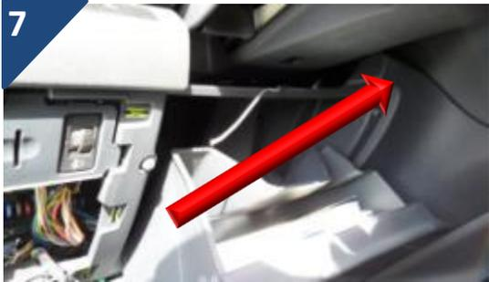
Run the cable under the dashboard into the glove box housing and towards the radio, attaching it with wire ties.
