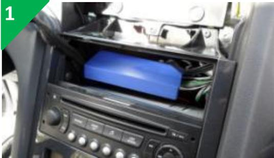
Connect the adaptor to the original connector. Connect all of the wires to the blue box as shown in the diagram below. Test before refitting, then slide the assembly behind the screen after refitting the radio.
