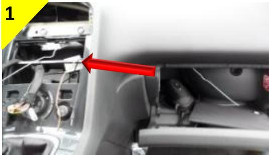
1 Pass a guide from the glove box towards the radio housing.
