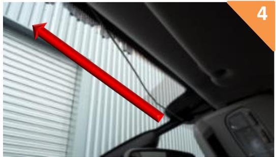
4 Using the plastic trim tools, run the cable under the headliner and into the windscreen post on the driver's side.
