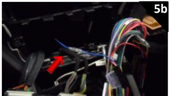
For adaptor 84744/9706AT (MKi range): disconnect the blue wire in front of the fuse, then connect the ACC wire.
