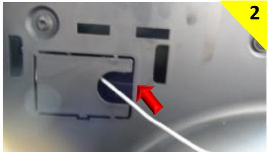
2 Pass the cable through the hole at the bottom inside the glove box.
