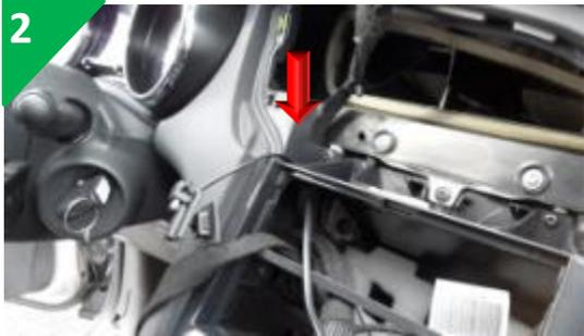
Run the bracket cable between the screen and the air vents.
