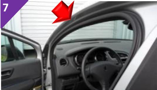
Remove the door seal on the driver's side.
