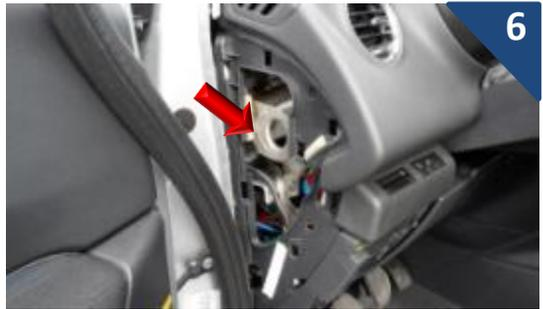
6 Pass the cable into the dashboard on the left side.
