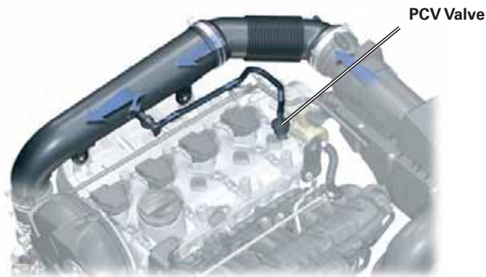
Cutaway View of Crankcase Breather Valve
