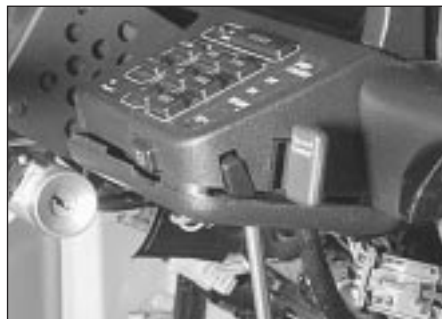
10.1 Remove the lower trim cover(s) from the instrument panel switch assembly
