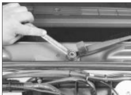
15.1 Lift up the wiper arm nut cover, remove the nut and pull the wiper arm straight off the shaft
