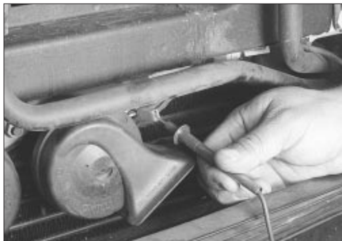
20.3 Check for power at the horn terminal with the horn button depressed
