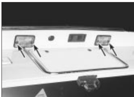
21.6 Detach the lens retaining screws (arrowed) and the lens to access the number plate light bulbs
