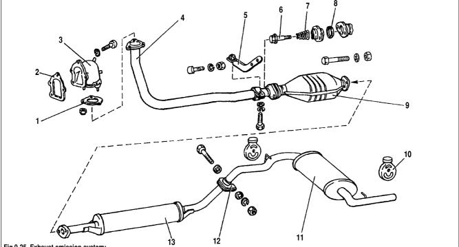
Fig.9-25. Exhaust emission system:
