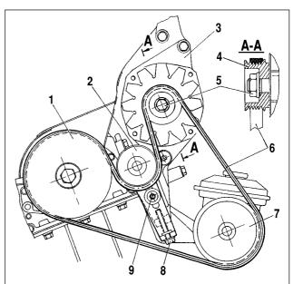
Fig.9-23. Removing and refitting the alternator drive belt:
