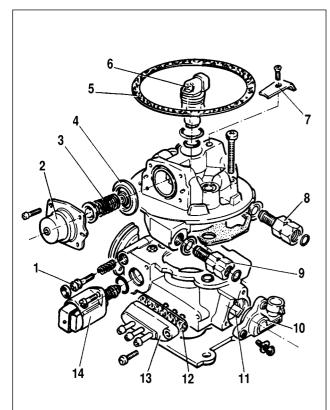
Fig.9-4. Components and assemblies of central injection unit:
