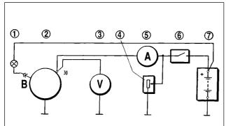
Fig.7-6. Alternator wiring connections for oscilloscope test:
