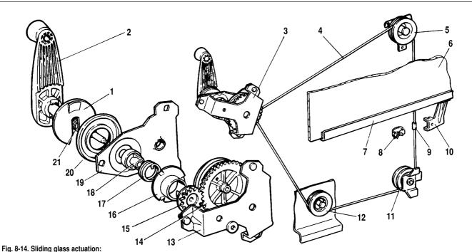
1 - escutcheon; 2 - window lifter handle; 3 - window lifter mechanism; 4 - cable; 5 - top roller; 6 - sliding glass; 7 - sliding glass holder; 8 - cable retainer; 9 - cable sleeve; 10 - glass holder bracket; 11 - bottom roller; 12 - tensioner; 13 - window lifter housing; 14 - barrel and driven gear; 15 - pinion; 16 - support; 17 - brake spring; 18 - spring brake drive link; 19 - housing cover; 20 - surround; 21 - shaft
