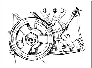
Fig.7-18. Ignition timing marks:
