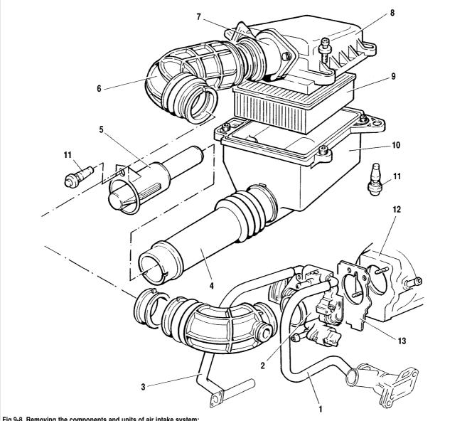
Fig.9-8. Removing the components and units of air intake system:
