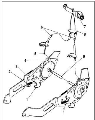
Fig.8-32. Front seat back reclining and tipping mechanisms:
