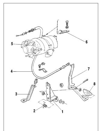
Fig.9-7. Removing the accelerator linkage:
