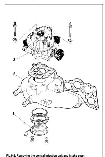
1 - intake manifold preheater; 2 - intake manifold; 3 - central injection unit
