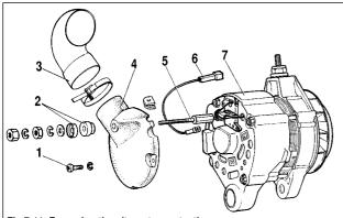
Fig.7-11. Removing the alternator protective case:
