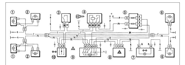
Fig.7-30. Wiring diagram for direction indicators and hazard flashers :
