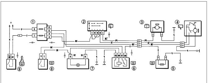
Fig.9-33. Wiring diagram for tailgate wipe/wash and heating element:
