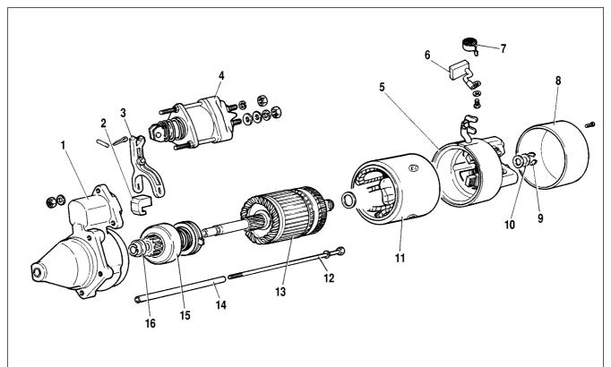
Fig.7-16. Exploded view of starter motor:
