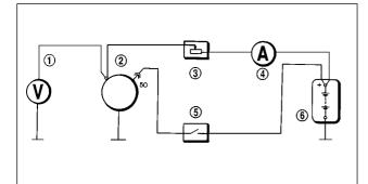
Fig.7-15. Wiring connections for starter motor testing:
