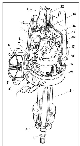
Fig.7-19. Ignition distributor (3810.3706 model):
