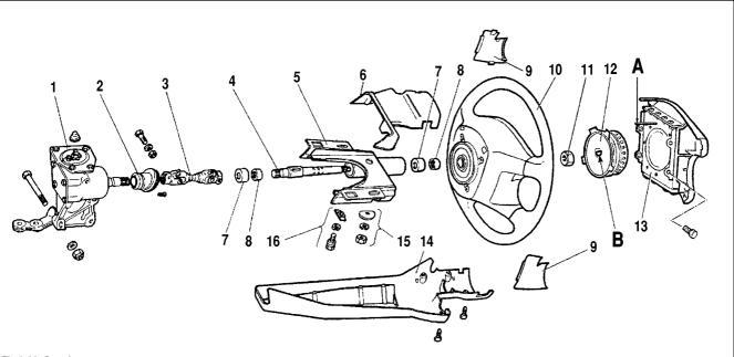
Fig.9-38. Steering components:
