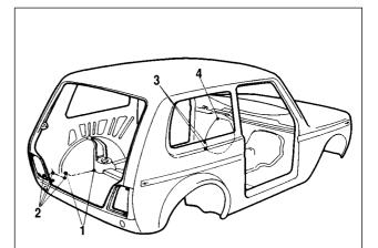
Fig.8-11. Locations for 51-F7-type sealant application (rear body view):
