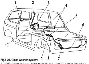
1 - tailgate washer jet; 2 - pump-to-jet hose; 3 - tailgate washer reservoir; 4 - windscreen washer jets; 5 - headlight washer pump; 6 - hose to headlight jet; 7
