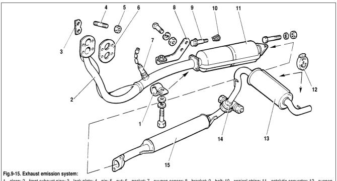
1 - clasp; 2 - front exhaust pipe; 3 - lock plate; 4 - pin; 5 - nut; 6 - gasket; 7 - oxygen sensor; 8 - bracket; 9 - bolt; 10 - conical string; 11 - catalytic converter; 12 - suspension loop; 13 - main silencer; 14 - clip; 15 - front silencer
