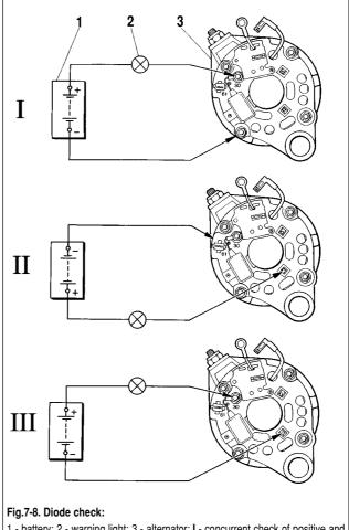
1 - battery; 2 - warning light; 3 - alternator; I - concurrent check of positive and negative diodes; II - check of negative diodes; III - check of positive diodes
