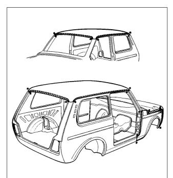
Fig.8-5. Weld contours, front wing and roof panel. Dots designate seams of resistance welding. Arrowed are places tacked by gas welding
