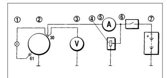
Fig.7-5. Wiring connections for diode plate test:
