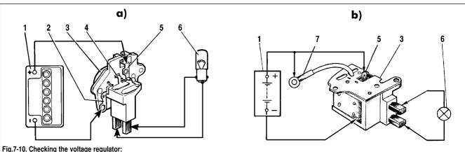
a - 1996-on voltage regulator; b - pre-1996 voltage regulator; 1 - battery; 2 - voltage regulator earth; 3 - voltage regulator; 4 - voltage regulator terminal «Ш»; 5 - voltage regulator terminal «B»; 6 - warning light; 7 - voltage regulator terminal «Б»
