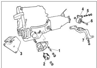
Fig.9-19. Engine support:
