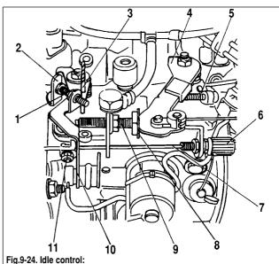
1 - throttle stop (CO adjustment) screw; 2 - stop lever; 3 - locating pin; 4 - load lever; 5 - limiter; 6 - outer cable tensioner; 7 - accelerator cable; 8 - gasket; 9 - limiter; 10 - fast idle lever; 11 - cable tensioner
