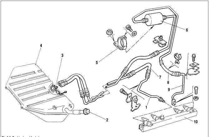
Fig.9-6. Fuel tank and fuel pipes:
