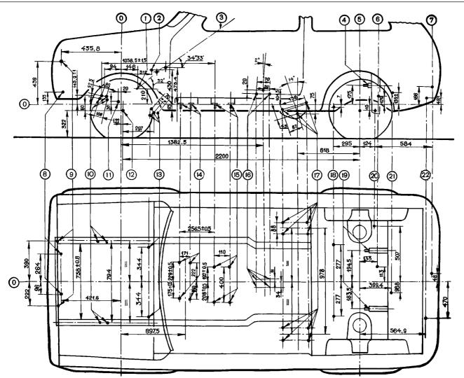
Fig.8-4. Anchorages of vehicle units and assemblies:
