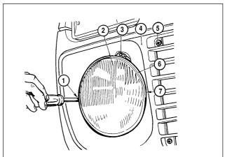
Fig.7-31. Headlight alignment:
