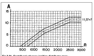
Fig.7-21. Centrifugal advance ignition distributor map:
