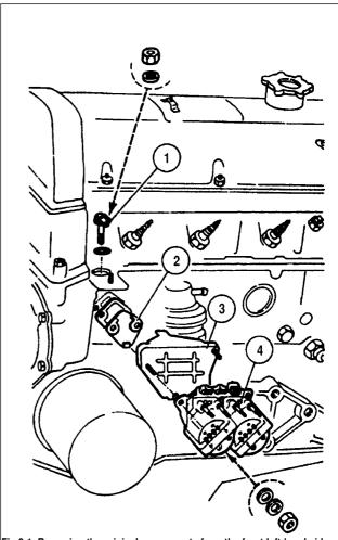
Fig.9-1. Removing the original components from the front left-hand side of the engine:
