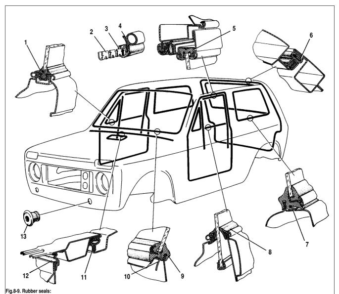
1 - of swivel glass; 2 - front door seal frame; 3 - seal molding; 4 - front door seal; 5 - of sliding glass; 6 - of tailgate aperture; 7 - of side window; 8 - lower seal of sliding window; 9 - of windscreen; 10 - drain pipe; 11 - bonnet seal; 12 - of air intake; 13 - of front bumper connection
