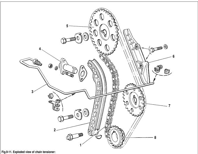
1 - chain; 2 - tensioner shoe; 3 - oil delivery pipe to tensioner; 4 - chain tensioner; 5 - camshaft sprocket; 6 - chain damper; 7 - oil pump shaft sprocket; 8 - crankshaft sprocket
