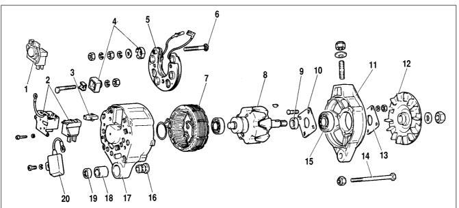
Fig.7-12. Alternator components:
