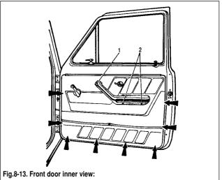
1 - top armrest screw clip; 2 - bottom armrest securing screws Arrowed is the location for door trim securing clips
