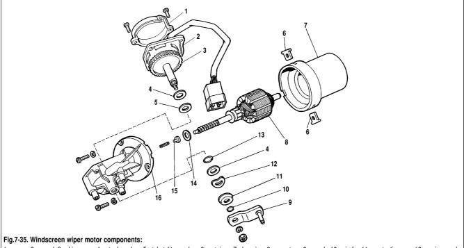
1 - cover; 2 - panel; 3 - drive gear; 4 - steel washer; 5 - tekstolite washer; 6 - retainer; 7 - housing; 8 - armature; 9 - crank; 10 - circlip; 11 - protective cap; 12 - spring washer; 13 - sealing ring; 14 - shim; 15 - thrust washer; 16 - motor cover
