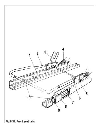
1 - slide; 2 - seat sliding mechanism handle; 3 - bottom seat back rake adjuster
