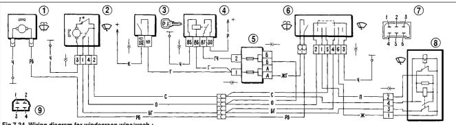
Fig.7-34. Wiring diagram for windscreen wipe/wash:
