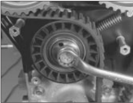
8.20 Slacken tensioner bolt to give initial belt tension
