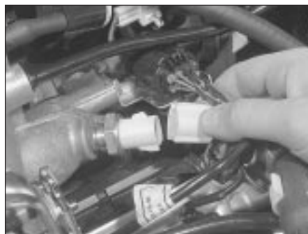
14.43 Disconnecting the intake air temperature sensor multi-plug
