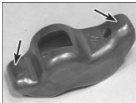
11.19 Inspect the rocker arm contact points indicated for excessive wear
