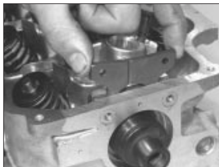
11.10b ... and lift out the camshaft thrust plate
