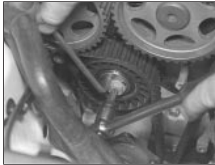
8.12 Slacken tensioner bolt, and use Allen key to rotate tensioner away from timing belt
