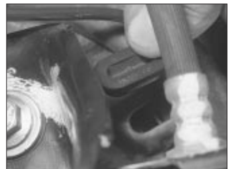
5.2 Removing the rubber access plug from the rear of the brake backplate
