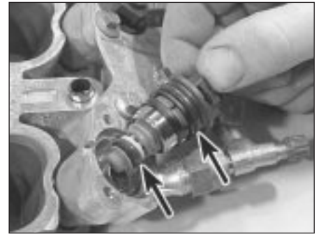
14.18 Removing an injector from the fuel rail. Note the O-ring seals (arrowed)
