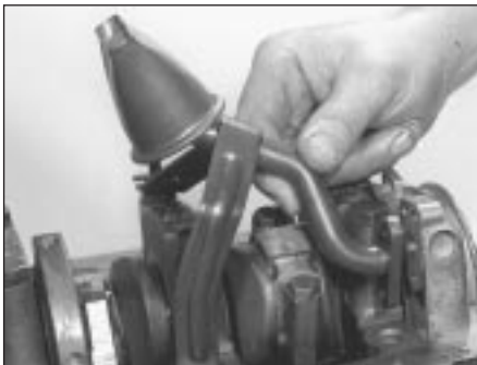
14.4 Removing the oil inlet pipe
