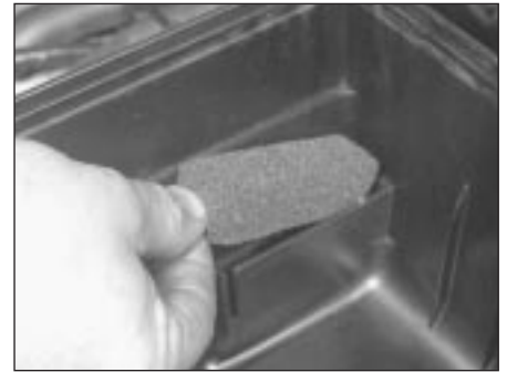
25.13 The crankcase ventilation system foam filter is located in the air cleaner housing on Zetec engines
