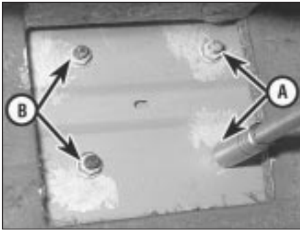
11.6 Servo mounting bracket retaining nuts
