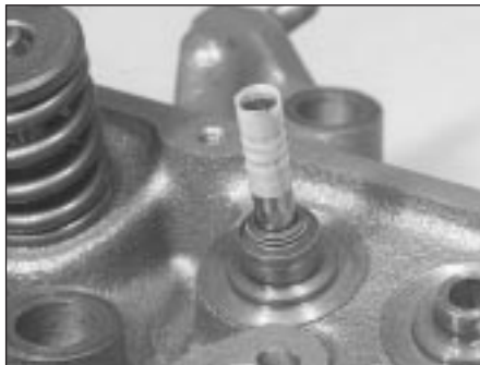
9.3a Tape the end of the valve stem before fitting the valve stem seal
