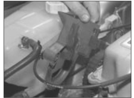
7.5 Lower timing belt cover removal
