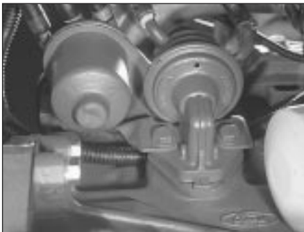
7.6 Fuel pump and fuel vapour separator arrangement on HCS engine (shown from below)
