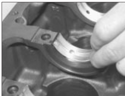
17.6 Fit the bearing shells to the main bearing housings in the crankcase
