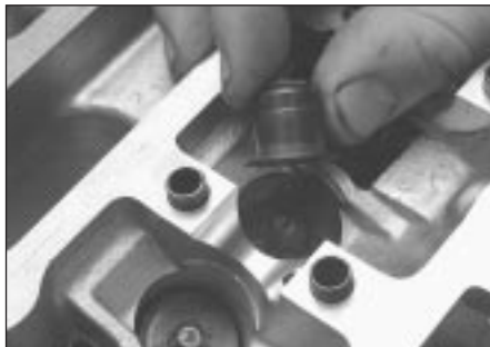
9.16 Valve spring pressure is sufficient to seat lower seat/stem oil seals on reassembly
