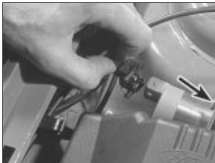
14.24 Disconnect the multi-plug from the idle speed control valve. Upper valve retaining bolt (arrowed)
