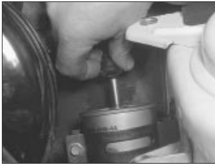
30.5 Releasing the fuel pipe unions from the filter on models with quick-release couplings
