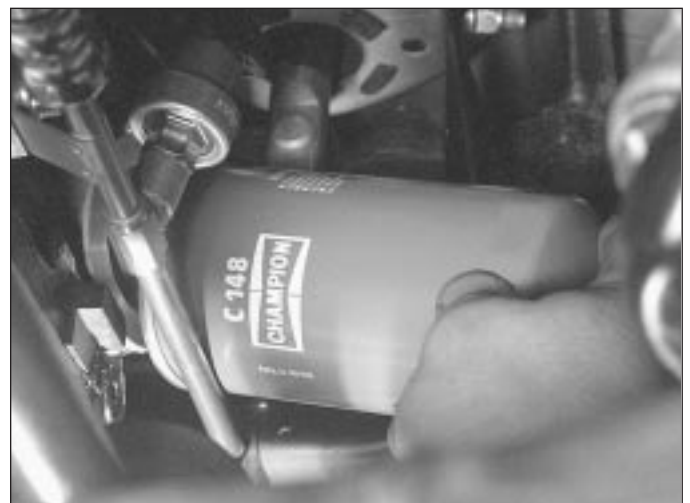
3.10b Fitting the new oil filter on the Zetec engine
