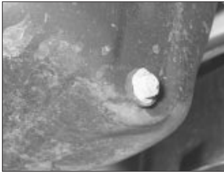
3.7a Engine oil drain plug location in the sump on HCS, CVH and PTE engines
