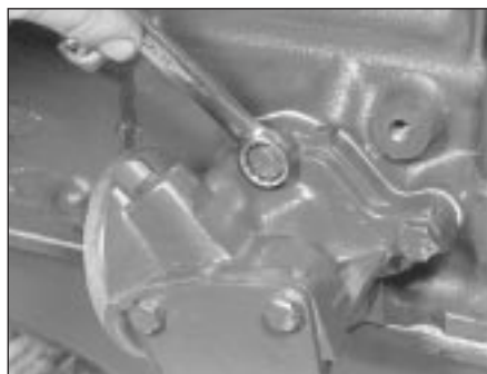
12.4 Unscrewing the oil pump retaining bolts
