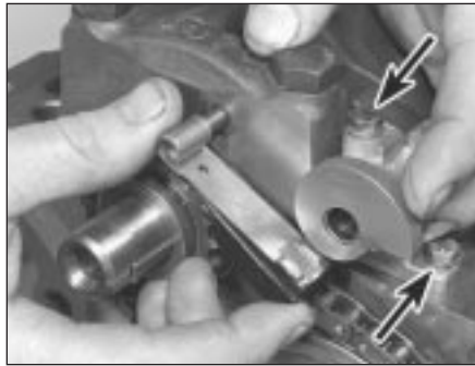
10.3 Chain tensioner arm removal from the pivot pin. Note tensioner retaining bolts (arrowed)
