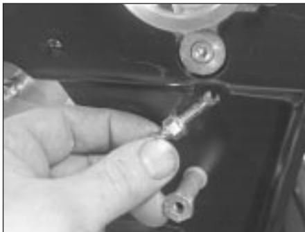
8.17a Fitting tensioner spring retaining pin
