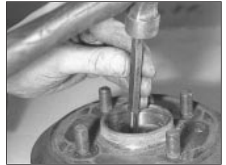
9.8 Removing bearing cups
