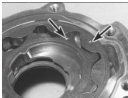
15.4 Inner and outer rotor matchmarks (arrowed)
