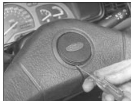
19.2 Removing the motif from the steering wheel
