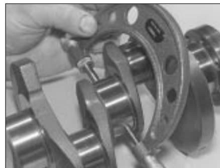
12.22 Measure the diameter of each crankshaft journal at several points, to detect taper and out-of-round conditions
