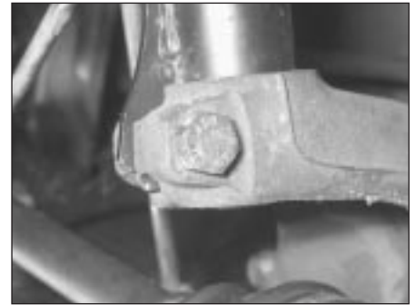
2.10 Remove the suspension strut-to-spindle carrier pinch bolt
