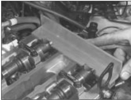
8.8 Fit camshaft-aligning tool to ensure engine is locked with Nos 1 and 4 cylinders at TDC
