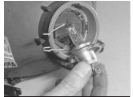
5.2b . . . then unlock the headlight bulb retaining spring and withdraw the bulb
