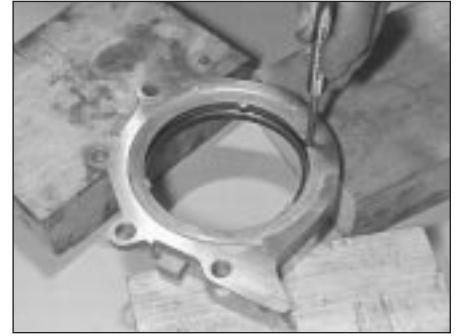
15.13 . . . and ensure that carrier is properly supported when driving out used oil seal - note notches provided in carrier for drift
