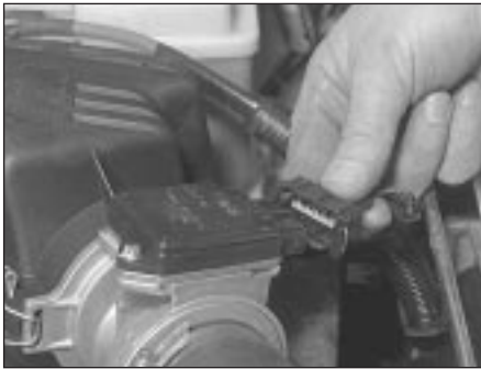
24.7 On SEFi fuel injection engines, disconnect the mass air flow sensor wiring multi-plug . . .
