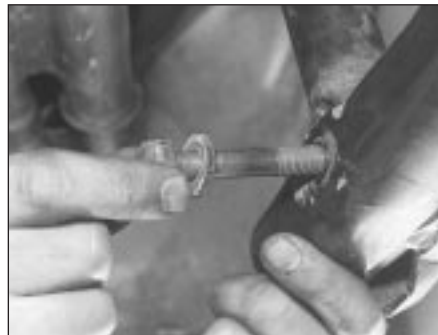
10.3 Lower suspension strut-to-axle mounting bolt
