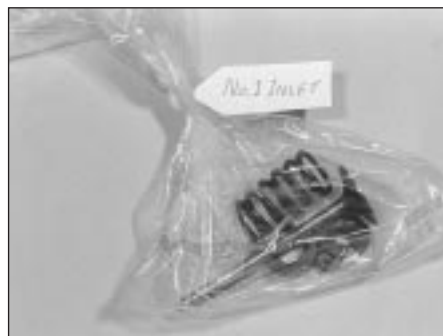
7.9 Use a labelled plastic bag to store and identify valve components
