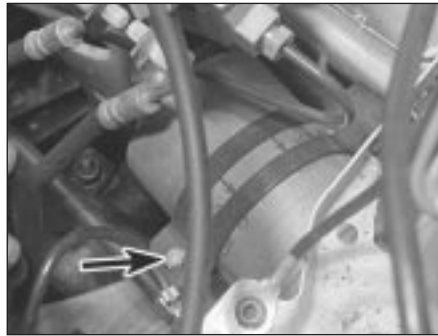
30.6a Fuel filter location below battery showing clamp bolt (arrowed). Note fuel flow direction arrows on filter body
