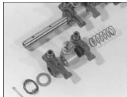
6.4 Rocker shaft partially dismantled for inspection
