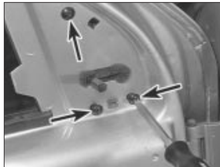
18.8 Removing the three mirror retaining screws (arrowed)
