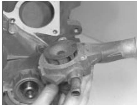
8.6 HCS engine water pump removal
