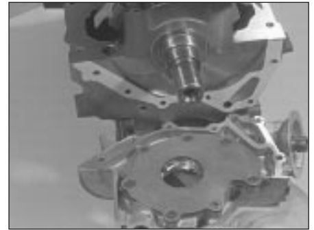
14.12 Use new gasket when refitting oil pump
