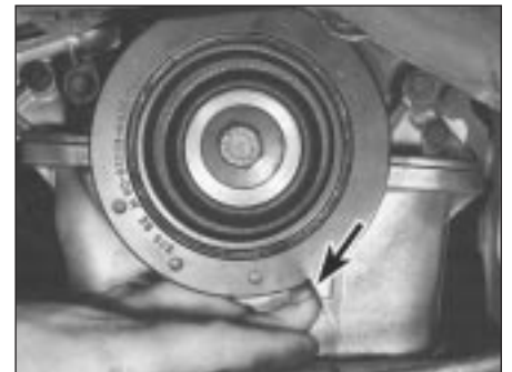
3.6b . . . use a straight edge extended out from the sump (arrowed) if greater accuracy is required
