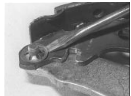
6.8 Lever off the spring clip securing the handbrake operating lever to the trailing shoe
