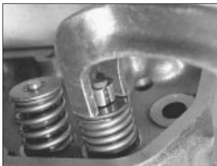
7.6 Compress the valve spring to remove the collets
