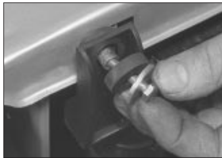
7.6a Radiator securing bolt, insulator and washer
