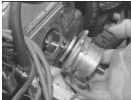
8.6 Removing the distributor from the cylinder head
