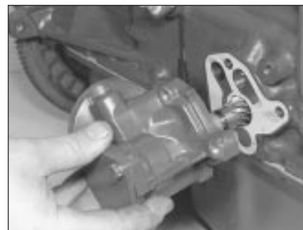
12.7 Refitting the oil pump. Note the new gasket
