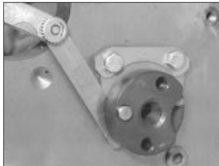
10.3 Checking the camshaft endfloat
