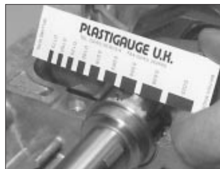
17.15 Compare the width of the crushed Plastigauge to the scale on the envelope to determine the main bearing running clearance
