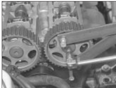
11.3 Using forked holding tool while camshaft toothed pulley bolt is slackened
