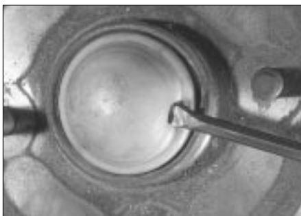
9.3 Removing the outer grease cap from the hub centre
