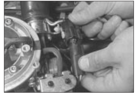
14.28b Disconnecting the throttle plate control motor multi-plug
