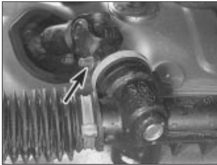
20.9 Pinch-bolt securing lower steering shaft universal joint to pinion splined shaft (arrowed)
