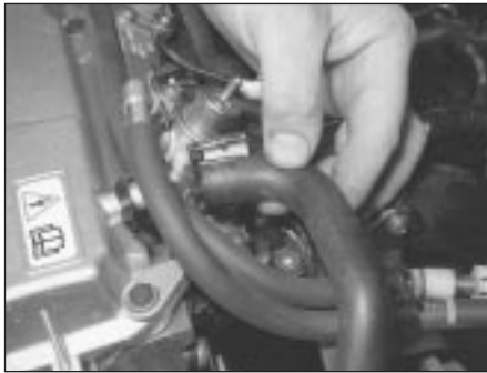
4.6 Disconnecting crankcase breather hose from cylinder head cover union
