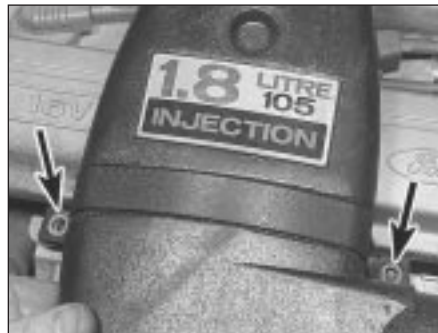
4.9 Unscrew the nuts (arrowed) to release the air intake duct on Zetec engines
