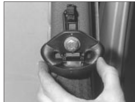
41.11 Removing a seat belt upper anchor cover
