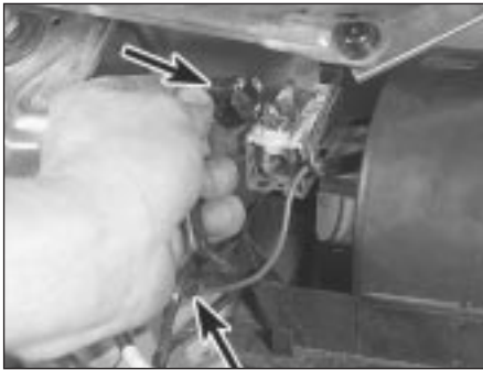
11.17 Disconnecting the wiring from the heater fan motor and resistor assembly (arrowed)
