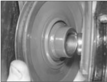
6.7 Crankshaft pulley removal
