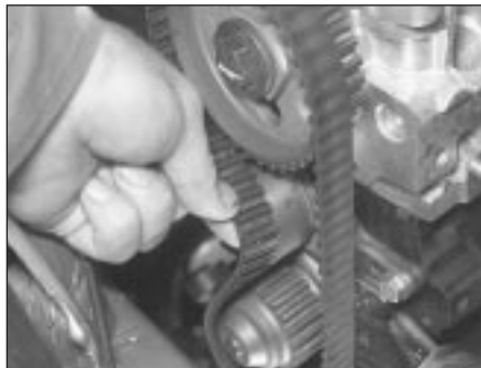
8.5 Timing belt removal
