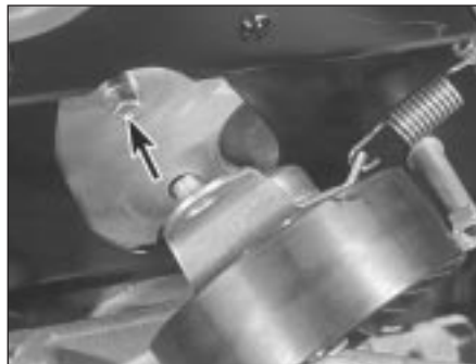
8.17b Hook spring onto tensioner and fit as shown - engage tensioner backplate on locating peg (arrowed) . . .
