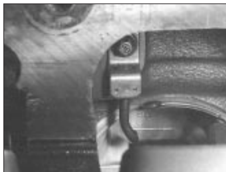
13.1b . . . but note that piston-cooling oil jets (where fitted) must be renewed whenever engine is overhauled - Zetec engines
