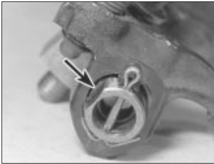
6.8 Flat on the rocker shaft (arrowed) to same side as rocker arm adjusting screws
