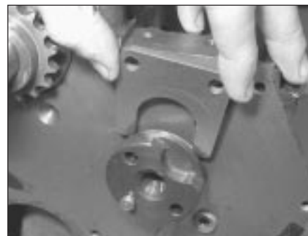
10.15 Refitting the camshaft thrust plate
