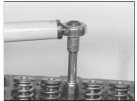
7.27b Tightening the cylinder head bolts (Stage 1)
