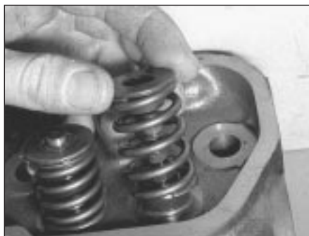
7.7a Remove the valve spring retainer and spring . . .
