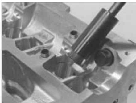
7.21a Ford service tool in use to remove valve spring lower seat/stem oil seals . . .
