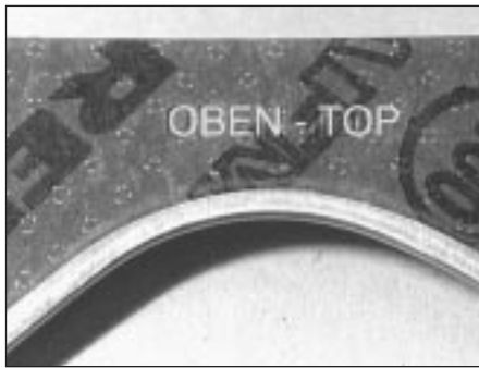
7.25 Cylinder head gasket top-face marking ("OBEN")
