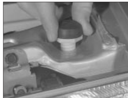
6.9 Altering the setting of a bonnet closure bump stop
