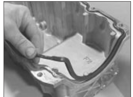
13.11 Ensure gasket is located correctly in sump groove
