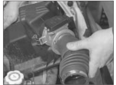
24.9 . . . then undo the retaining screws or release the clips and lift off the air cleaner lid complete with mass air flow sensor
