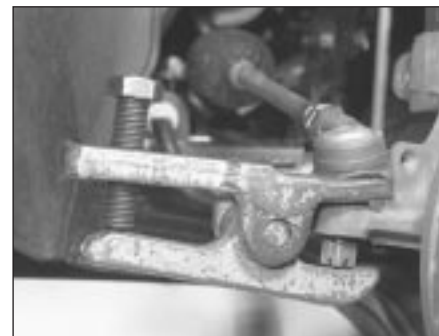
28.3 Balljoint separator tool in position. Note that the nut should be left loosely in position to protect the thread for re-use
