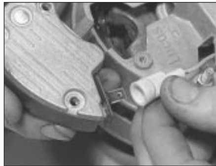
7.7b Disconnecting the field connector (Magneti-Marelli alternator)
