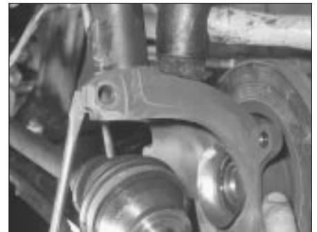
2.12 Separate the spindle carrier from the strut
