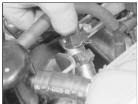
14.9a Disconnect the wiring multi-plug from each injector ...
