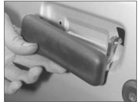
22.4b Removing the door exterior handle, guiding its operating rod out through the door skin (front door)
