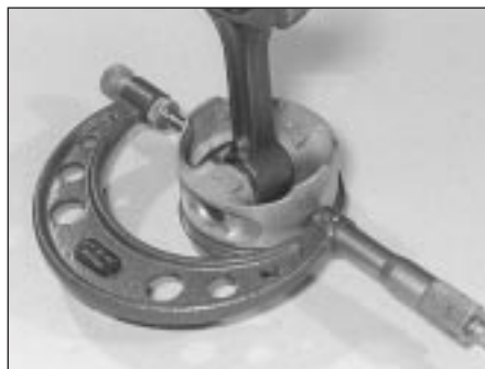
13.13 Measure the piston skirt diameter at right-angles to the gudgeon pin axis, just above the base of the skirt
