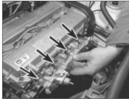
14.17b Note nose seals (arrowed) between rail and intermediate flange
