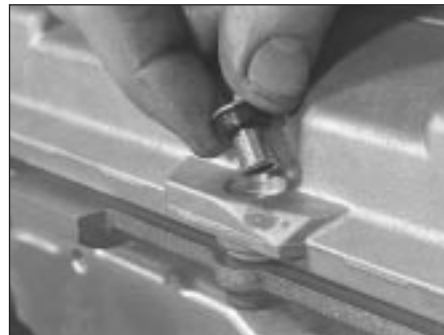
4.11 Ensure rubber seal is fitted to each cover bolt spacer, as shown
