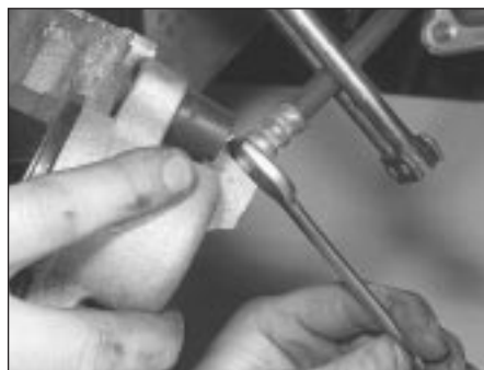
3.5 Hold the brake hose with a spanner and unscrew the caliper from the hose
