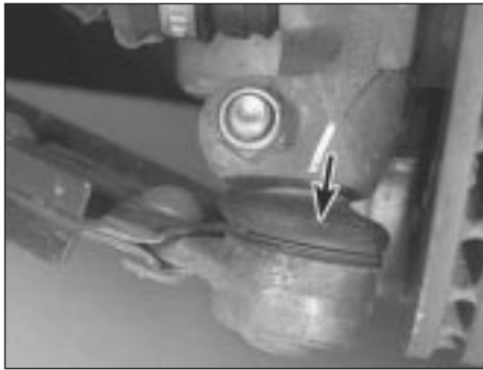
10.2b Check the condition of the lower arm balljoint dust cover (arrowed)
