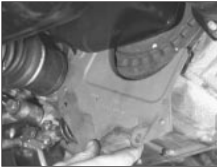
13.7 Removing the clutch cover plate
