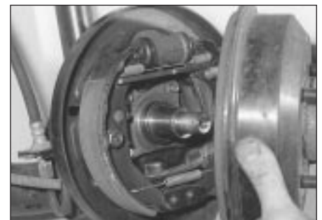
9.5 Slide off the wheel hub/brake drum unit
