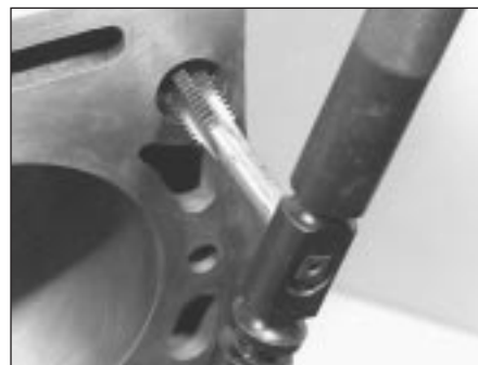
13.6 All bolt holes in the block should be cleaned and restored with a tap
