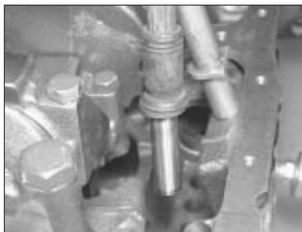
10.6 Tappet withdrawal using a valve grinding tool suction cup
