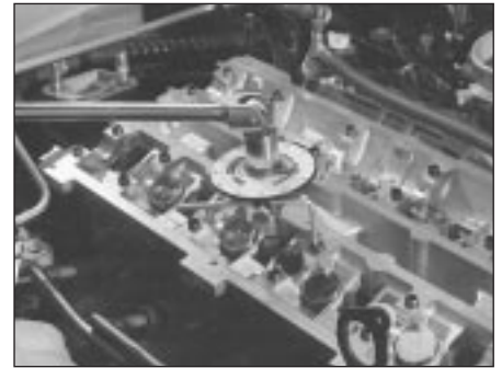
12.28c . . . and to Stage 3 using angle gauge
