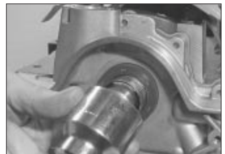
15.5 Socket of correct size can be used to replace Ford service tool, drawing new seal into place as described
