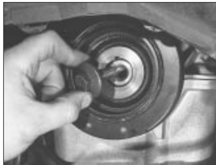
6.9 Unscrew pulley bolt to release crankshaft pulley
