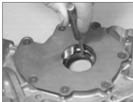
15.2 Driving out crankshaft right-hand oil seal
