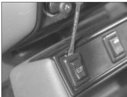
4.20a Prise the centre console switch up from its location . . .
