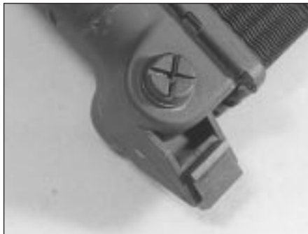
23.3 Drain plug location at the base of the radiator - use a coin to unscrew the plug
