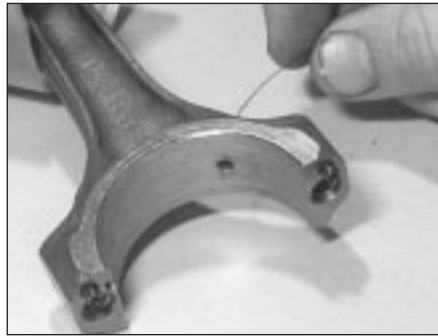
11.24 Check that the connecting rod oilway on CVH engines is clear
