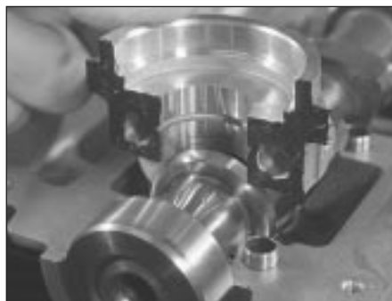
11.19 Apply sealant to mating surface of camshaft right-hand bearing caps
