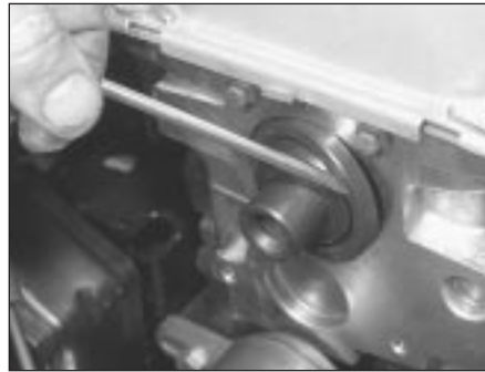
10.2 Camshaft front oil seal removal
