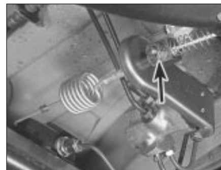
22.3 Light-laden valve linkage adjustment locknut (arrowed)
