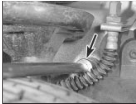
15.8 Unscrew and remove the engine mounting side bolt (arrowed) from under the wheel arch
