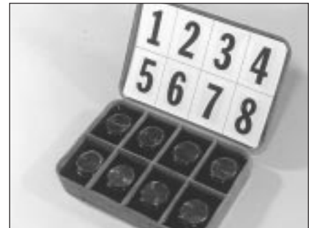
11.6b Store tappets in clearly-marked container filled with oil to prevent oil loss
