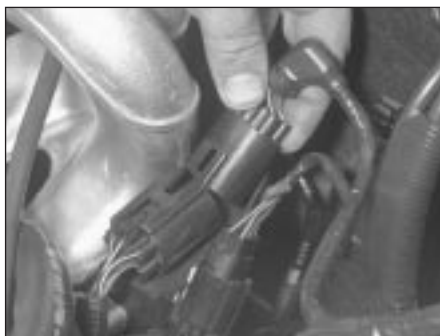
12.7a Unplug engine wiring loom connector alongside the inlet manifold
