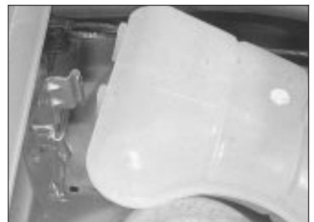
7.22b . . . and release the expansion tank from its retaining bracket
