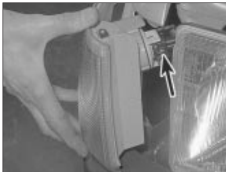
7.7b ... then pull the light unit out to enable the multi-plug (arrowed) to be disconnected
