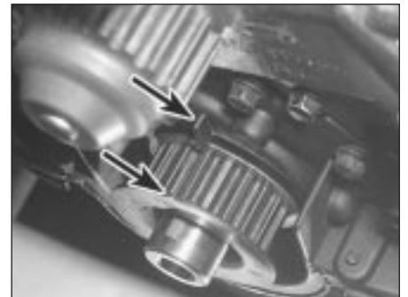
8.7 Sprocket and oil pump housing TDC marks in alignment
