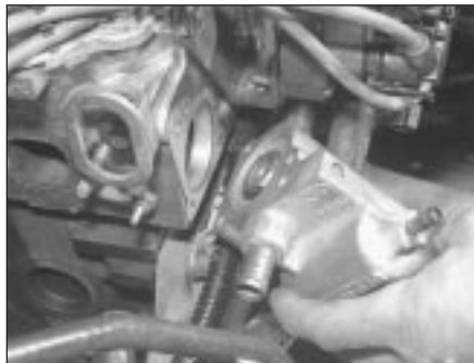
4.6 Removing the thermostat housing from a CVH engine
