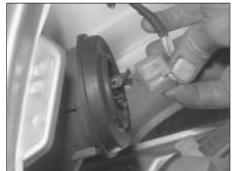
7.2 Disconnecting the multi-plug from the back of the headlight
