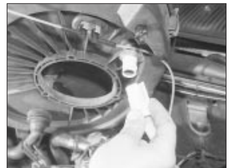
2.4b Disconnecting the intake air temperature sensor multi-plug (CVH engine shown)
