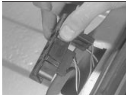
4.46 Withdrawing the luggage area contact plate for access to disconnect the multi-plug
