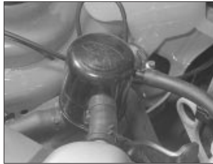
25.5 Crankcase ventilation system filter on CVH engines
