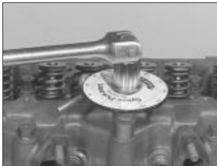
7.27c Cylinder head bolt tightening (Stages 2 and 3) using an angle gauge
