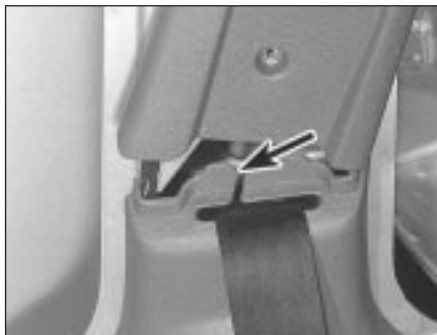
42.23 B-pillar trim being removed to expose seat belt removal/refitting slot in sill scuff plate (arrowed)
