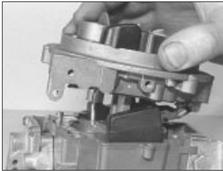
20.5b . . . then detach the carburettor upper body
