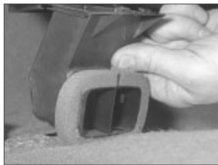
11.27 Removing the footwell vent from the base of the heater casing
