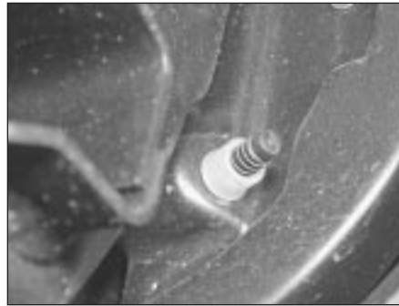
27.3 Handbrake adjuster plunger located on the inside face of each rear brake backplate
