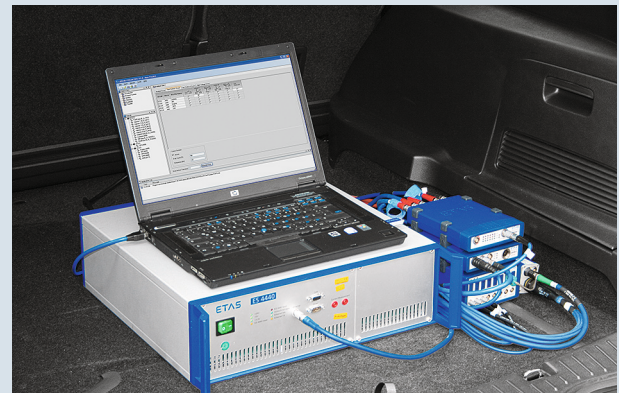
Figure 3: Electric fault simulation in the vehicle.
