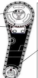
Avoid This Common Mistake when assembling an Opel engine: A common error is when Opel engines are assembled in the #4 TDC position, but not rotated to #1 TDC position before installing distributor.
