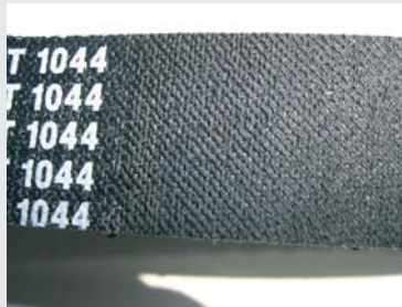
Fig. 2 CT 1044 with belt back fabric
