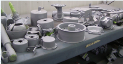
Here, disassembled drivetrain and chassis components that have been re-built are prepped and ready for painting.
