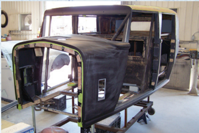
The car retained all its original bodywork, shown here in the final stages of priming and sanding. Primer is water-sanded to prepare the ultra-smooth surface needed for painting.
