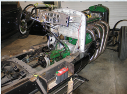
Careful inspection showed that the drivetrain was complete, pictured here during disassembly, and every component was rebuilt and refurbished.
