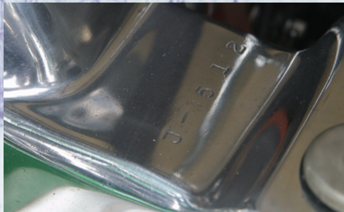
This is a photo of the cast aluminum bell housing that carries the all-important "J number" that all Duesenbergs are known by – J512 (S was understood to be added when the cars were supercharged).
