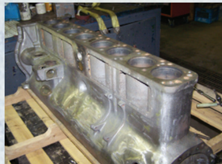
The Duesenberg Model J cylinder block, with its long stroke design and 420-cubic inch displacement, was found to be in excellent condition and only needing minor machine work, new pistons and babbited bearings.
