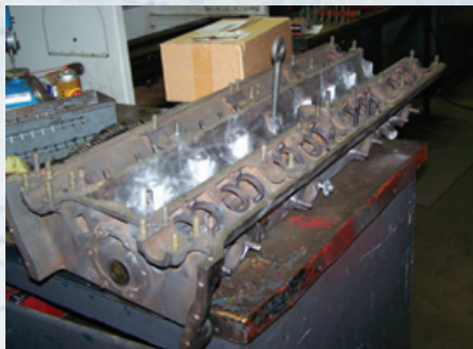
The disassembled Duesenberg Model J cylinder head with four valves per cylinder and dual overhead camshafts. This was the design responsible for the record-breaking, 265 hp output in standard form, 320 hp in supercharged form as found in SJ512.
