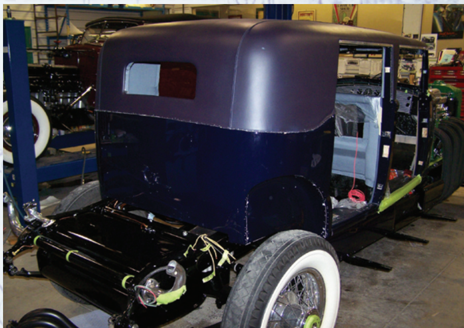
As the finished product comes together, easily scratched freshly painted or chromed components are covered in protective tape to prevent damage from the subsequent work. Here can be seen the new leather roof installed and fitted, waiting for edge trim.
