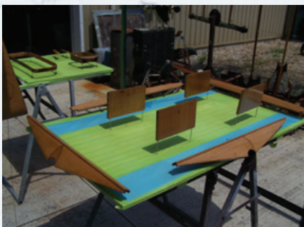
SJ512's original oak interior trim was in excellent shape and was all saved, only requiring stripping, refinishing and minor repairs. Note the subtle and original dual-tone finish on the oak.
