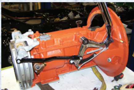
The 3-speed transmission with hand brake finished and ready to re-install. It had previously been completely disassembled and rebuilt with new bearings.
