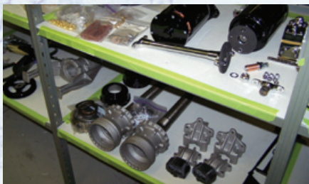
More drivetrain and chassis components disassembled, re-finished and ready to be installed on the chassis. The generator and starter have been rewound and fully rebuilt.
