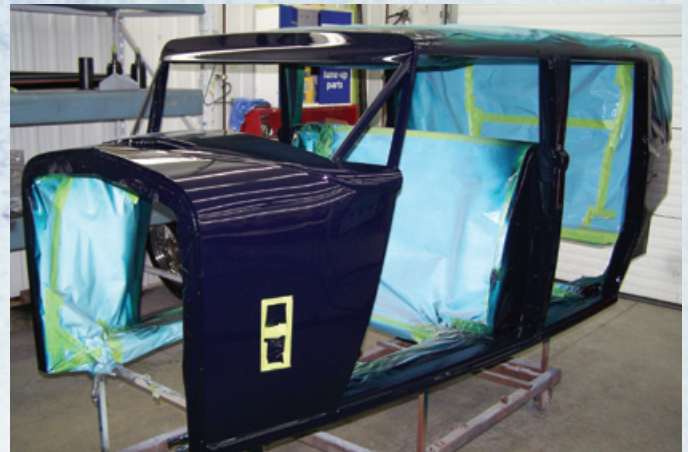
The paint was applied and baked to cure, then color-sanded and machine-polished to a concours-level finish.
