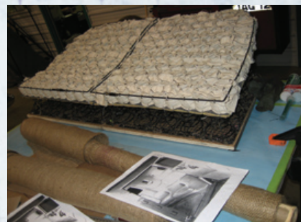
Restoration experts worked from Murphy's original studio photography of the car's interior when new to ensure their handiwork was entirely correct, as seen here during the construction of a seat.
