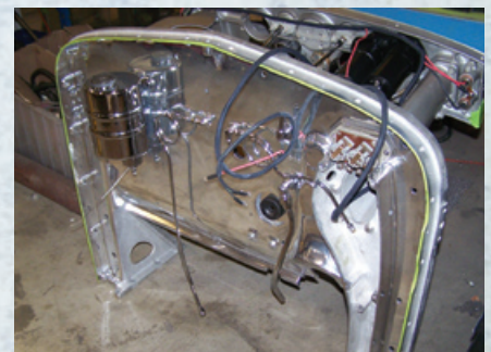
The monumental cast-aluminum firewall and instrument panel assembly is shown here re-polished and newly fitted with wiring and lines.
