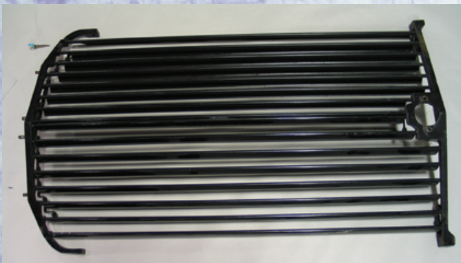
Seen here, the weather-front (radiator shutters) was incorrectly finished, as it was painted instead of chromed.
