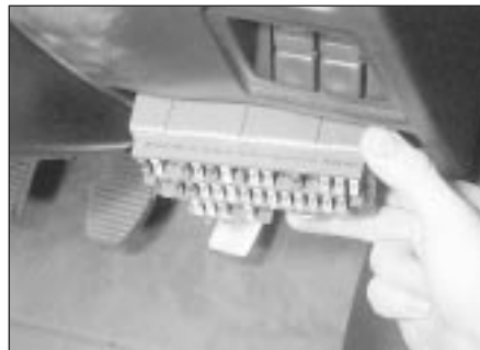
3.11b . . . to release the fusebox - models from 1993
