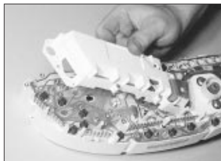
10.8 Removing the cover from the rear of the instrument panel
