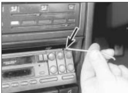
20.13 Make up two removal tools - note slot (arrowed) in end of tool
