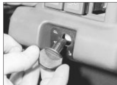
9.5 Prise off the headlight adjuster switch knob
