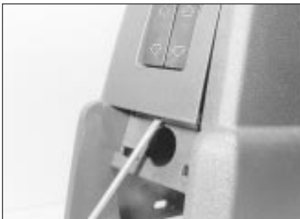
4.24 Prising off a rear centre console switch trim panel . . .
