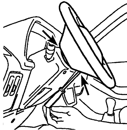
25.7 Turn the steering wheel for access to the two air bag unit screws (arrowed)
