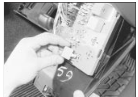
3.14a Removing a relay from the main fusebox - models up to 1992
