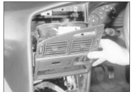
11.15 . . . then withdraw the housing
