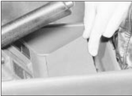
4.19 Prise the trim panel from the bottom of the oddments tray . . .
