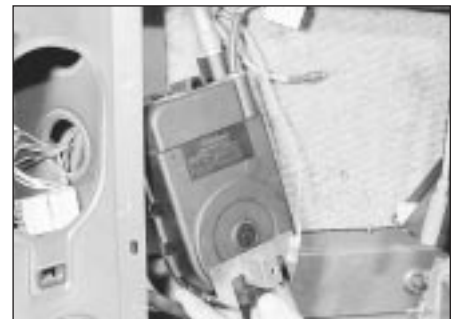
22.18c . . . and withdraw aerial assembly - Estate (rear wing-mounted aerial)
