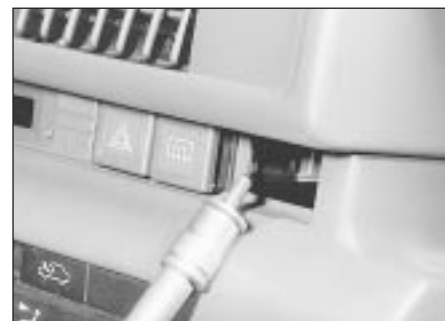
9.3a . . . and remove the visor securing screws
