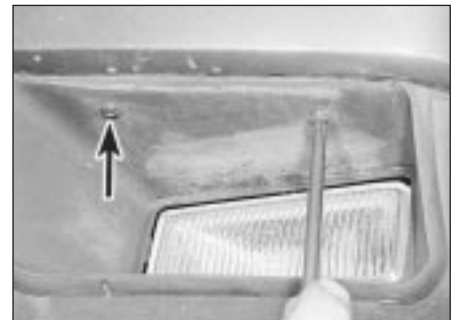
7.16 Remove the front driving light/foglight cowl securing screws
