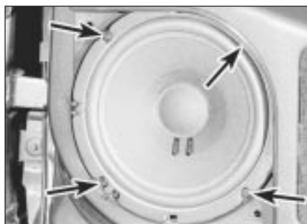
21.3 Door-mounted loudspeaker securing screws (arrowed)
