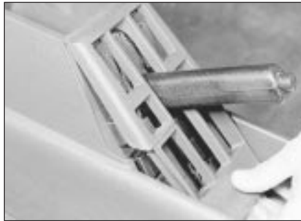
4.20 . . . then prise off the switch trim panel . . .
