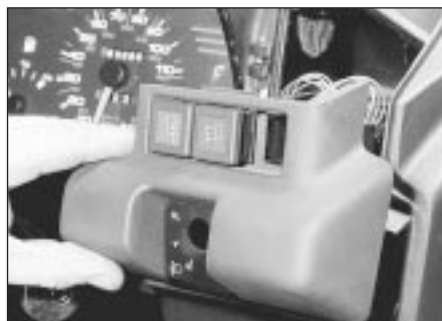
9.6 Withdrawing the driver's side upper facia panel
