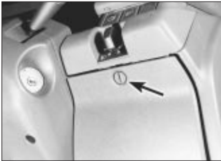
3.3a Release the securing clips (arrowed) . . .
