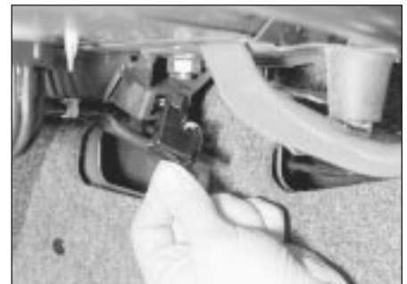
4.35 Removing the luggage compartment courtesy light switch - Saloon model
