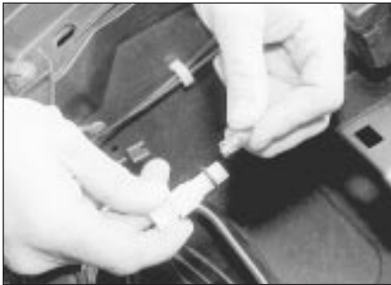
5.11 . . . and withdraw the bulb
