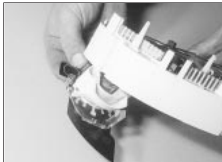
10.11a . . . then withdraw the gauge . . .
