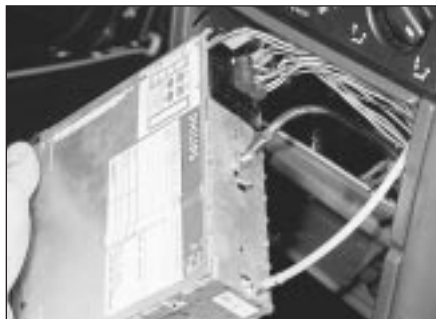
20.4 . . . and withdraw the unit
