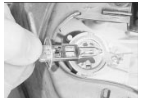
5.23b Removing a headlight-mounted driving light bulb
