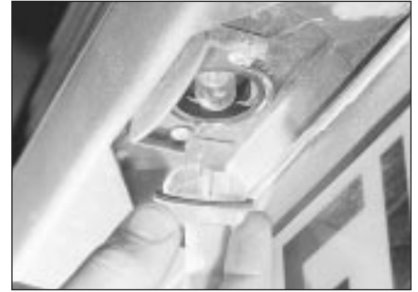
5.39 Prise the lens from the bumper . . .
