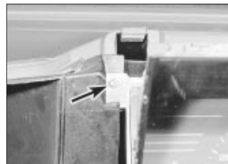
9.8 Instrument panel securing screw (arrowed)
