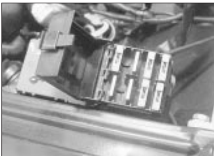
3.4 Fusebox location on right-hand side of engine compartment
