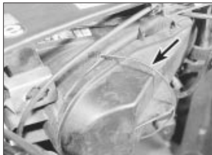
5.2 Headlight rear cover securing clip (arrowed)
