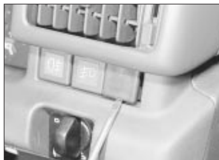
9.2 Prise out the blanking plates . . .
