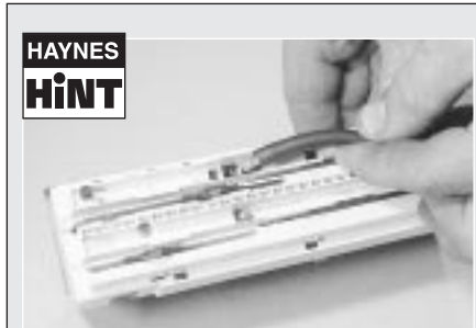
A length of rubber tubing can be used to remove and refit the bulbs
