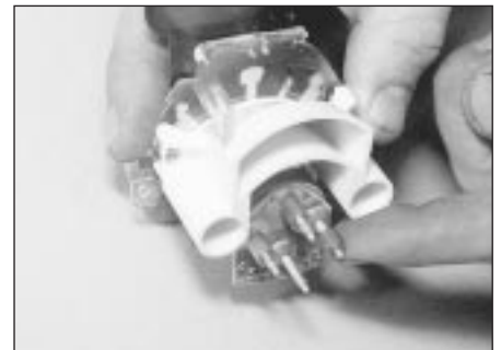
10.11b . . . and recover the spacers from the studs
