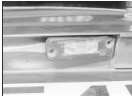
5.42 Prise out the number plate light unit . . .
