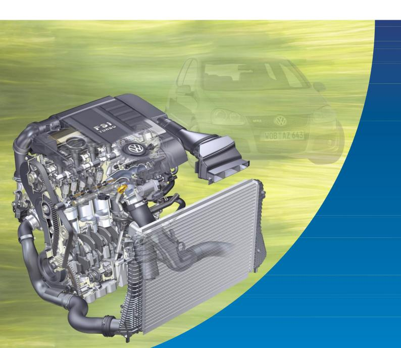
The new FSI engines from Volkswagen do without stratified injection and place greater emphasis on output and torque. Until now, FSI direct injection was always associated with stratification. On the turbocharged engine, the abbreviation FSI remains but there is no stratified charge. Doing without fuel stratification and NOx sensors represents a loss on one part, but also promises the finest driving enjoyment with high output and a torquey engine and great pulling power and economy.
