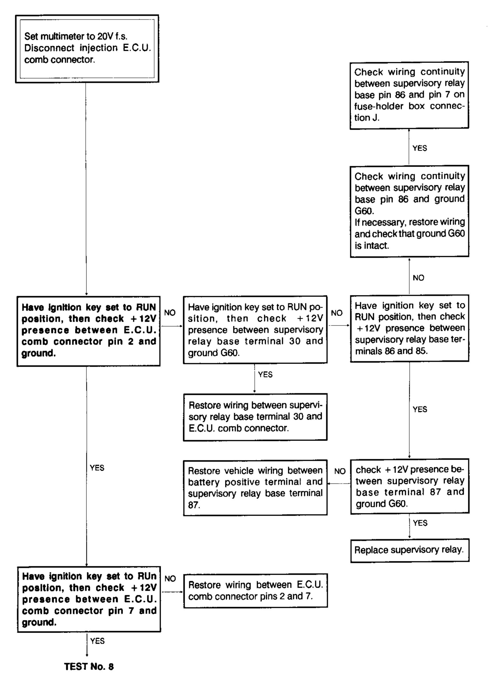
TEST No. 8 - CHECK OF LAMBDA PROBE (E.C.U. PIN 13)
