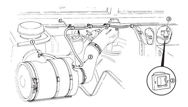
Figure 2-1. Manometer Intake Restriction Test.
