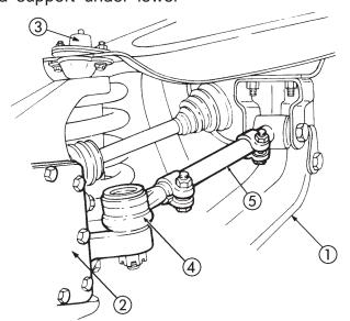
Figure 7-7. Toe-Out Rear Wheel Check Adjustment.
