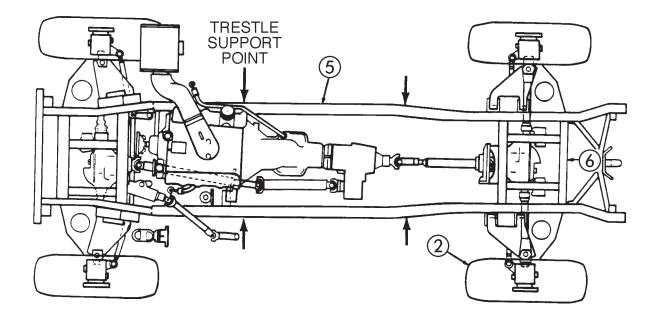
Figure 8-2. Rear and Entire Vehicle Jacking Procedures.
