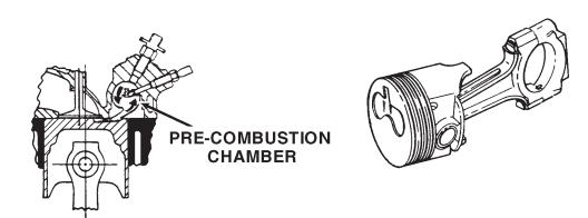
Figure 4-1. Pre-combustion Chamber and Piston Crown Shape.
