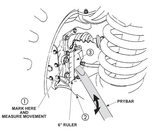
Figure 7-2. Lower Ball Joint Inspection.
