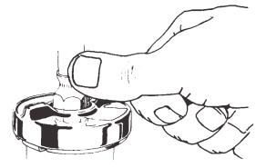
Figure 1-6. Releasing Cooling System Pressure Tester.
