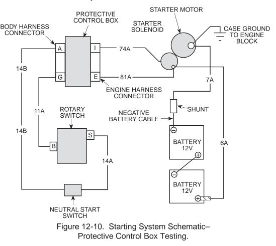
protective control box cannon plugs, neutral start switch lead 14B, starter lead 74A to starter, and negative battery cable to battery.
