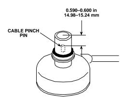
Figure 6-2. Moudlator Pinch Pin Depth.
