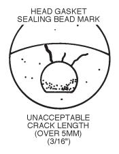
Figure 4-14. Pre-chamber Cracks.
