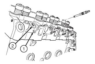
Figure 4-2. Damaged Glow Plug Removal
