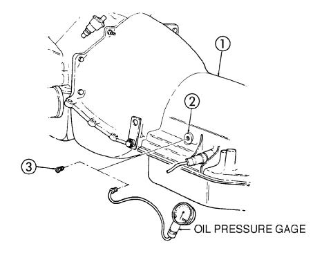
Figure 6-7. Transmission Oil Pressure Gage Removal.
