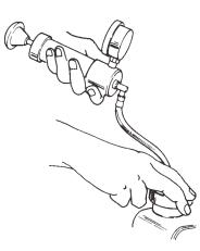
Figure 1-4. Attaching Coolant Pressure Tester
