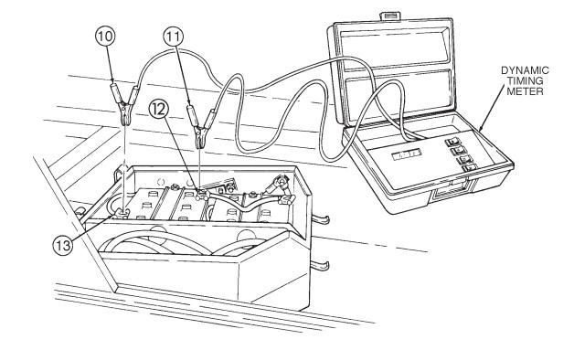
Figure 4-4. Timing Meter Power Hook-up
