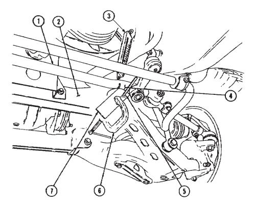
Figure 7-4. Using a Spring Scale Dial Indicator to Check Idler Arm Free Play.
