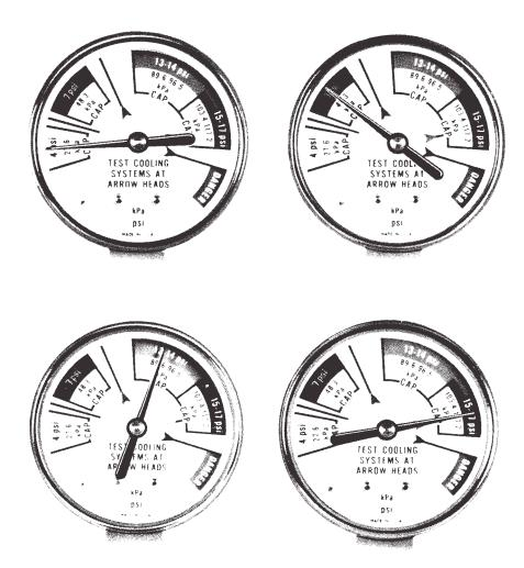
Figure 1-10. Tester Gage Readings.
