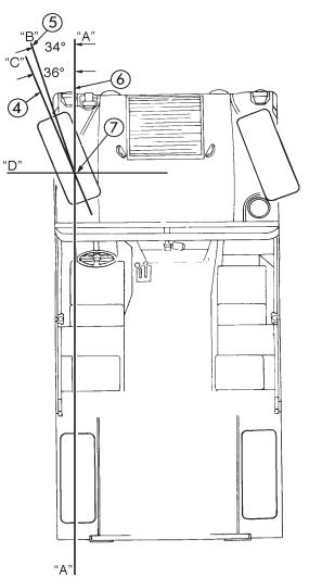
Figure 7-11. Steering Stop Reference line
