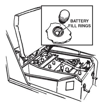
Figure 12-2. Battery Fill Rings.
