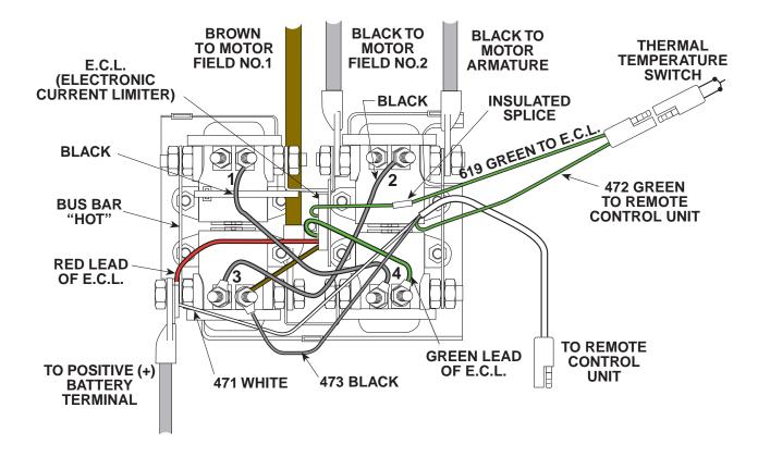
Figure 12-16 Repeat. Winch Testing.
