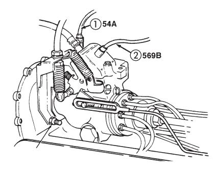
Figure 3-7. Fuel Solenoid Test Hook-up.
