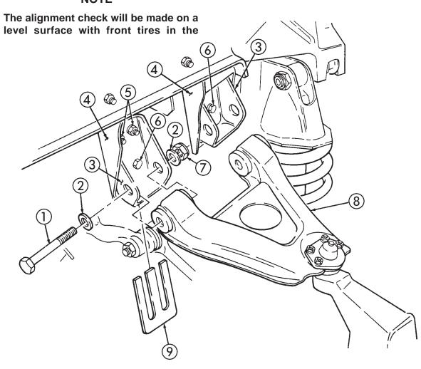
Figure 7-14 . Caster and Camber Adjustment.
