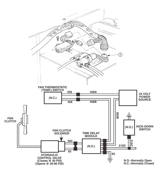
Figure 1-2. Fan Clutch Solenoid Resistance Test Hookup.
