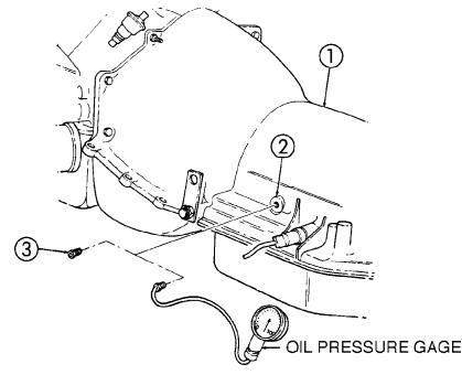
Figure 6-6. Transmission Oil Pressure Test Hook-up.
