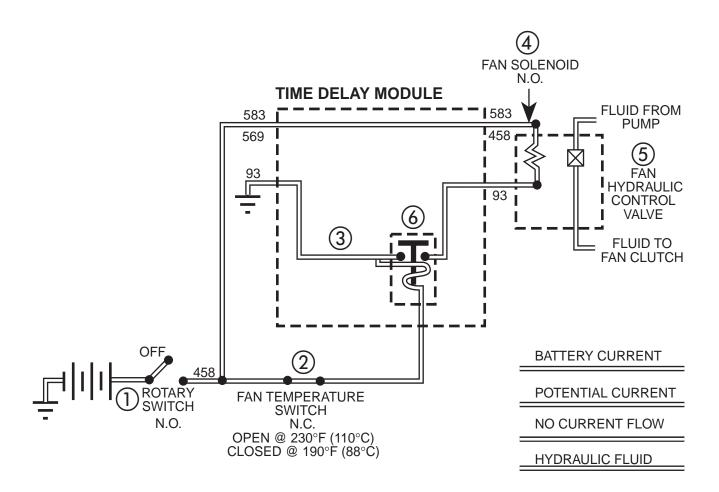
Figure 13-1. Fan Temperature Switch Closed Engine Not Running.
