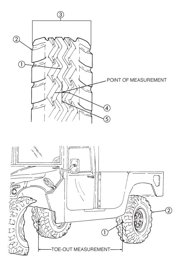
Figure 7-8. Toe-Out Points of Measurement.
