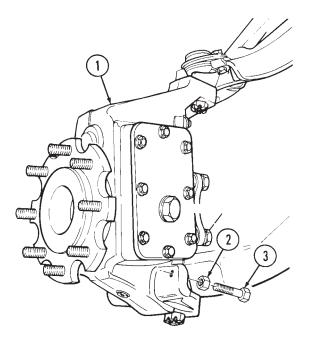
Figure 7-10. Steering Arm Capscrew Adjustment.
