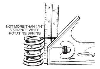
Figure 4-15. Valve Spring Check.
