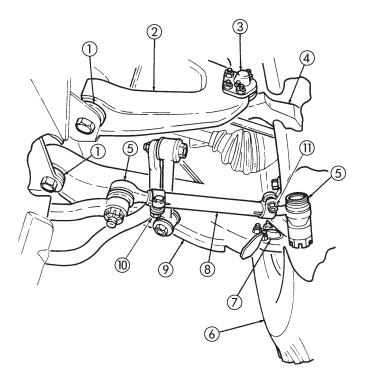
Figure 7-6. Toe-in/Front Wheel Check
