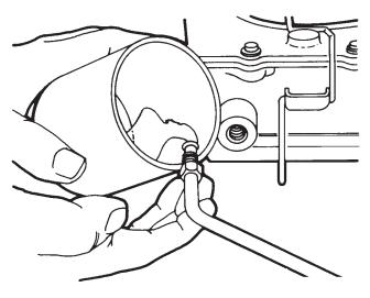
Figure 3-13. Fuel Flow Test.
