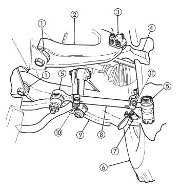
Figure 7-1. Toe-in Front Wheel Check and Adjustment.
