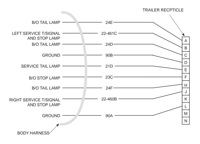
Figure 12-15. Trailer Lighting System Schematic.
