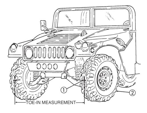
Figure 7-5. Toe-in Measurement Check.
