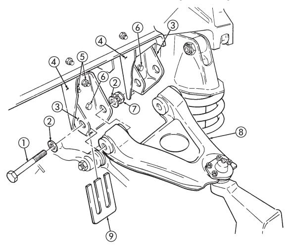
Figure 7-14 (Repeat). Caster and Camber Adjustment.
