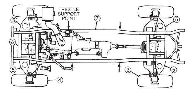
Figure 8-1. Front and Corner Jacking Procedures.
