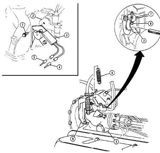
Figure 6-9. Kick-down Switch Adjustment.
