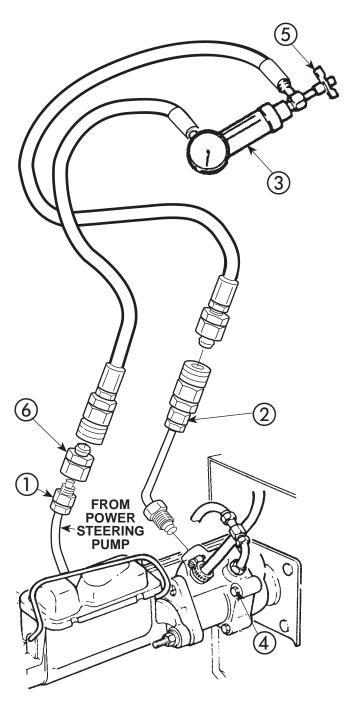
Figure 9-1 Repeat. Power Steering Test Hook-up.
