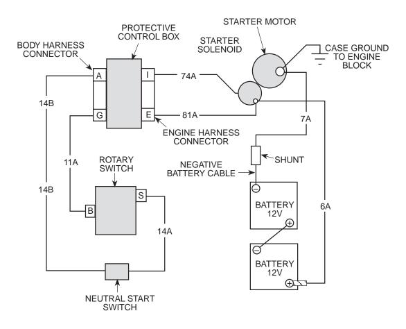
Figure 12-10. Starting System Schematic– Protective Control Box Testing.
