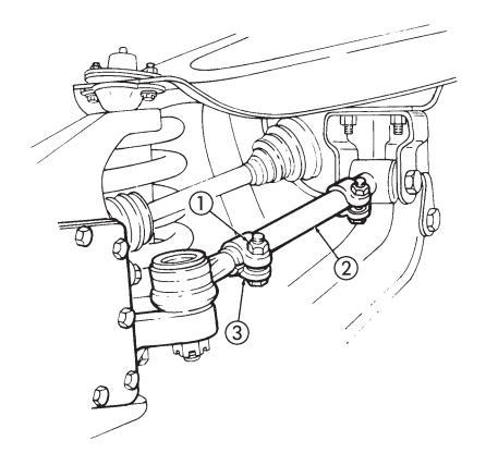
Figure 7-9. Toe -out Adjustment.
