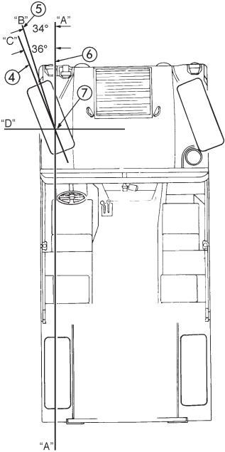
Figure 7-12. Repeat. Steering stop Check and Adjustment.
