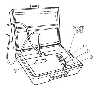
Figure 4-7. Timing with Dynamic Timing Meter.
