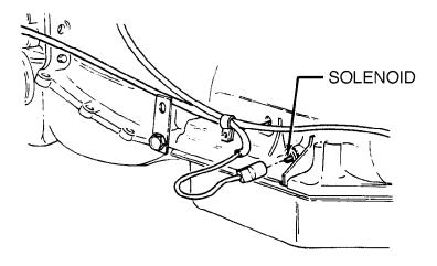
Figure 6-8. Transmission Detent Solenoid Resistance Test.
