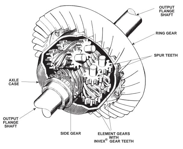
Figure 11-1 Repeat. Torsen Differential.
