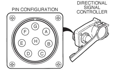
Figure 12-14. Turn Signal Pin Configuration.
