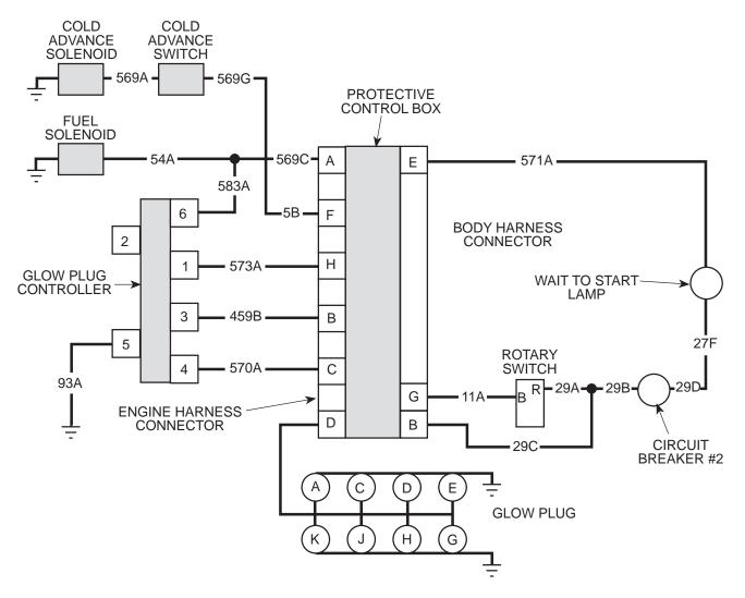
Figure 12-3. Glow Plug Controller Testing
