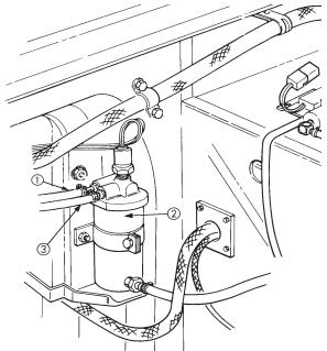
Figure 3-4. Fuel Filter Pressure Test Hook-up
