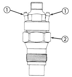
Figure 3-6. Fuel Injector Nozzle.
