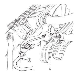
Figure 1-3. Fan Clutch Valve Pressure Test Hookup.
