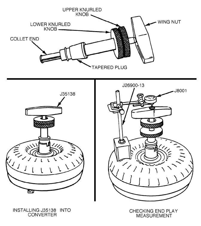
Figure 6-11. Torque Converter Checks.
