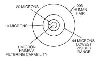
Figure 3-15. Relative Size of Micron Particles
