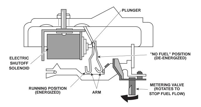
Figure 3-9. Electrical Shutoff Solenoid.
