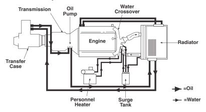
Figure 1-12. Cooling System Schematic.
