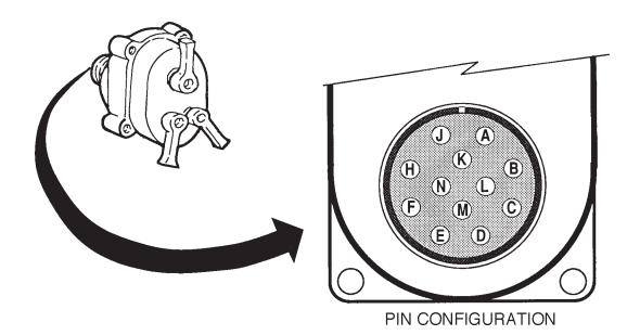
Figure 12-12. Master Lightswitch Pin Configuration.
