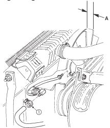
Figure 1-11. Fan Shroud Adjustment.
