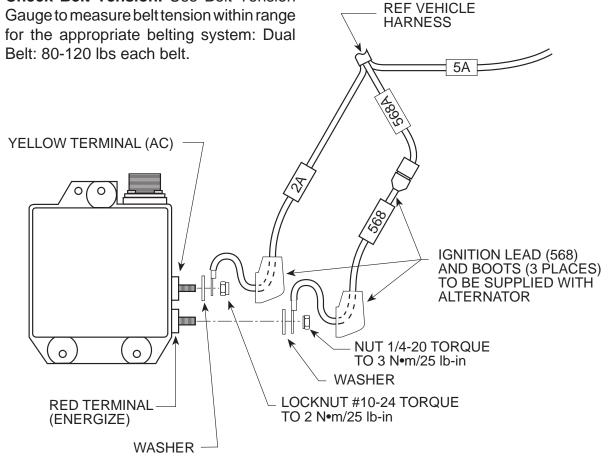
Figure 12-7. **Regulator AC and Energize Terminals**
