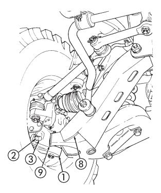
Figure 7-13. Steering Stop Adjustment and Lower Contrtol Arm
