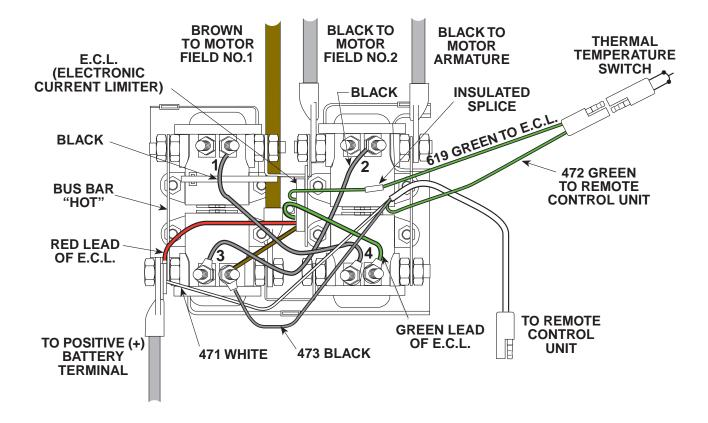
Figure 12-16. Winch Testing.
