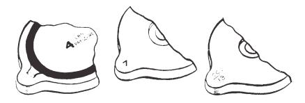
Figure 1-7. Pressure Cap Markings
