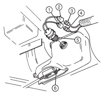
Figure 5-3. Parking Brake Switch.
