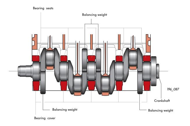
You must not remove or loosen the crankshaft in the 1.4-ltr. engine.
