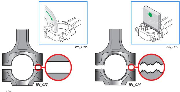
As a rule, con rods must be replaced as a set. Don't forget to mark which con rod belongs to which cylinder.
