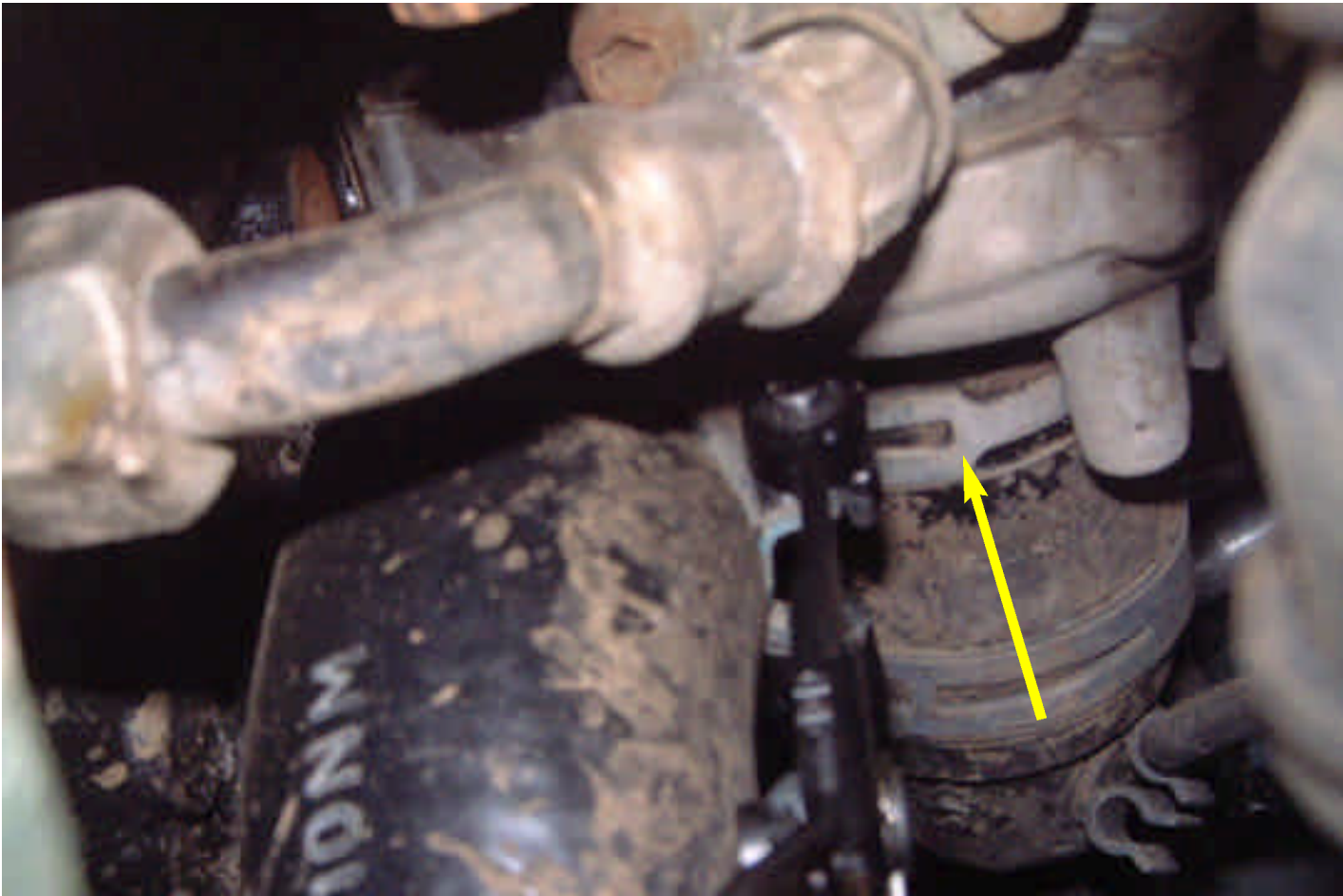
Crawl under the car and at the back of the engine above the passenger side drive shaft is the turbo compressor outlet pipe. Using your flat band clamp" pliers, remove the spring on turbo compressor outlet.
