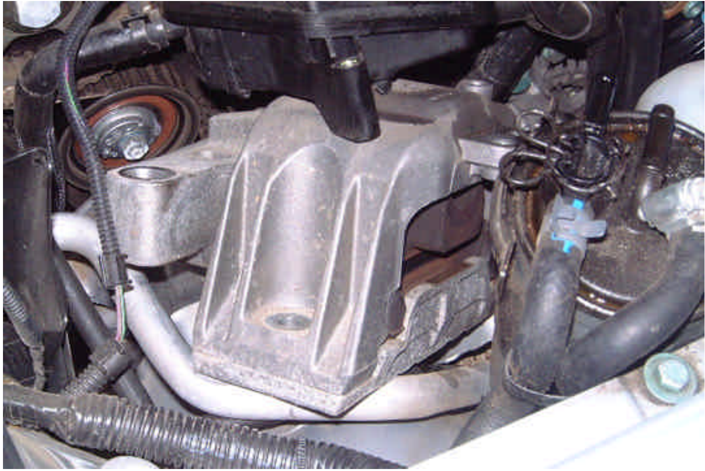
Slide the engine mount out of its position and remove from the car.
