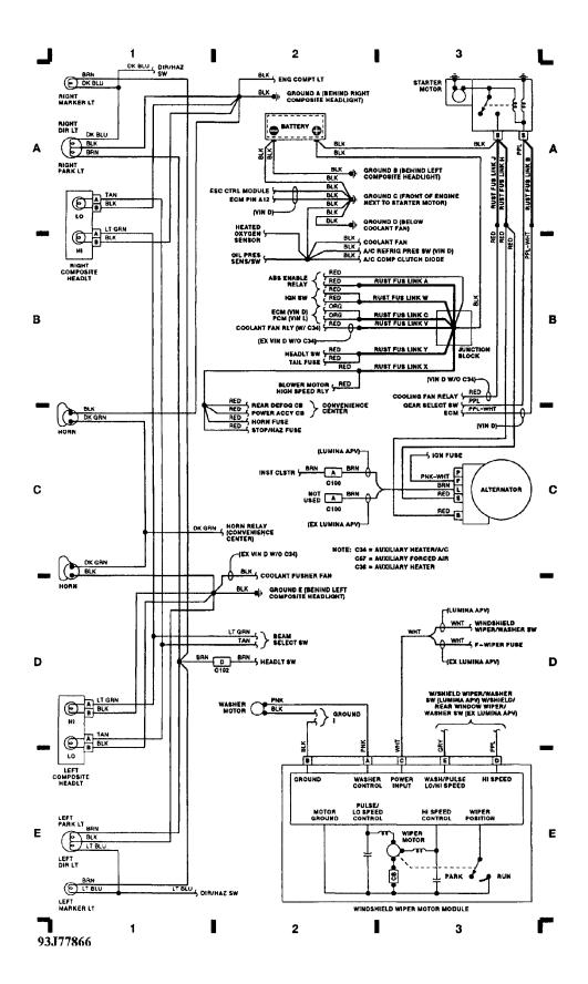
WIRING DIAGRAMS Fig. 2: Electronic Control Module (3.1L V6 VIN D) (Grids 4-7) (p. 2) 1993 Pontiac Trans Sport
