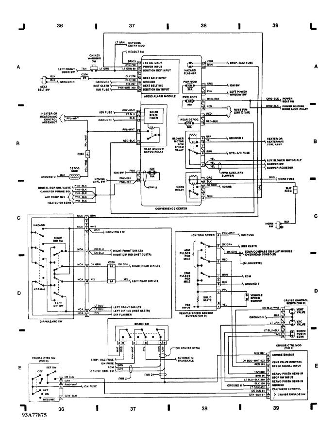
WIRING DIAGRAMS Fig. 11: Headlt Sw, W/Shield Wiper/Washer Sw (Grids 40-43) (p. 11) 1993 Pontiac Trans Sport
