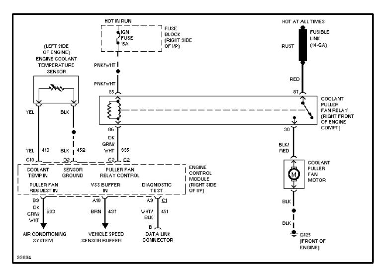
SYSTEM WIRING DIAGRAMS 3.8L (VIN L), Cooling Fan Circuit (p. 3)
