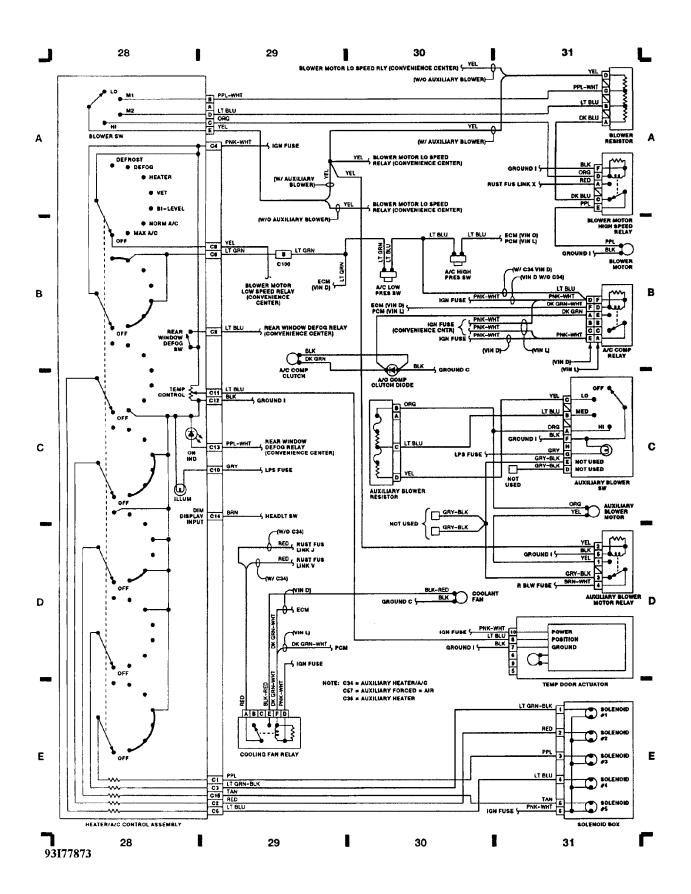
WIRING DIAGRAMS Fig. 9: Heater Control Assembly, Solenoid Box (Grids 32-35) (p. 9) 1993 Pontiac Trans Sport
