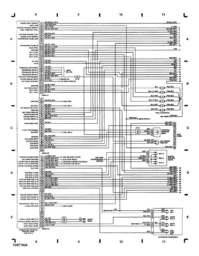
WIRING DIAGRAMS Fig. 4: Cruise Control Servo, Sw, Fuel Pump Relay (Grids 12-15) (p. 4) 1993 Pontiac Trans Sport
