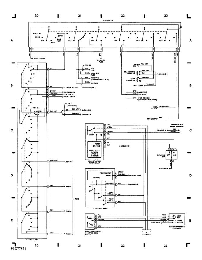
WIRING DIAGRAMS Fig. 7: Electronic Brake Control MOD (Grids 24-27) (p. 7) 1993 Pontiac Trans Sport
