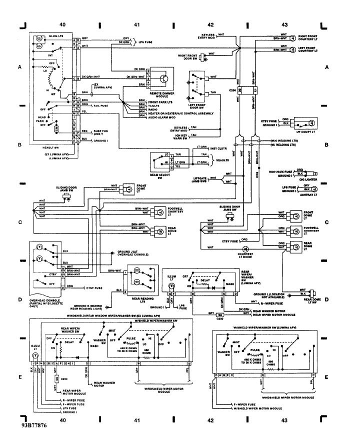
WIRING DIAGRAMS Fig. 12: Instrument Cluster, Mirror Switches (Grids 44-47) (p. 12) 1993 Pontiac Trans Sport
