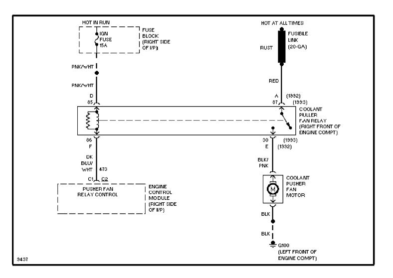
SYSTEM WIRING DIAGRAMS 3.1L (VIN D), Cooling Fan Circuit, W/O Pusher Fan (p. 2) 1993 Pontiac Trans Sport
