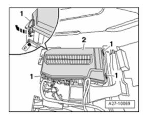
= Remove cover - 2 - over battery by releasing retaining clamps - 1 - - arrow - .
