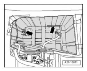
Insert battery in battery mount so that base strip engages in battery mount retaining strips arrows - .
