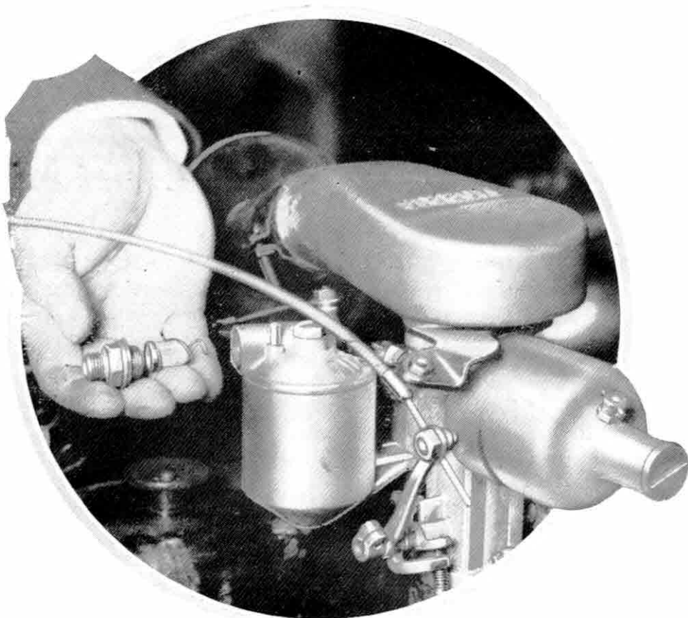
The petrol feed pipe removed to show the filter
