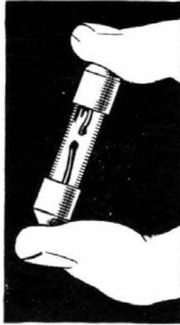
The appearance of a blown fuse.
