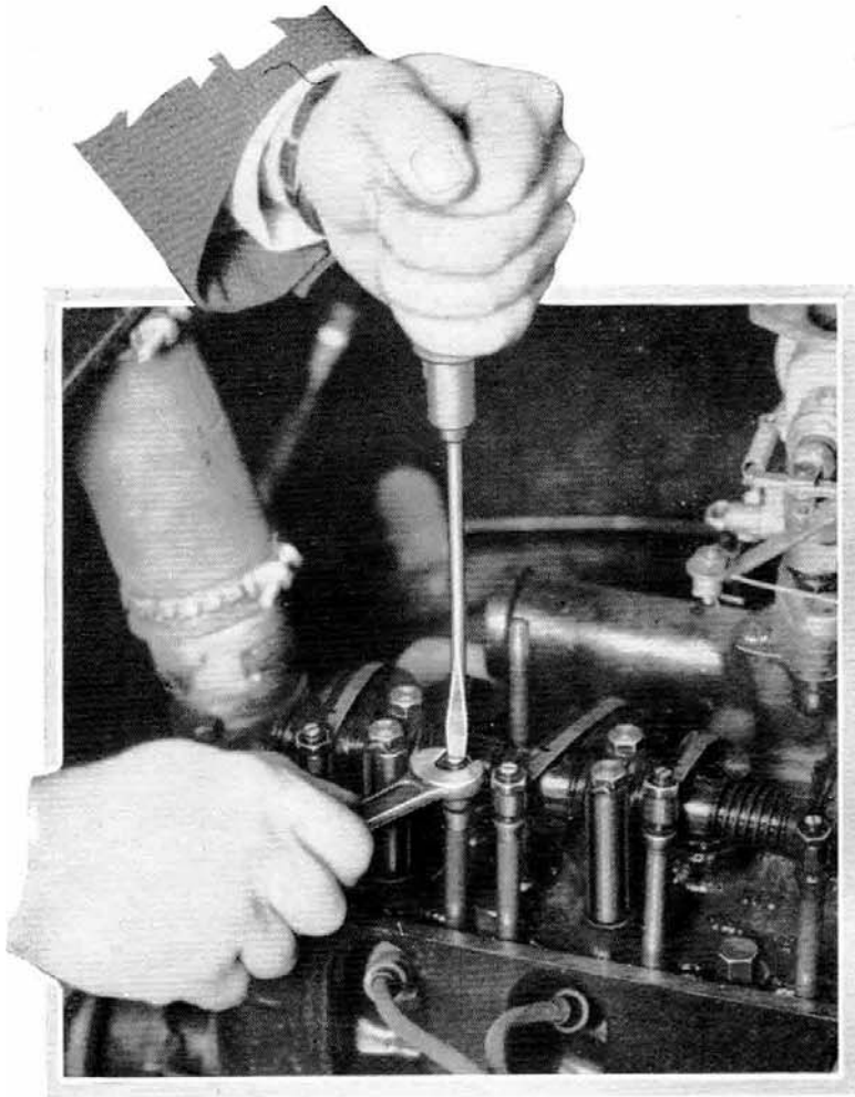
Left :- The tappet adjustment screw is released for adjustment by slackening off the hexagon lock nut with a spanner while holding the tappet screw against rotation with a screwdriver. The tappet screw is relocated in a similar manner after adjustment
