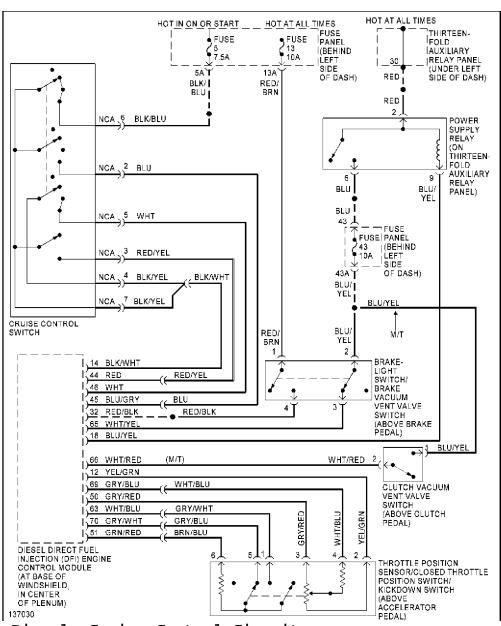
1.9L Turbo Diesel, Cruise Control Circuit
