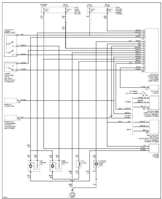
Cooling Fan Circuit, Manual A/C
