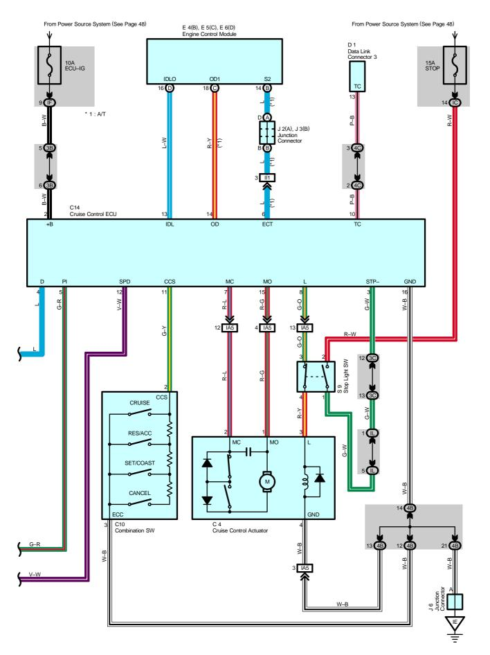
The current is applied at all times through the STOP fuse to TERMINAL 2 of the stop light SW.
