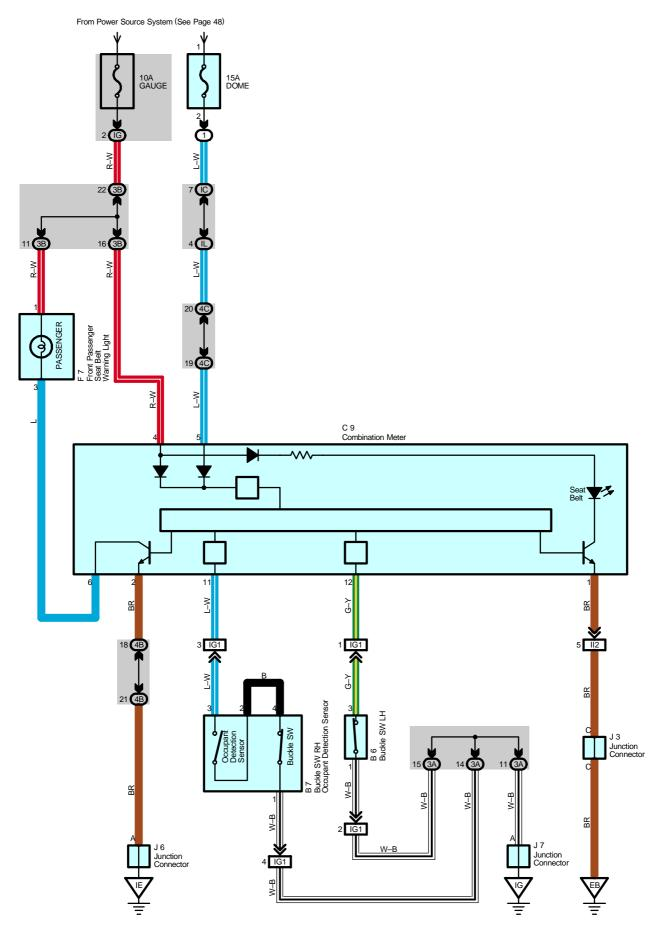
Current is always applied from the DOME fuse to TERMINAL 5 of the combination meter. When the ignition SW is turned to ON position, the current from the GAUGE fuse flows to TERMINAL 4 of the combination meter and flows TERMINAL 1 of the front passenger seat belt warning light.
