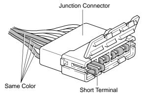
Junction connector in this manual include a short terminal which is connected to a number of wire harnesses. Always perform inspection with the short terminal installed. (When installing the wire harnesses, the harnesses can be connected to any position within the short terminal grouping. Accordingly, in other vehicles, the same position in the short terminal may be connected to a wire harness from a different part.)
