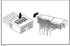
Push the terminal retainer down to the temporary lock position.
