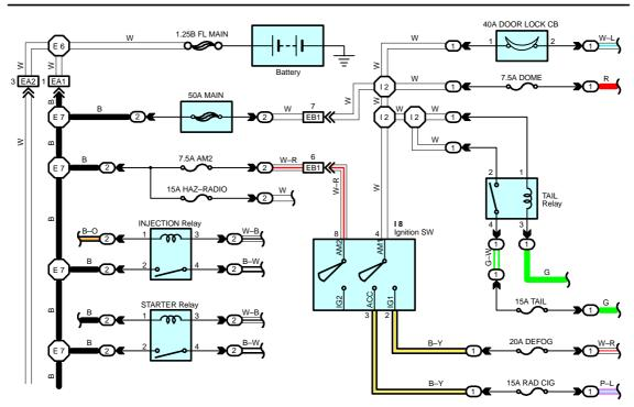
\* The system shown here is an EXAMPLE ONLY. It is different to the actual circuit shown in the SYSTEM CIRCUITS SECTION.
