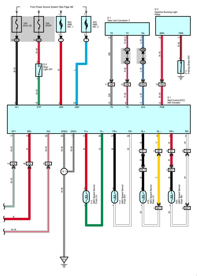
ABS is a brake system designed to improve the operating ability and securing the stability of the vehicle by preventing the lock–up of the vehicle by controlling the wheel cylinder pressure of all the four wheels at the time of sudden braking.
