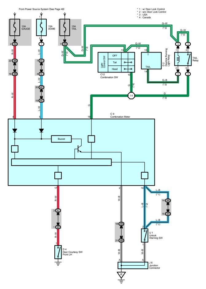
The current is applied at all times to TERMINAL 5 of the combination meter through the DOME fuse.
