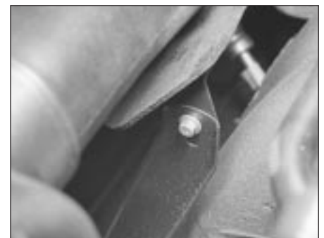
2.3 Forward air trunking to support bracket bolt
