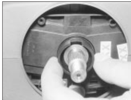
18.8 Position the direction indicator cancelling bush with the slot pointing upwards
