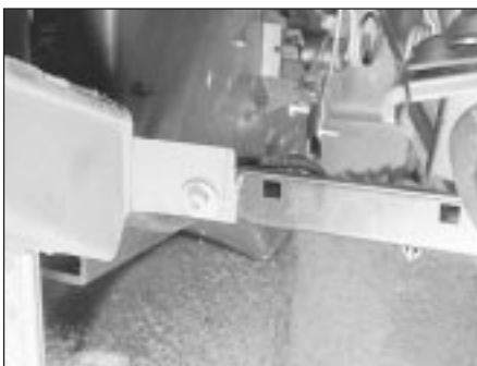
48.13 Undo the cross-brace screws
