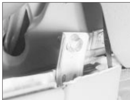
48.14 Undo the bolt at the fascia lower end
