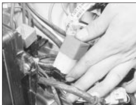
4.17 Remove the relay behind the ignition/fuel ECU
