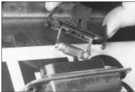
5.41 . . . squeeze the two plastic tags together and release the bulbholder from the light unit
