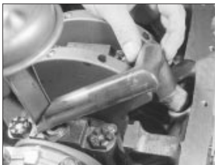
13.5 Remove the crankcase breather tube extension tube
