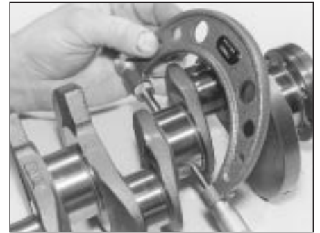
17.4 Measuring the main bearing journal diameters
