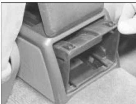
47.6 Remove the rear ashtray and insert . . .
