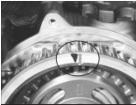
12.9a Front camshaft sprocket timing mark, aligned with the corresponding line in the backplate
