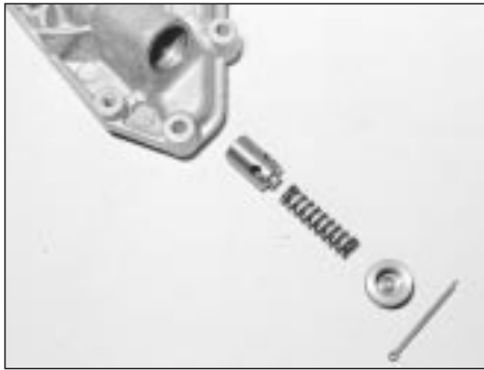
15.2 Oil pressure relief valve components
