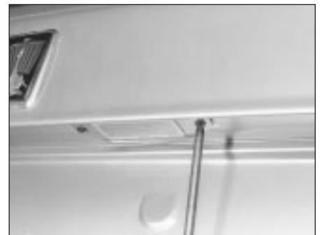
7.15 Undo the two screws securing each number plate light unit
