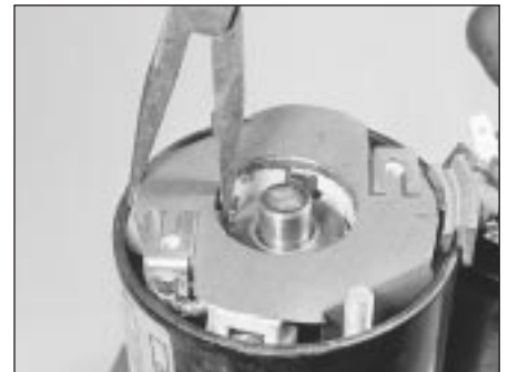
22.10 Using pointed-nose pliers to compress the brushes
