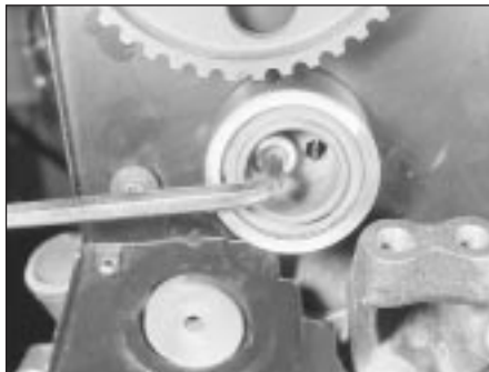
11.3 Undo the timing belt idler pulley bolt
