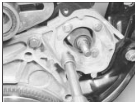
26.15 Undo the four pump retaining bolts
