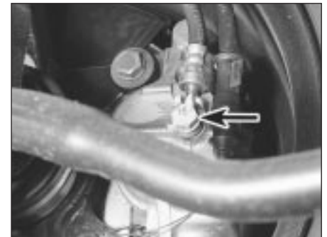
15.10 Front brake hose-to-caliper banjo union bolt (arrowed)
