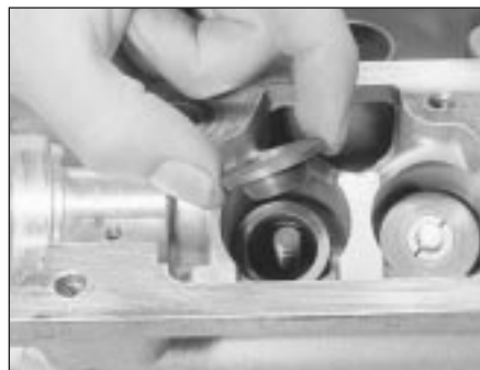
7.3a Release the compressor, and lift off the spring top cup . . .
