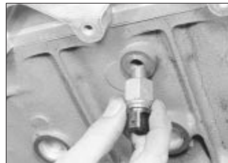
12.3b . . . then unscrew the sensor
