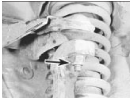
2.12 Undo the upper suspension arm balljoint nut (arrowed)
