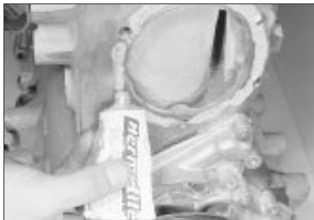
9.13 Apply RTV sealant to the cylinder block mating face
