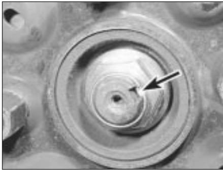
2.2 Knock up the staking (arrowed) securing the driveshaft retaining nut
