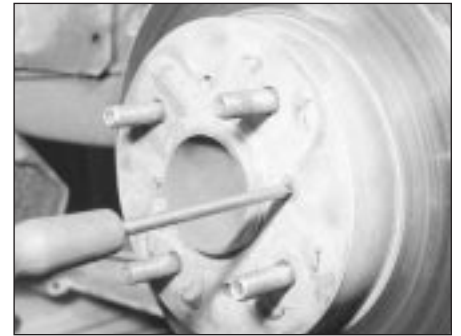
10.7a Undo the two retaining screws . . .
