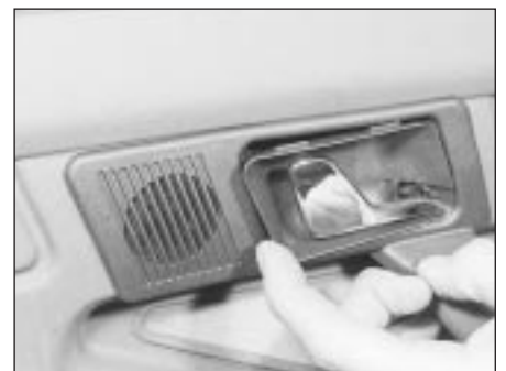
21.3a On later models, prise out the inner handle centre finisher trim . . .
