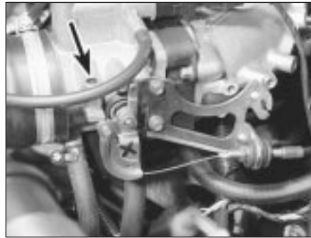
11.17 Base idle speed adjusting screw tamperproof plug (arrowed)
