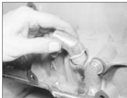
13.4 Withdraw the crankcase breather tube elbow
