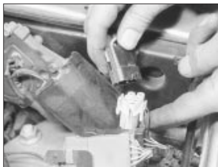
16.8 Disconnect the motor wiring multiplug
