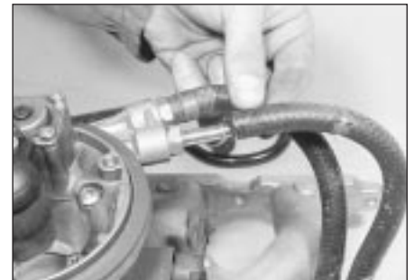
12.16 Release the two fuel hose retaining clips at the injector housing, and disconnect the two hoses
