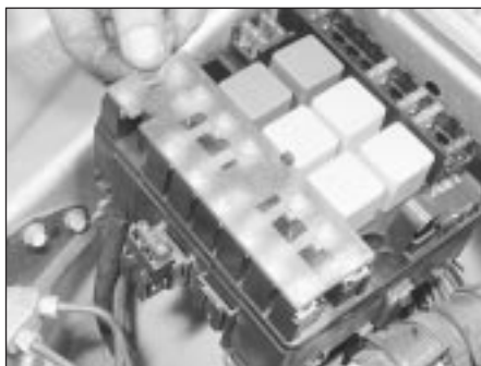
3.10 Lift off the protective cover for access to the fusible links
