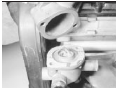
4.3b . . . and remove the water outlet elbow
