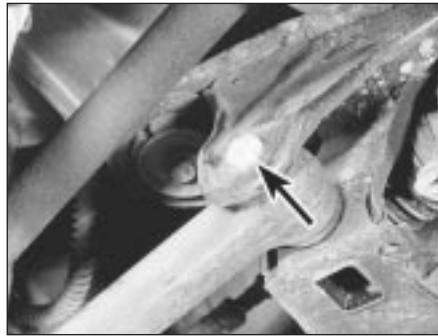
8.6 Lower suspension arm inner mounting bolt (arrowed)
