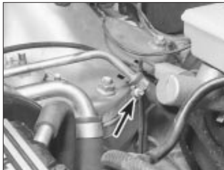
4.30 Disconnect the power steering fluid return hose (arrowed)
