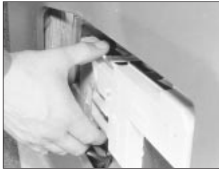
5.26a Lift the top retainer on the bulb panel, press the two bottom retainers and withdraw the panel
