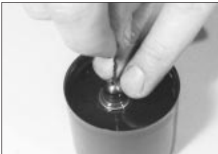
15.24b . . . immerse the tappet in oil and push the valve inside in and out to remove all the air
