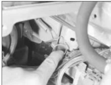
5.13 Unhook the direction indicator lens retaining spring
