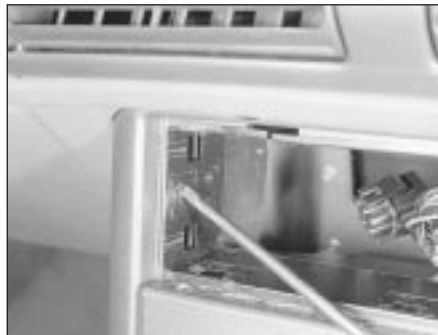
48.8a Release the radio mounting plate retainers (arrowed) . . .
