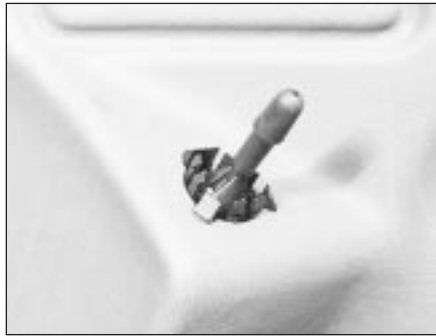
21.13b . . . release the stalk retaining clips and push the stalk through the panel
