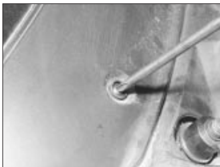
16.4a Undo the screws on the finisher front face . . .
