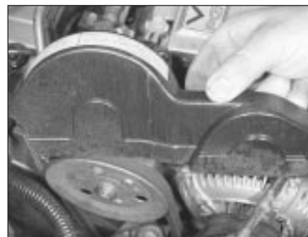
26.27d . . . and lift off the two covers
