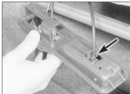
44.3 Extract the outer cable retaining clip (arrowed) at the lever surround . . .
