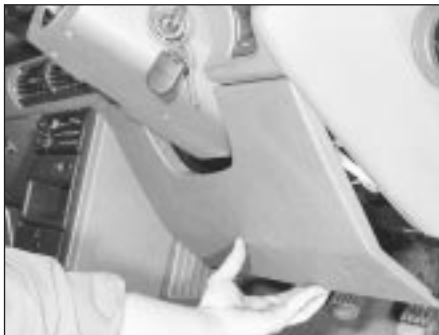
21.3a Remove the upper trim panel . . .
