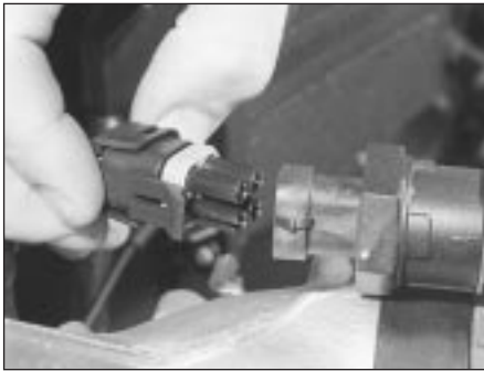
11.14 Disconnect the stepper motor wiring multiplug
