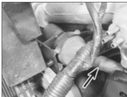
12.17 Detach the hose from the diverter valve (arrowed)
