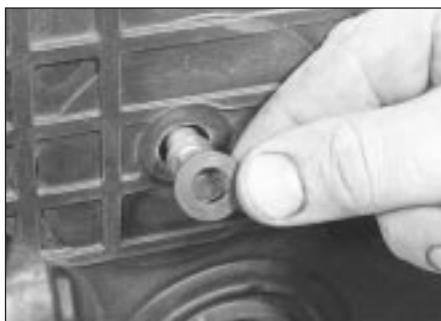
11.11 Release the rubber grommet from the protruding head of the timing belt tensioner retaining bolt
