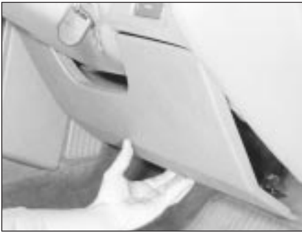
3.2a Lift away the trim panel for access to the fusebox . . .
