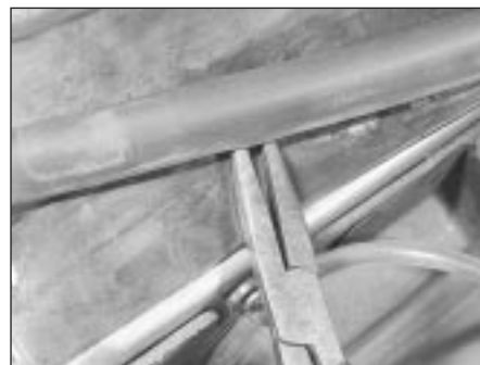
16.5a Release the rubber sealing strip retaining clips . . .
