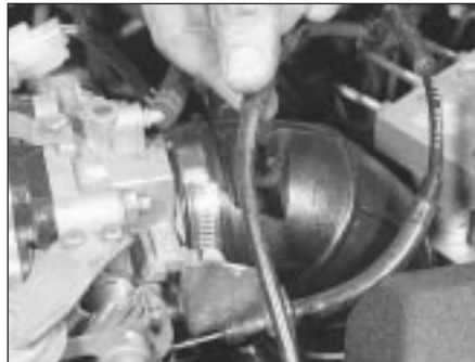
2.1 Release the coil HT cable from the clip on top of the upper intake trunking
