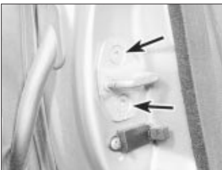
22.8 Door striker plate retaining screws (arrowed)
