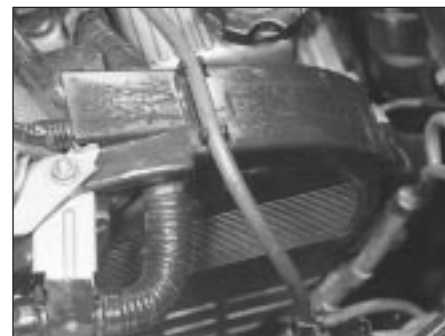
16.27 On V6 engines, remove the pulley covers over the top of the engine ...
