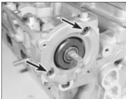
10.10 Undo the two screws (arrowed) and remove the distributor adaptor plate
