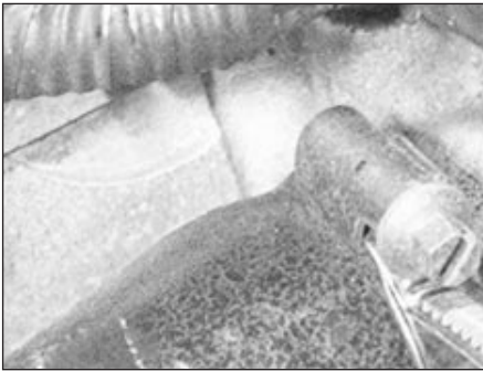
5.10 Slacken the clips and disconnect the coolant hoses at the thermostat housing
