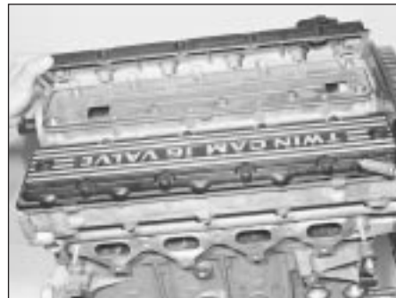
4.4b . . . and remove the covers
