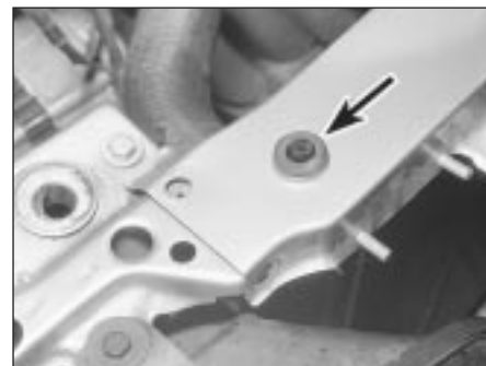
7.12b . . . and the centre platform grommets (arrowed) locate over the radiator upper lugs
