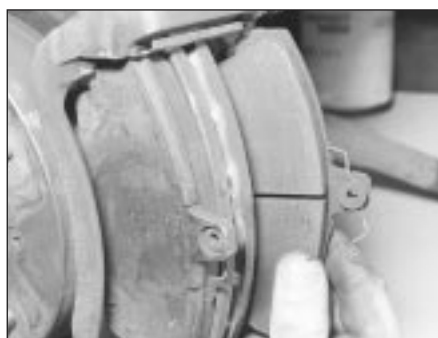
3.4a Lift out the brake pads together with their shims
