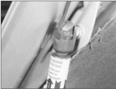
6.7 Prise out the support strut retaining clips
