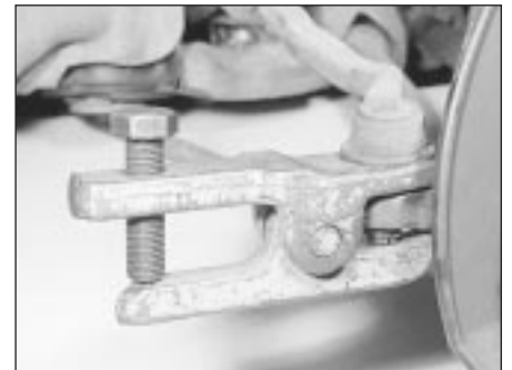
22.4 Using a universal balljoint separator tool to release the track rod balljoint
