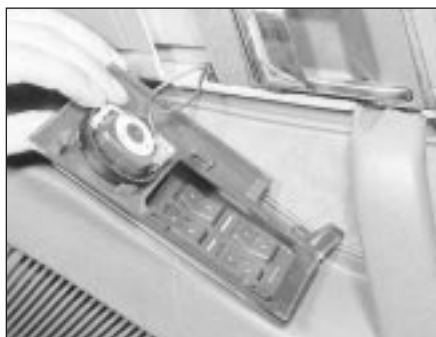
21.2b . . . and disconnect the tweeter speaker leads
