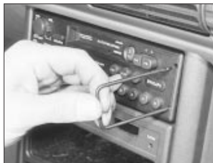
19.2 Insert the radio removal tools into the holes on the edges of the unit
