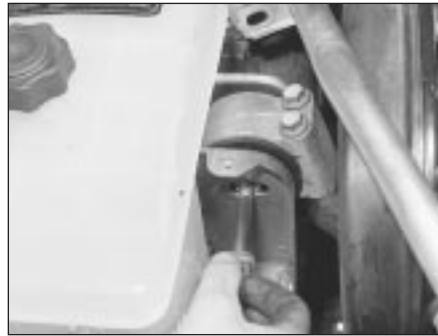
7.7 Undo the engine right-hand mounting through-bolt
