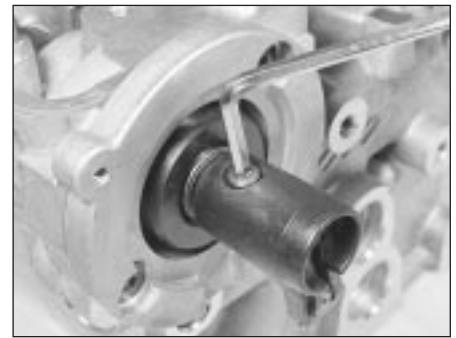
5.3b . . . then undo the rotor arm grub screw
