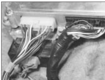
12.80 Disconnect the ECU wiring multiplugs
