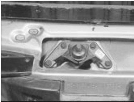
16.15a Wiper linkage centre spindle assembly . . .
