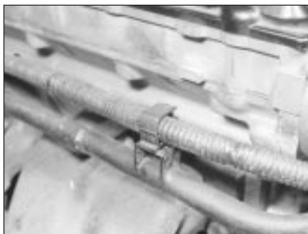
12.13 Release the wiring harness clips from the bypass pipe
