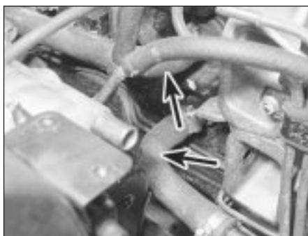
4.12b . . . and the heater hoses at the heater matrix (arrowed)
