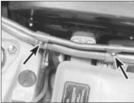
7.6 Undo the bolts securing the power steering pipe support brackets (arrowed)
