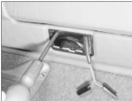
21.10 Undo the screw behind the blanking plate or interior light
