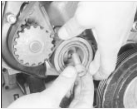
7.14 Removing the timing belt tensioner
