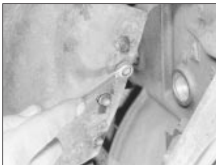
6.8a Undo the bolts securing the two halves of the manifold stove . . .
