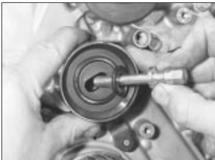
13.3 Remove the tensioner retaining bolt, lift off the tensioner and remove the spring
