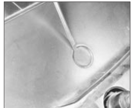
16.3 Prise up the windscreen finisher screw caps
