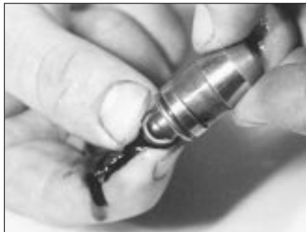
15.29 Depress the internal tappet valve to drain the oil prior to installation
