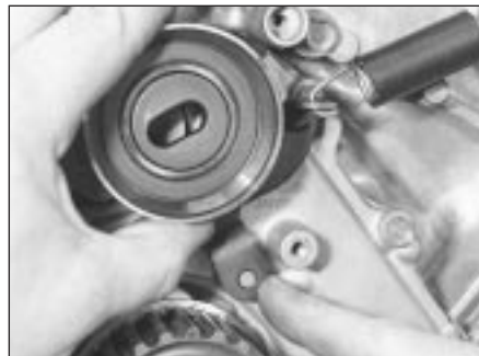
13.5 Ensure that the lower tensioner arm engages over the lug in the casing when refitting
