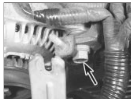
16.29a ... slacken the alternator side pivot bolt (arrowed) ...
