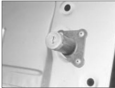
10.4 Boot lid private lock retaining rivets
