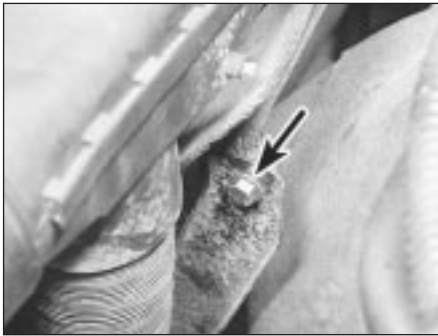
2.5c ... and the air cleaner trunking to support bracket bolt (arrowed)
