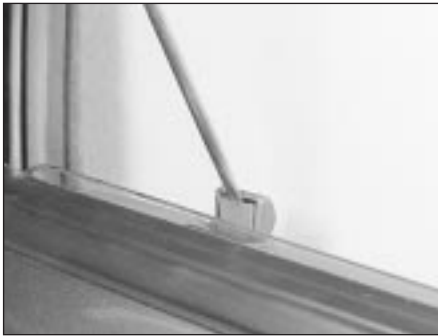
21.1a Prise apart the interior lock button . . .
