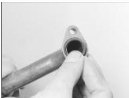
13.14 Fit a new O-ring to the pick-up pipe flange
