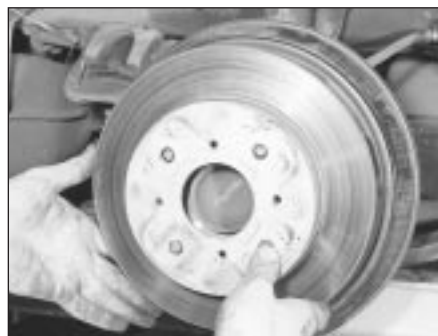
10.7b . . . and withdraw the rear disc from the hub flange
