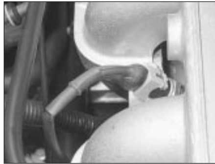
12.30 Fuel temperature switch wiring multiplug
