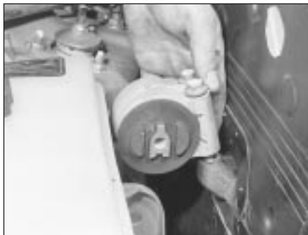
4.43 Remove the right-hand engine mounting
