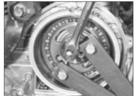
13.7 Use a tool like this to hold the camshaft sprocket as the bolts are undone
