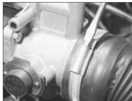
2.1 Disconnect the air trunking at the throttle housing
