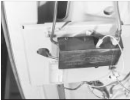
22.3 Aerial amplifier unit located under the rear parcel shelf on early Saloon models
