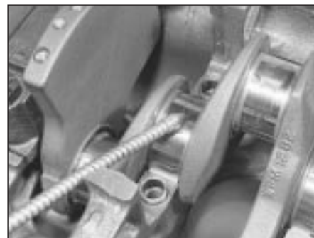
21.14 Thoroughly lubricate the crankshaft journals
