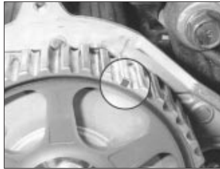
12.9b Rear camshaft sprocket timing notch, aligned with the corresponding line in the backplate
