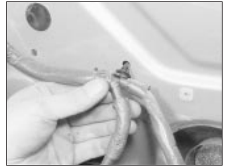
27.6a Release the wiring loom retaining clips . . .
