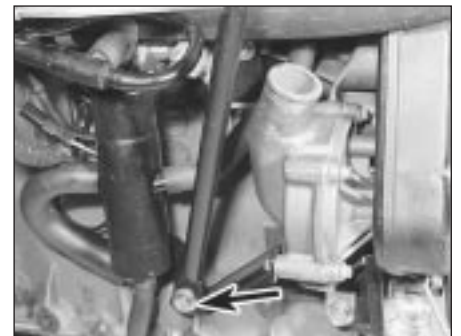
5.14 Undo the manifold stay bar lower retaining bolt (arrowed)
