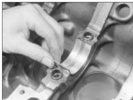
21.4 Fitting the main bearing shell upper halves
