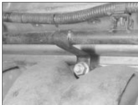
6.11 Undo the manifold nuts and bolts, noting that the upper nut also secures the bypass pipe bracket
