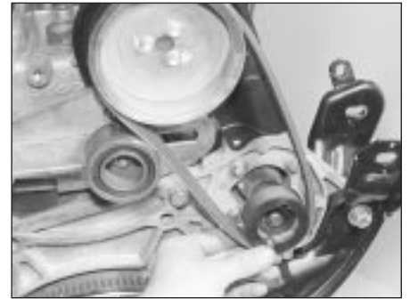
26.9 Withdraw the pulley and drivebelt from the pump
