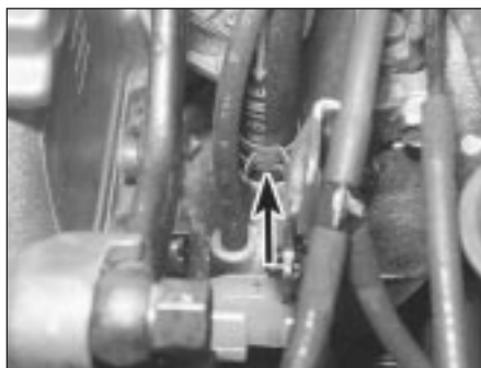
2.45 Disconnect the brake servo vacuum hose (arrowed) from the inlet manifold
