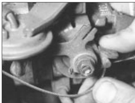
3.1 Slip the accelerator inner cable end out of the slot on the throttle lever
