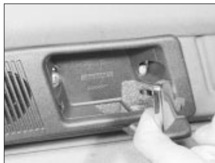
21.3b . . . and undo the trim surround screws
