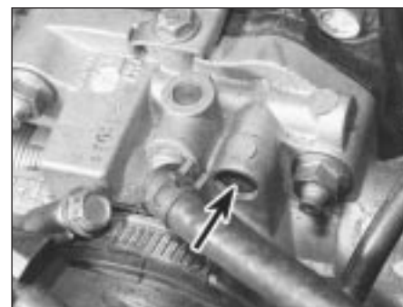
11.11 Idle speed adjustment screw (arrowed) on the idle valve. (On 2.5 litre engines the screw is on the side of the valve)
