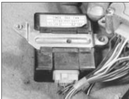
12.81 Where fitted, undo the two bolts and remove the cooling fan timer module
