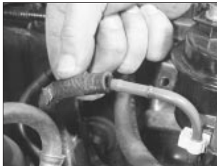
5.24 Disconnect the fuel return hose from the pipe below the fuel filter
