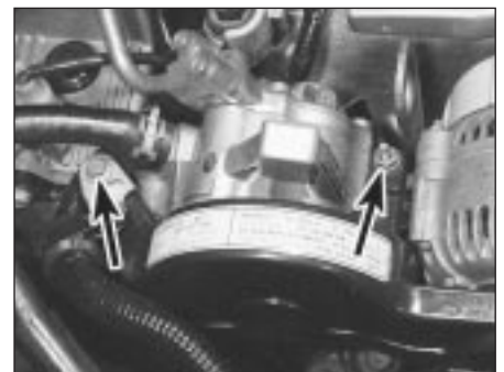
26.27a Undo the three nuts/bolts (arrowed) securing the pulley covers to the top of the engine . . .
