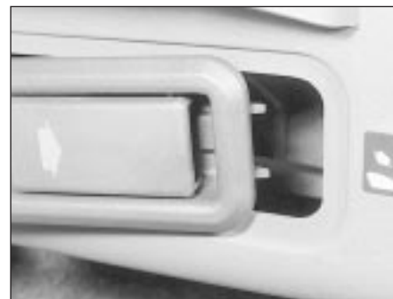
44.2b . . . and disengage the locating lugs
