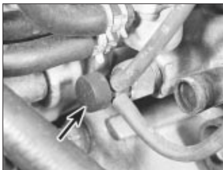
2.18 Disconnect the two vacuum hoses at the thermostatic valve (arrowed)
