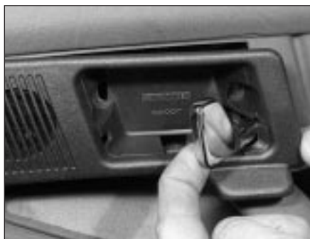
21.3c Manipulate the surround off the handle
