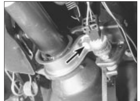
21.11 Steering column lower mounting bolt (arrowed)
