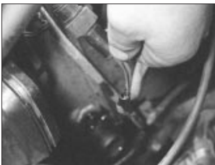
5.9 Disconnect the cooling fan multiplug at the wiring connector
