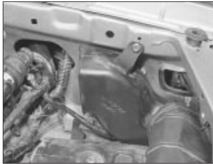
2.7 Side intake to body retaining bolt (arrowed)
