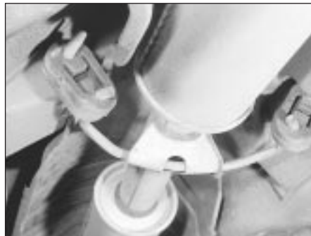
23.2 Typical exhaust system rubber mountings and brackets
