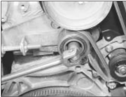
26.7 Slacken the tensioner wheel retaining nut
