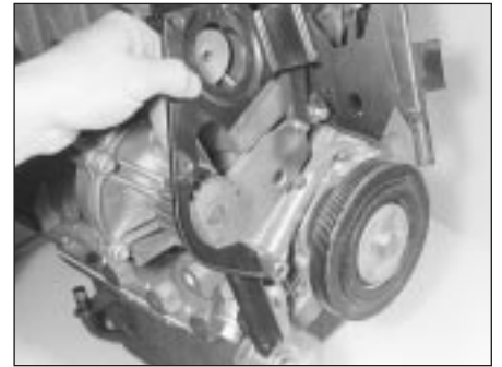
9.3 Removing the lower backplate from the engine (early metal version shown, later plastic version similar)
