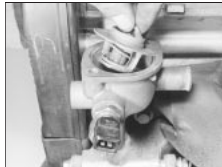
4.4 Withdraw the thermostat from the housing
