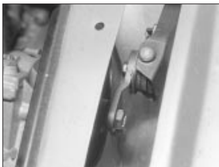
16.7 Undo the nut securing the linkage rotary link to the motor spindle
