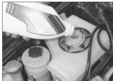
3.13 Topping up the cooling system
