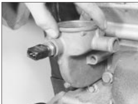
4.7 Removing the thermostat housing
