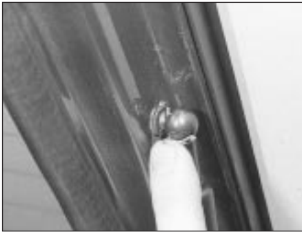
15.2a Extract the support strut wire spring retainer . . .
