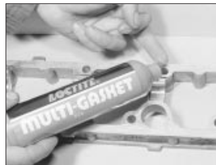
11.26 Apply sealant to the camshaft housing mating face
