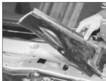
16.6b . . . and the left-hand side plenum moulding
