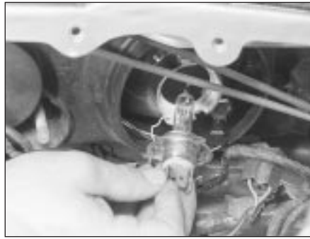
5.2 Release the wire clip and withdraw the bulb from the headlight unit
