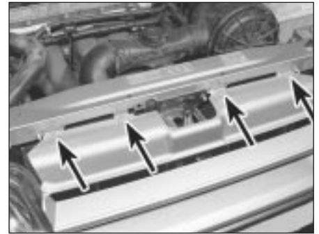
19.1 On early models, undo the radiator grille upper retaining screws (arrowed) . . .
