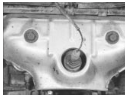
2.42 Rear oxygen sensor location in the exhaust manifold
