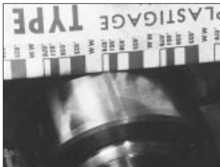
21.11 Measuring the width of the deformed Plastigage using the scale on the card provided
