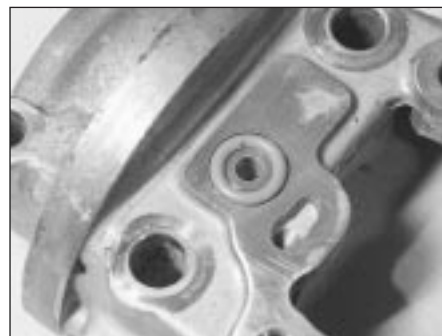
15.9 Recover the small O-ring seal in the camshaft carrier
