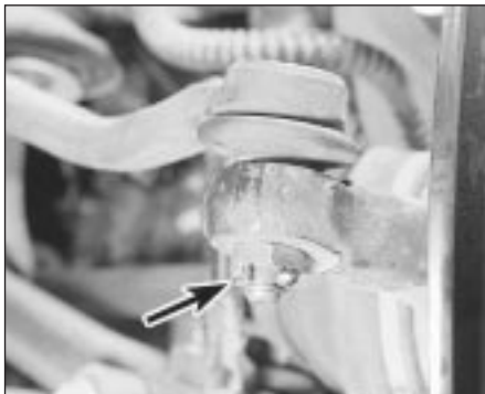
2.10 Extract the track rod balljoint nut split pin (arrowed)
