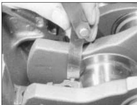
13.3 Checking crankshaft endfloat using feeler gauges
