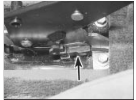
18.5 Disconnect the warning light switch wiring plug (arrowed)
