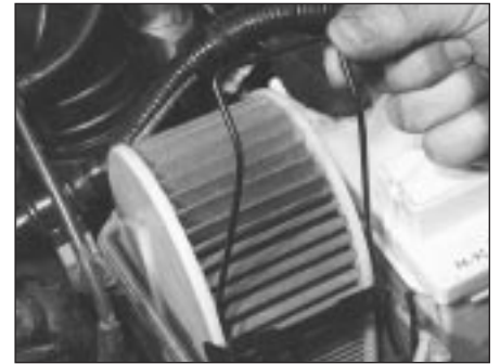
12.1c Lift the element out of the housing, together with its support frame on V6 engines
