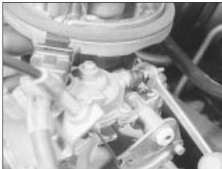
11.15a Slacken the base idle speed adjusting screw locknut . . .
