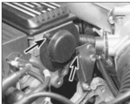
10.17 Undo the two bolts (arrowed) and remove the blanking plate
