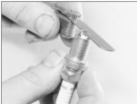
11.14a Measure the spark plug gap with a feeler gauge . . .
