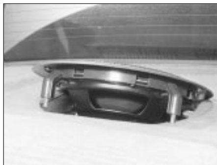
21.2 Removing the rear speaker from the parcel shelf
