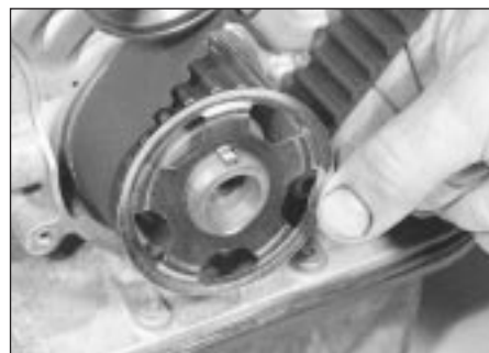
11.23 Remove the belt guide from the crankshaft sprocket
