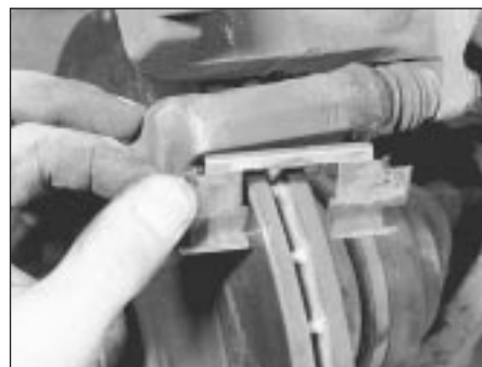
3.4b Remove the upper anti-rattle shim ...
