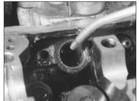
15.31a Fill the tappet bores with oil before fitting the tappets
