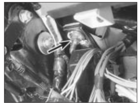
21.10 Steering column upper mounting nut (arrowed)
