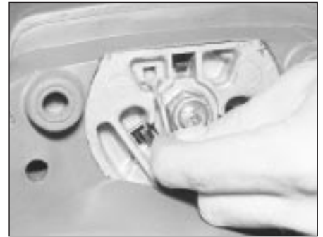
18.3b . . . and disconnect the two horn switch leads
