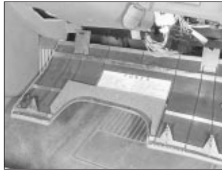
3.2b . . . noting the fuse identification on the rear of the panel
