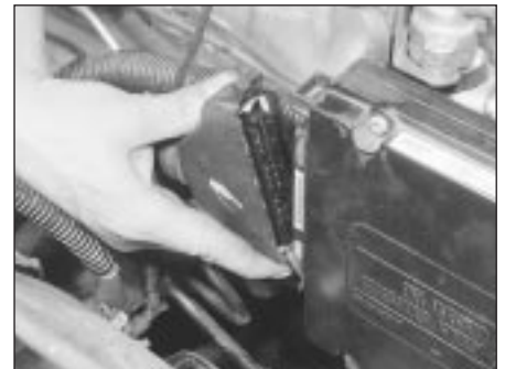
12.47 Disconnect the ECU wiring multiplug
