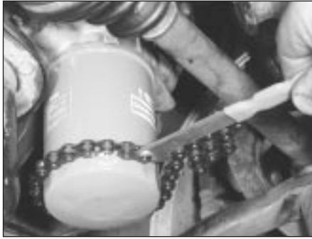
7.9 Using a filter removal tool, unscrew the oil filter from the housing
