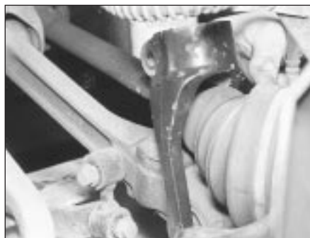
5.5 Removing the front suspension forked member
