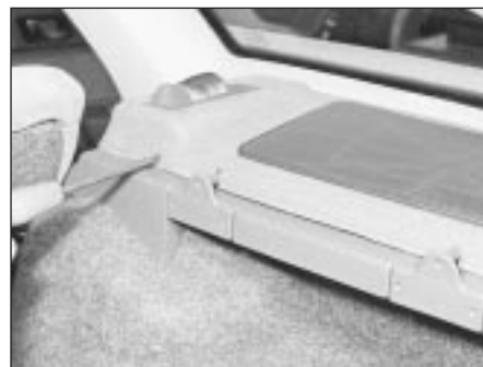
21.4 Remove the trim panel over the rear speaker on Fastback models
