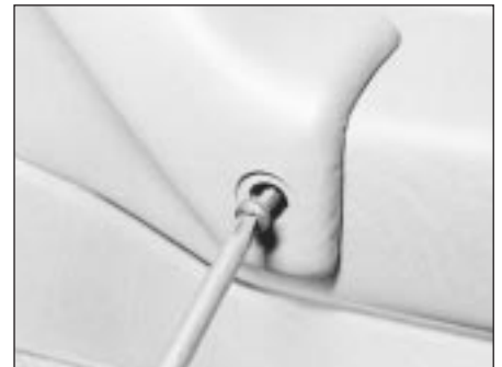
21.12b . . . and undo the recessed screw behind
