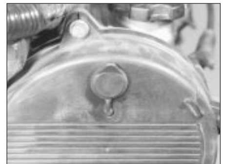
4.4 Remove the plastic plug from the viewing hole on each timing belt upper cover
