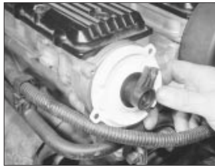
5.3a Where fitted, withdraw the plastic shield . . .
