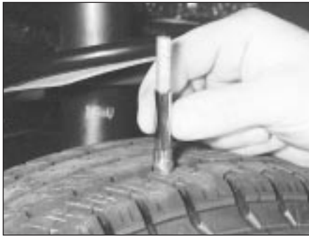
4.2 Checking the tyre tread depth with a depth gauge
