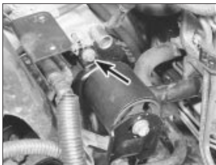
4.9 Undo the bolt (arrowed) securing the engine rear tie-bar support bracket to the inlet manifold
