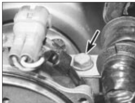
6.14 Undo the bolt (arrowed) and release the wiring harness from the side of the distributor body
