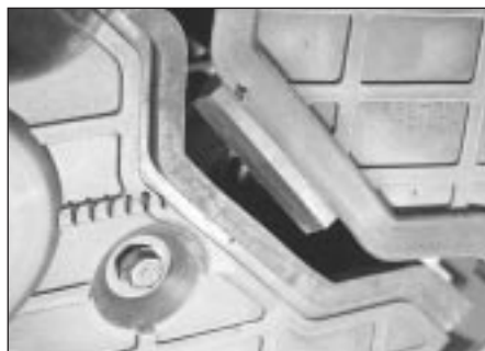
11.7 Ensure that the lip on the upper cover lower edge engages behind the lower cover
