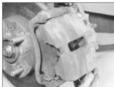
3.3 Pivot the caliper body upwards
