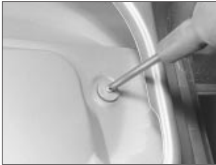
10.2 Undo the centre lens and reflector retaining screw
