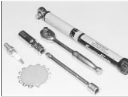
11.2 Tools required for spark plug removal, gap adjustment and refitting
