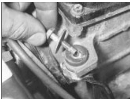
2.10b . . . and front bolt, securing the air cleaner assembly to the battery tray
