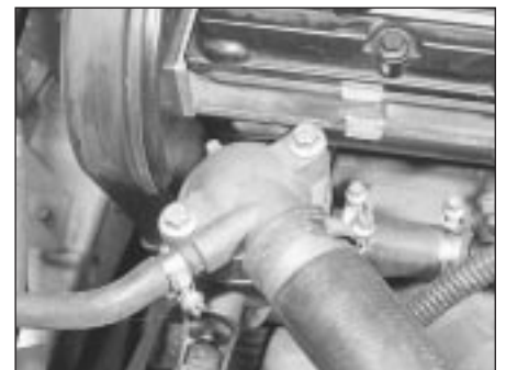
4.2 Detach the radiator top hose and expansion tank hose from the water outlet elbow
