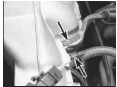
12.36 Vacuum hose connections at the throttle housing end of the plenum chamber
