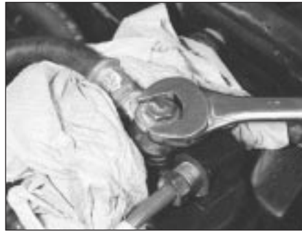
34.3b Unscrewing the banjo union bolt on V6 engines
