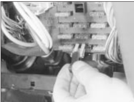
3.3b . . . to withdraw the fuses from their locations
