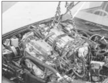
5.52 Removing the engine and transmission from the car
