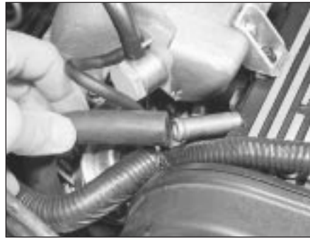
12.46 Detach the breather hose from the camshaft cover
