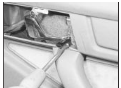
21.5 Undo the screw at the top of the door pull
