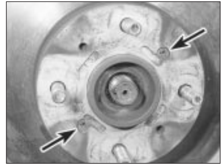
2.8 Brake disc retaining screws (arrowed)
