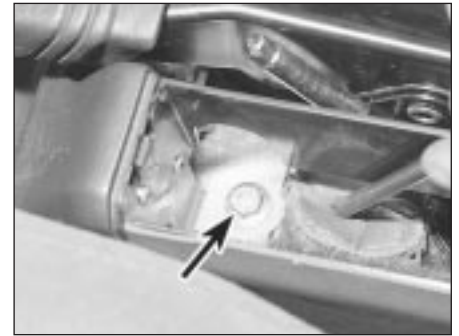
47.5 Console left-hand retaining bolt (arrowed)
