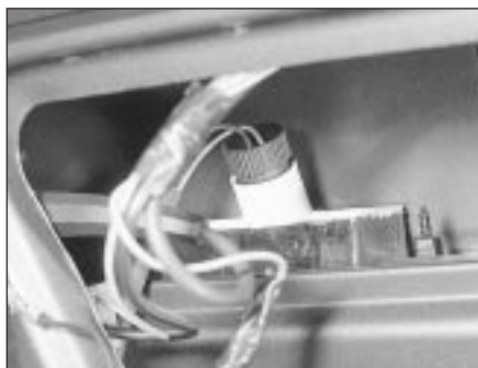
5.37 Number plate light bulbholder on early Fastback models
