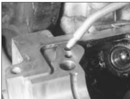
15.31b Prime the tappet oil feeds in the cylinder head with oil
