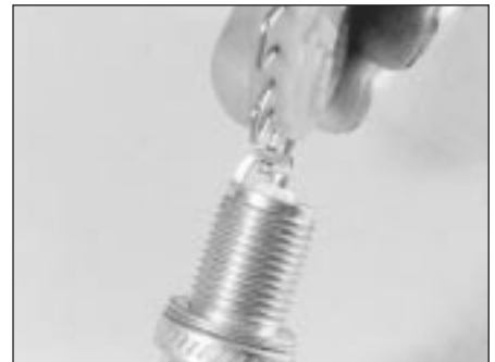
11.14c . . . then use the end of the special tool to adjust the gap
