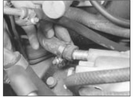
5.8 Disconnect the coolant hose from the right-hand end of the manifold
