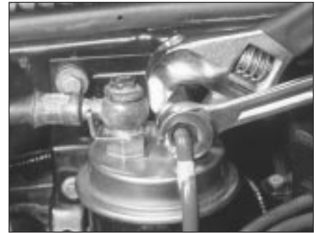
34.4 On V6 engines, unscrew the inlet union nut and withdraw the pipe from the filter head
