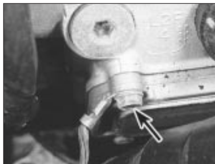
6.2 Engine earth lead (arrowed) on the upper front side cover bolt
