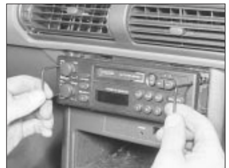
19.4 Withdraw the radio, using the tools to release the retaining clips
