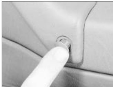
21.12a If the panel has a moulded door pull, prise out the blanking plug . . .
