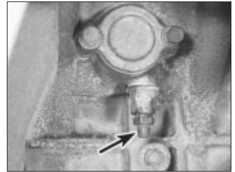
38.5 V6 engine cylinder block drain plug (arrowed)
