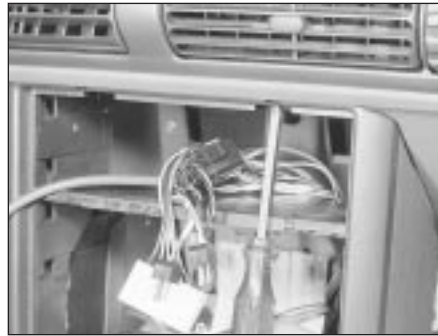
48.11a Undo the lower fascia upper screws . . .
