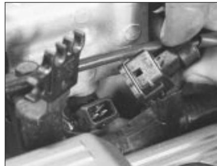
12.54 Disconnect the injector wiring multiplugs
