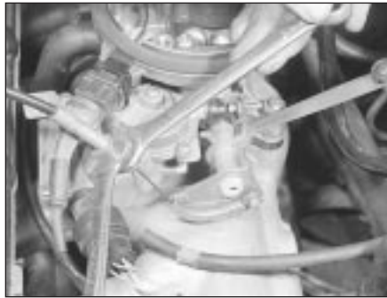
11.16b . . . and adjust the lost motion gap at the accelerator cable
