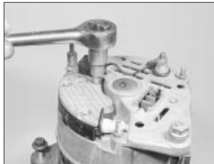
18.2 Undo the regulator and brushbox retaining screws
