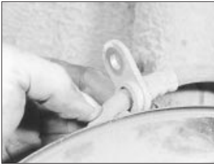
10.3 Release the rear flexible brake hose support clip from the suspension strut
