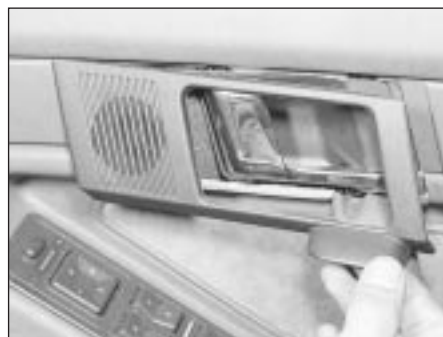
21.2a On early models, prise out the inner handle finisher trim . . .
