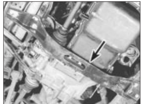
4.35 Undo the bolts and remove the longitudinal support member (arrowed)
