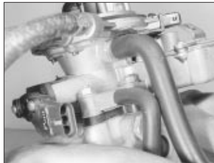
12.35 Breather hose attachments at the throttle body
