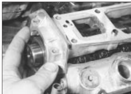
15.11 Lift the camshaft carrier off the cylinder head
