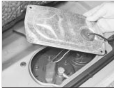
6.8b . . . and lift off the fuel pump access panel
