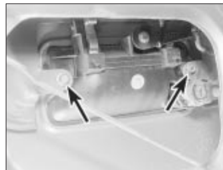
25.3 Front door exterior handle retaining bolts (arrowed)
