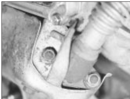
2.56 Undo the two nuts from the suction valve pipe front flange and release the heat shield
