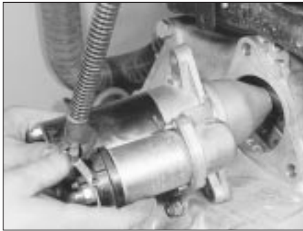
21.4 Removing the starter motor on 4-cylinder engines
