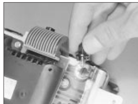
10.2b Instrument panel warning light bulb renewal
