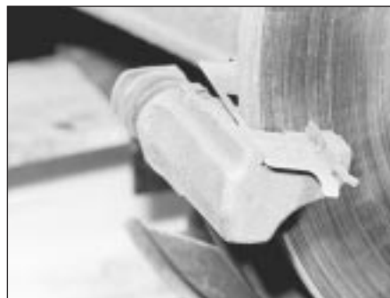
7.6c ... and lower anti-rattle shim
