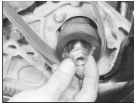
26.8 Unscrew the pump pulley retaining nut
