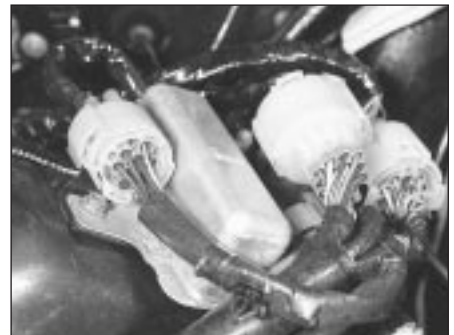
5.25 Disconnect the three wiring multiplugs at the rear of the engine compartment
