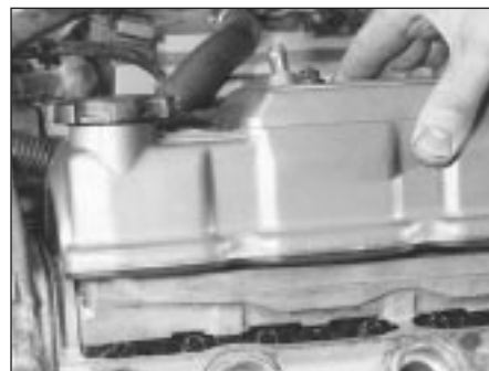
5.5 Lifting off the front camshaft cover
