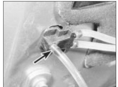
6.3 Disconnect the windscreen washer fluid feed hose (arrowed)
