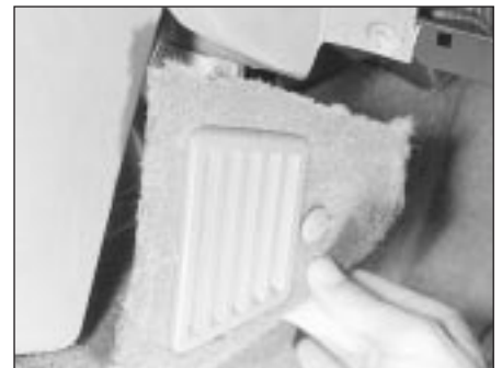
48.6 Withdraw the trim panel at the base of the lower facia
