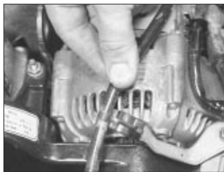
26.27b . . . release the pipes and cables from the support brackets . . .
