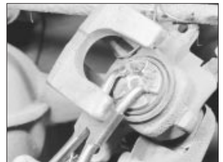
7.11 Using angled circlip pliers to screw the piston back into the caliper. Note the position of the cut-outs
