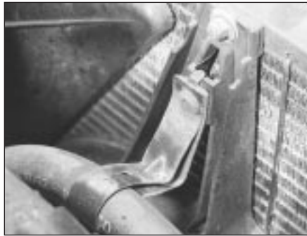
8.6 Undo the screw and release the hose support strap from the fan cowl
