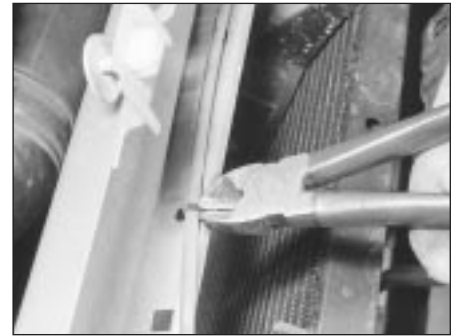
5.8 Cut off the cable ties securing the bonnet release cable
