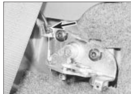
44.5 . . . and the clip at the locking mechanism (arrowed)
