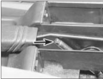
17.7 Handbrake adjuster location (arrowed)
