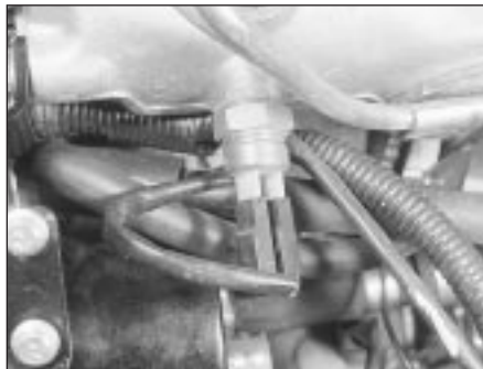
5.20 Disconnect the leads at the manifold heater temperature sensor
