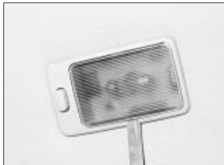
6.1 Prise off the courtesy light lens
