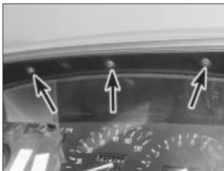
9.5 Undo the three cowl screws (arrowed) above the instrument panel . . .
