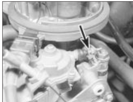
11.15b . . . and turn the adjusting screw (arrowed) to obtain the correct setting
