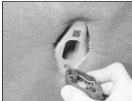
6.2 Remove the under-bonnet illumination light
