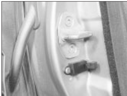
4.27 Courtesy light door pillar switch location
