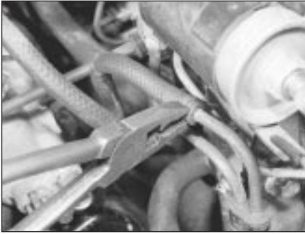
5.4 Release the hose clips and disconnect the two hoses from the fuel pipes
