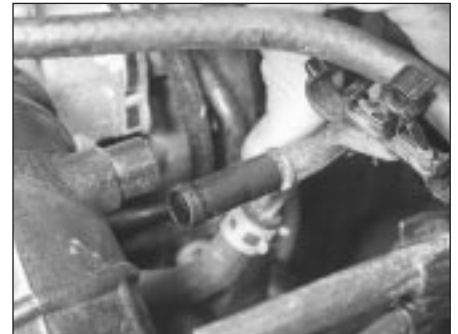
2.2 Remove the breather pipe from the side of the upper intake trunking
