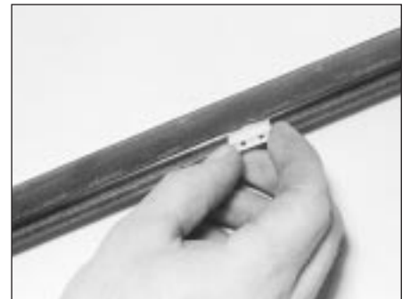
27.11 Position the waist seal retaining clips in the waist seal before refitting the seal to the door
