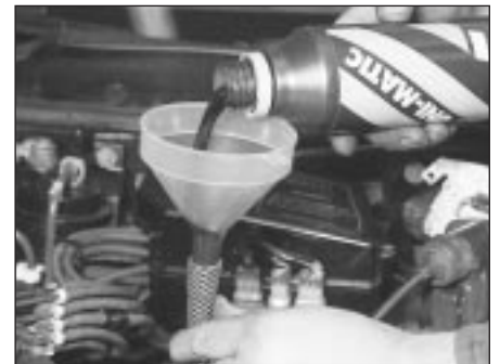
31.12 Add the specified automatic transmission fluid through the dipstick tube, using a clean funnel
