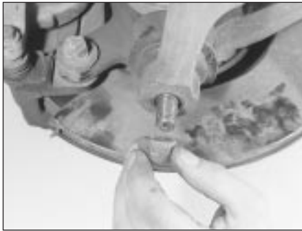
8.2 Undo the nut securing the steering knuckle balljoint to the lower suspension arm
