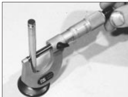
9.12 Measuring the valve stem diameter
