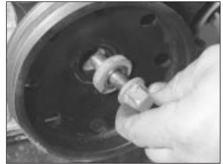
10.5 Remove the bolt and washer and withdraw the crankshaft pulley
