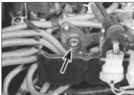
11.13a This is actually the ignition timing sensor/adjuster (arrowed) in the control box on 2.7 litre engines, but on 2.5 litre models, this is where you will find the idle mixture adjuster
