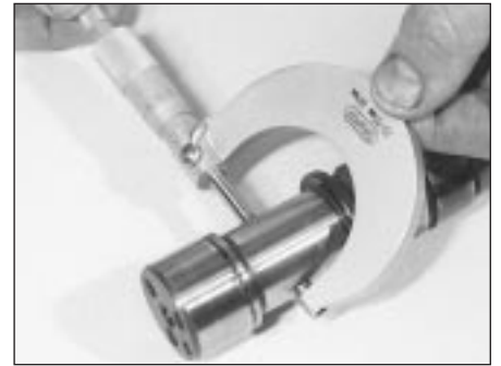
15.18 Measure the camshaft journal diameters using a micrometer
