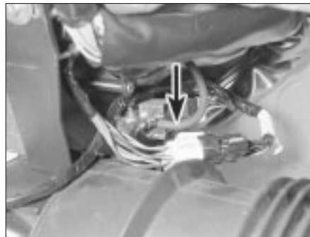
11.7 Solenoid vacuum hose (arrowed)
