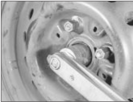
2.14 Tighten the new driveshaft retaining nut fully only when the weight of the car is on the roadwheels
