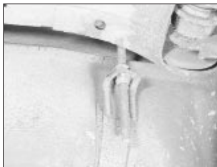
8.12 Fuel tank retaining strap and locknut
