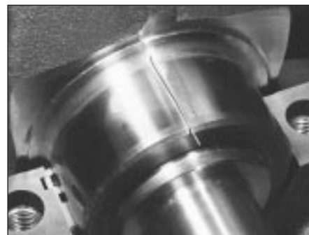
21.7 Plastigage in place on a crankshaft main bearing journal
