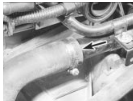
4.12a Disconnect the radiator hose (arrowed) at the main coolant pipe . . .
