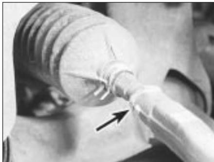
22.2 Steering track rod retaining locknut (arrowed)
