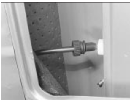
5.33 Number plate light bulbholder on early Saloon
