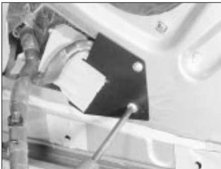
27.7 Undo the three screws and move the relay plate and relays aside
