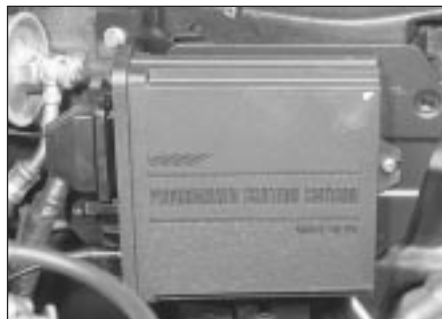
11.2 Ignition ECU location on the engine compartment bulkhead
