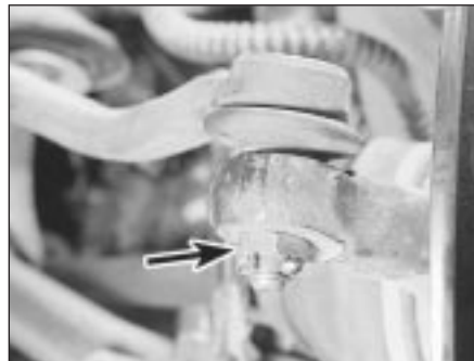
22.3 Extract the split pin and remove the track rod retaining nut (arrowed)
