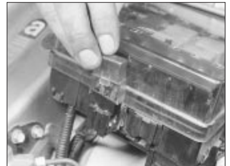
3.9 Additional fuse located under a cover on the outside of the fuse and relay box
