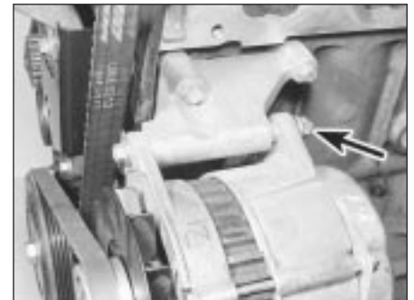
16.6b . . . and pivot bolt retaining nut on early "M" series 4-cylinder engines
