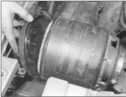
12.1a Removing the air cleaner cover . . .
