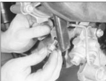
14.6 Undo the bolt securing the oil pipe retaining clip and timing belt backplate
