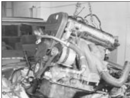
4.49 Removing the engine and transmission from the car
