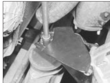
4.45 Undo the nut securing the front engine mounting
