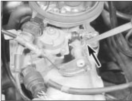
11.16a Insert a feeler gauge between the throttle lever and peg . . .
