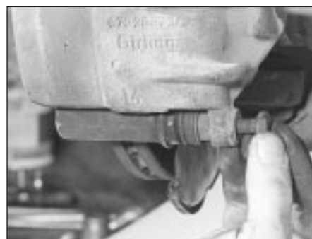
3.2b Unscrew the caliper lower guide pin bolt
