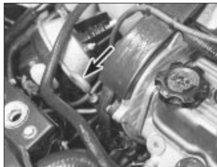
3.2 Engine oil dipstick location (arrowed) on V6 engines
