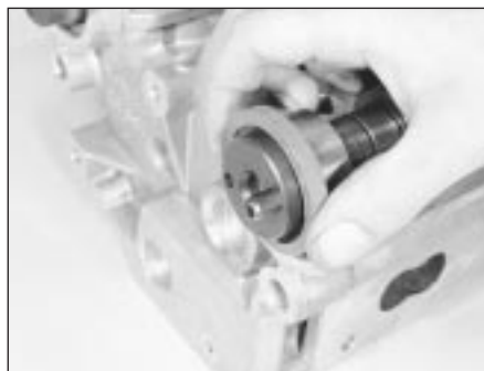
11.25 Fitting the camshaft oil seals
