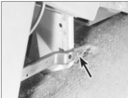
48.7 Undo the side brace retaining screws (arrowed)
