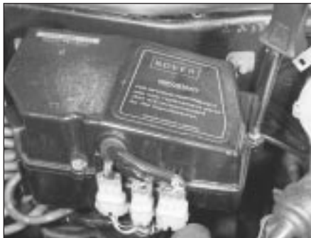
12.93 Undo the three screws and lift off the control box upper cover
