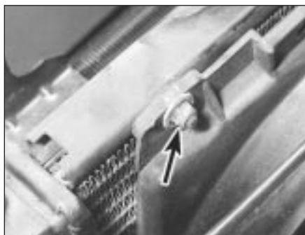
5.10a Cooling fan upper retaining nut (arrowed)
