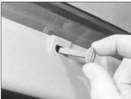
16.1 Release the screw studs and remove the tailgate inner trim panel
