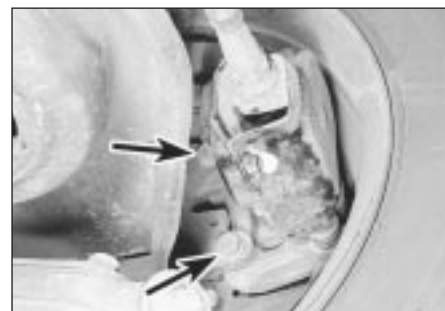
10.2 Carrier bracket-to-rear hub carrier retaining bolts (arrowed)
