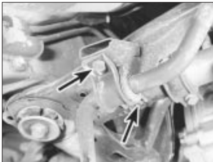
9.3 Anti-roll bar mounting bracket bolts (arrowed)
