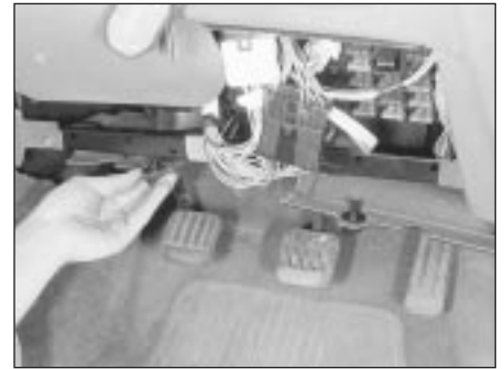
48.2 Remove the trim panel under the fascia
