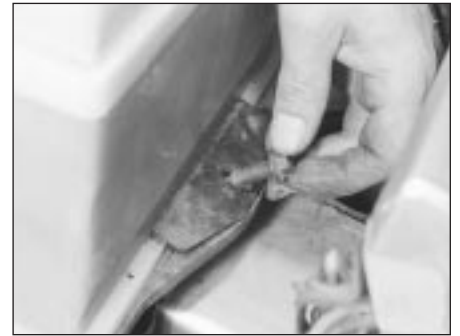
2.4 Removing the battery clamp retaining bolt
