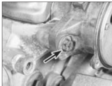
6.15a Undo the distributor retaining bolt . . .
