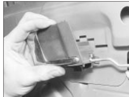
26.4 Withdraw the handle from the door
