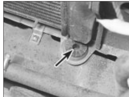
7.12a Ensure that the radiator lower lugs (arrowed) engage with the rubber grommets . . .
