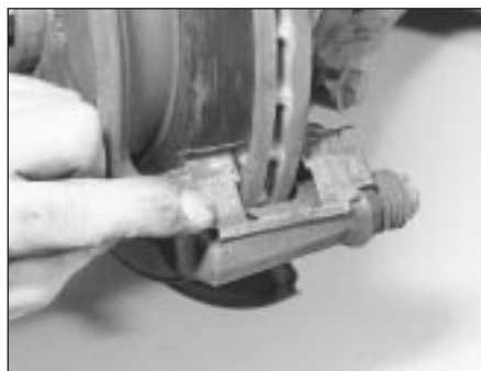
3.4c ... and lower anti-rattle shim
