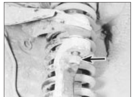
7.2b Undo the nut securing the upper arm balljoint to the steering knuckle (arrowed)
