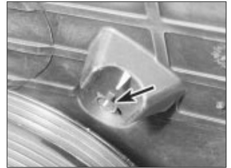
10.5 Highlight the pointer on the timing cover (arrowed) and the relevant pulley notch with white paint
