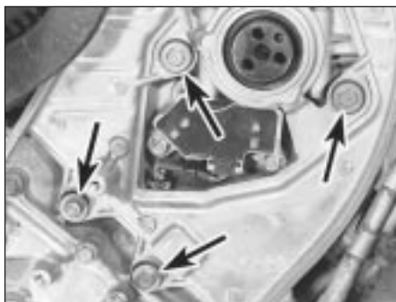
14.2 Front cylinder head backplate retaining bolts (arrowed)
