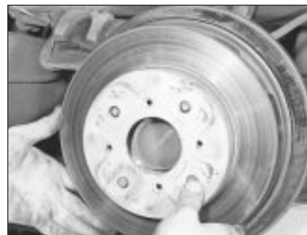
11.6b . . . and remove the brake disc
