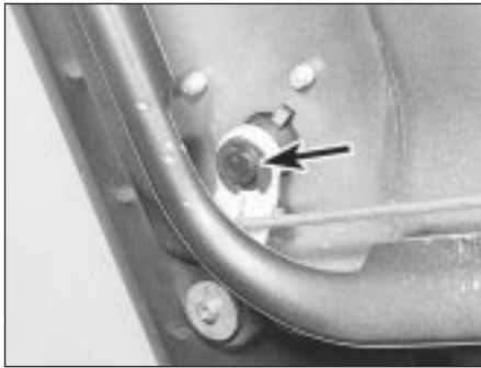
17.4 Private lock lever retaining circlip (arrowed) on early models
