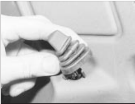
21.13a Release the rubber boot over the manual door mirror adjustment stalk . . .
