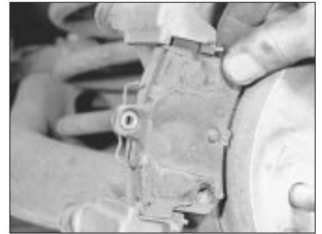
7.6a Lift out the two brake pads ...
