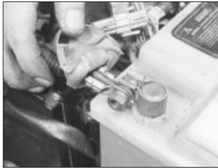
2.3 Lift off the plastic cover for access to the battery positive terminal
