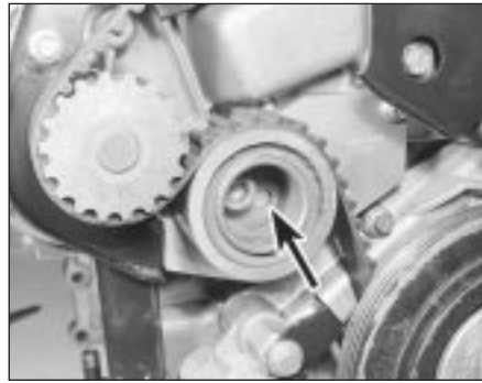
7.23 Tensioner hexagonal adjusting hole (arrowed)
