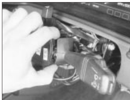
4.5a Depress the top and bottom switch retainers . . .
