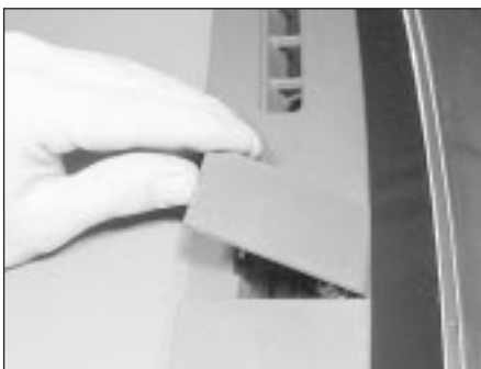
48.16 Lift up the centre cover plate and undo the bolt below the plate
