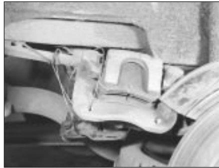
10.4 Tie up the caliper assembly to avoid straining the brake hose
