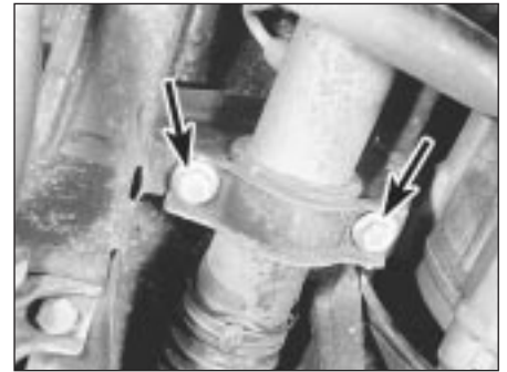
24.12b . . . and left-hand mounting bracket bolts (arrowed)
