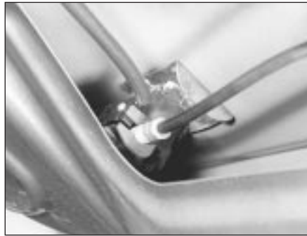
17.9 Private lock component attachments on later models
