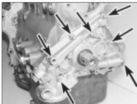
14.8 Oil pump housing retaining bolts (arrowed)
