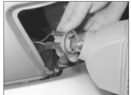
5.14 Withdraw the lens assembly and remove the bulbholder
