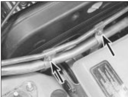
4.29 Undo the power steering pipe support bracket bolts
