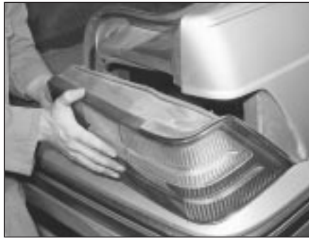
7.8b Removing the rear light cluster assembly
