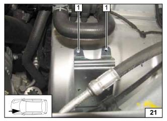
1 Copy hole pattern, 7 mm dia. hole [2x]
