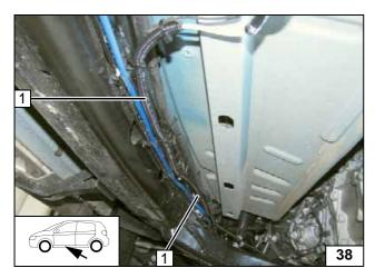
Route fuel line and wiring harness of metering pump in corrugated tube **1** to original vehicle lines at the installation location of the metering pump.
