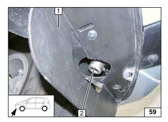
Install bumper 1. Align exhaust end section 2 to the back and flush on the bumper 1. Ensure sufficient distance from neighbouring components, especially from the exhaust system to the bumper, correct if necessary.
