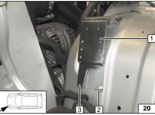
Bend bracket 1 according to the template, loosely install and align vertically.
