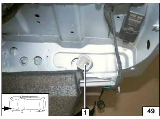
1 Exhaust-gas insulation in existing hole
