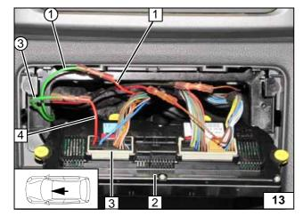
Connection to 20-pin T20a connector 3 Pin 20 from A/C control unit 2. Produce connections as shown in wiring diagram.
