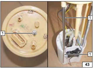
Shape fuel standpipe 1 according to template, cut to length and install.
