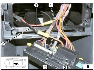
Connection of the 5-pin connector T5e **2** of the A/C control panel.
