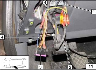
Connect the wiring harness of the fuse holder in passenger compartment 1 to the wiring harness of heater 2 according to the wiring diagram, with same colour wires connected to each other. Connection to OBD connector 3 terminal 15.
