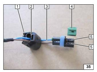
Complete connector of metering pump again after routing. Pin assignment is not relevant.
