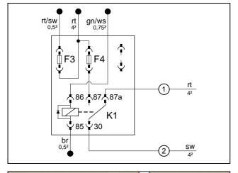
Install F4 25A fuse and K1 relay.
