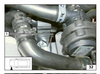
1 Connected wiring harness of circulating pump
