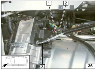
Insert fuel line 1 and wiring harness of metering pump 2 in corrugated tube 2100 and install in the engine compartment.
