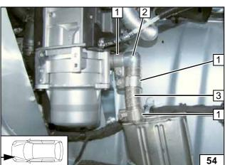
Ensure sufficient distance to wiring harness.
