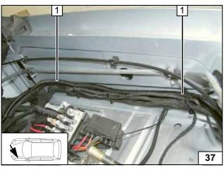
Route fuel line and wiring harness of metering pump in corrugated tube 1 to the firewall and further to the original vehicle lines of the underbody. Attach corrugated tube 1 with wiring harness of heater and earth wire on original vehicle wiring harness with cable ties.
