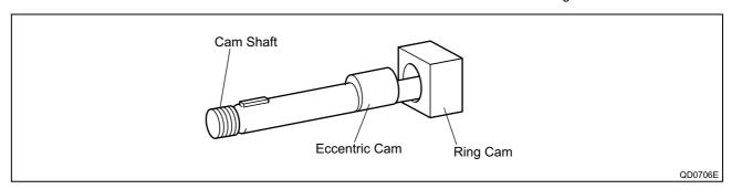
• As the cam shaft rotates, the eccentric cam rotates eccentrically, and the ring cam moves up and down while rotating.
