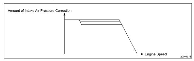
g. Amount of Injection Quantity by Atmospheric Air Pressure Correction
