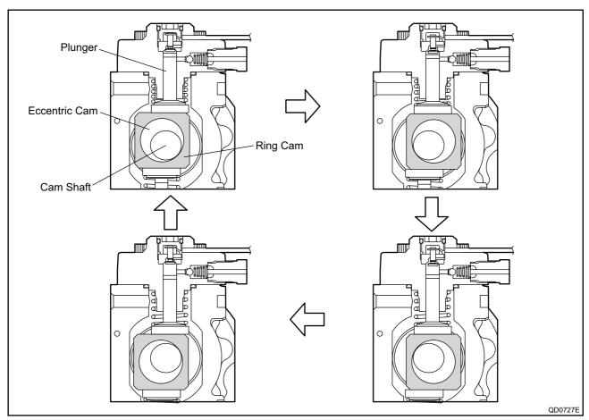
• The plunger and the suction valve are attached to the ring cam. The feed pump is connected to the rear of the cam shaft.
