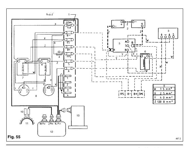
Starting circuit for 4012 engine range, read in conjunction with wiring diagram Fig. 57.
