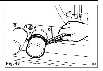
WARNING IT IS ESSENTIAL TO PRIME THE SYSTEM AFTER AN OIL AND FILTER CHANGE TO AVOID OIL STARVATION PROBLEMS, WITH AUTOMATICALLY STARTING GENERATOR SETS, WHICH TAKE FULL LOAD IMMEDIATELY AFTER STARTING.
