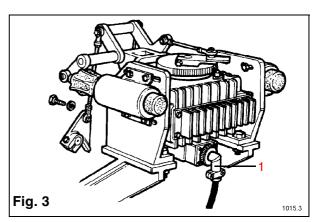
For earlier engines not fitted with a stop lever, disconnect the battery leads and remove the electric plug from the governor by unscrewing the locking collar and pulling the plug out of its socket. (See Fig. 2 & Fig. 3).
