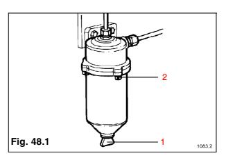
Open drain plug (1) to remove collected water and sediment. The plug is self retaining, leave open until clean fuel is seen then screw back in see page 41. Remove the bowl by unscrewing three screws (2). Clean thoroughly all components and dry with compressed air. Replace joint washer if damaged.
