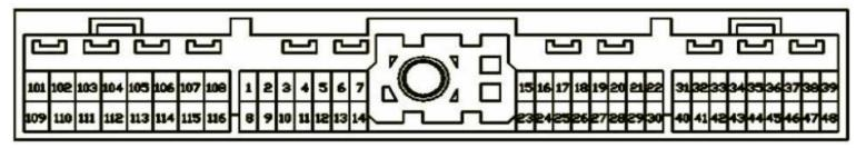
This pinout diagram can be used to install an SR20DET ECU into the factory wiring of a '95 Nissan Altima to run an SR20DET engine.
