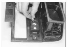
6.23 Removing the clock illumination bulb - models from 1993
