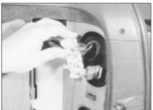
5.36a Removing a rear wing-mounted light bulbholder - Estate model
