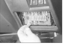
3.7 Removing a fuse using the plastic tool
