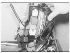
3.14c Main relay box located behind fusebox at rear of facia - models from 1993 (viewed with facia removed and inverted)
