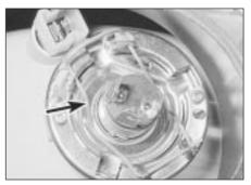
5.4a Release the spring clip (arrowed) . . .
