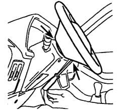
25.7 Turn the steering wheel for access to the two air bag unit screws (arrowed)
