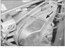
5.2 Headlight rear cover securing clip (arrowed)
