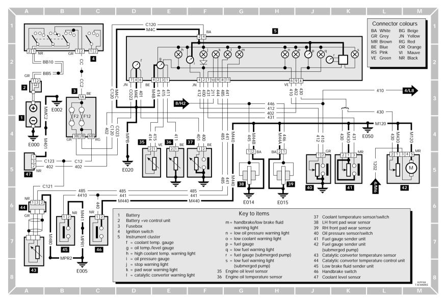
Diagram 5 : Warning lights and gauges - later models
