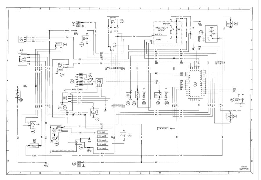
Diagram 1 : Typical starting, charging, ignition (XU52C/XU92C models only), cooling fan, warning lights and gauges - early models
