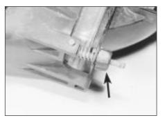
7.17 Unscrew the nut (arrowed) to separate the light from the cowl
