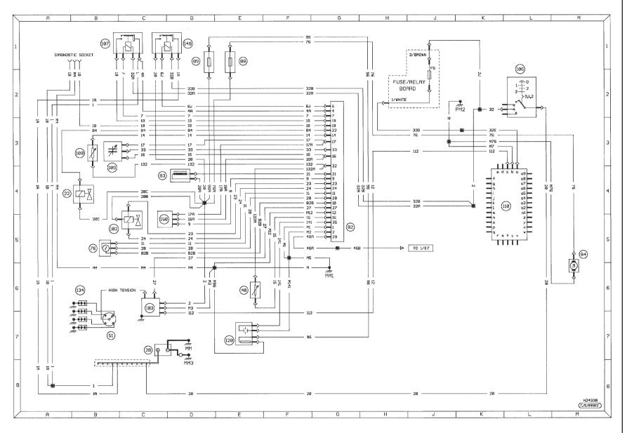
Diagram 1d : Typical fuel injection and ignition (XU9M/Z FENIX 1B) - early models
