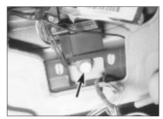
22.8 Roof-mounted radio aerial metal insulator (arrowed)
