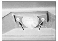
7.36 Number plate light securing screws (arrowed) - Saloon model
