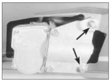
18.7 Tailgate wiper motor securing bolts (arrowed)
