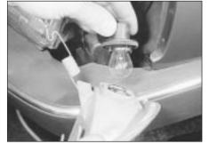
5.15 Withdrawing the bulbholder from the front direction indicator light
