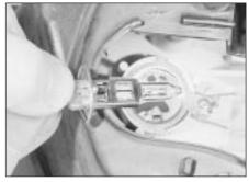
5.23b Removing a headlight-mounted driving light bulb
