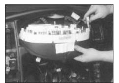
9.23 ... until the instrument panel can be withdrawn
