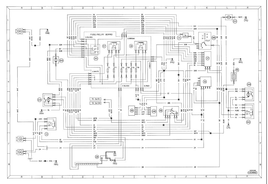
Diagram 3 : Typical ancillary circuits (wash/wipe, horn, heater blower and heated rear window) - early models
