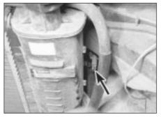
8.2b Headlight beam horizontal fine adjuster (arrowed)
