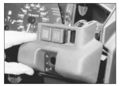
9.6 Withdrawing the driver's side upper facia panel
