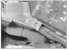
9.7 Remove the upper centre facia panel securing screw
