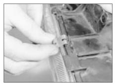
7.9 Removing a headlight lens securing clip
