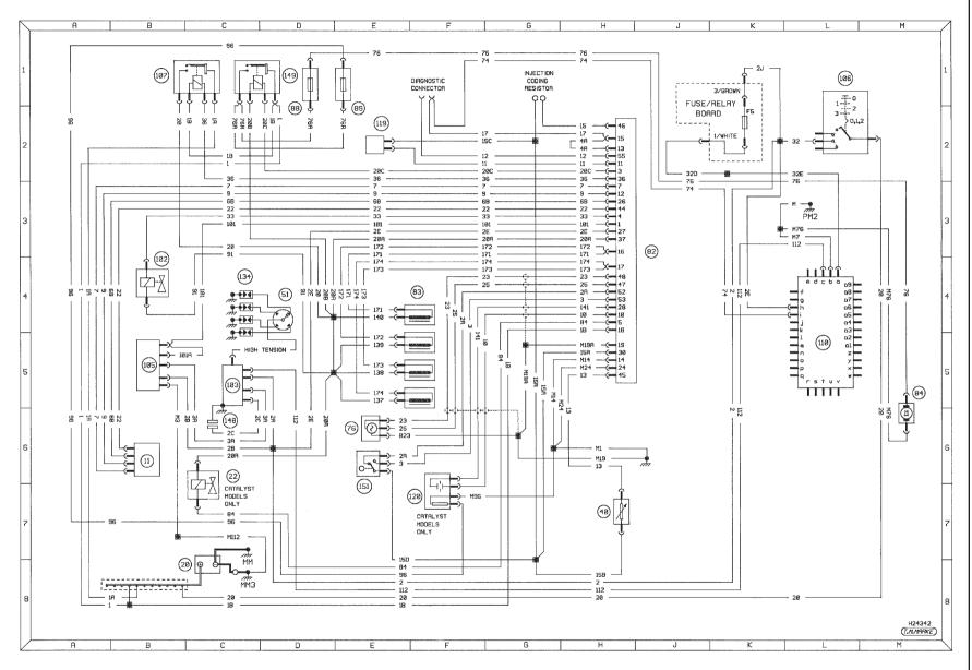
Diagram 1g : Typical fuel injection and ignition (XU9J4 and XU9J4/Z M1.3 Motronic) - early models
