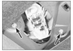
7.34c Tailgate-mounted rear light cluster securing nuts (arrowed) - Estate model
