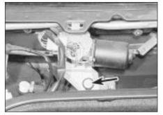
17.8a Windscreen wiper motor securing nut (arrowed)
