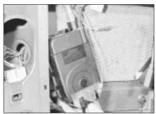
22.18c ... and withdraw aerial assembly -Estate (rear wing-mounted aerial)
