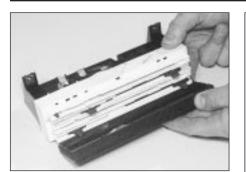
6.19 Unclip the front panel from the heater control unit
