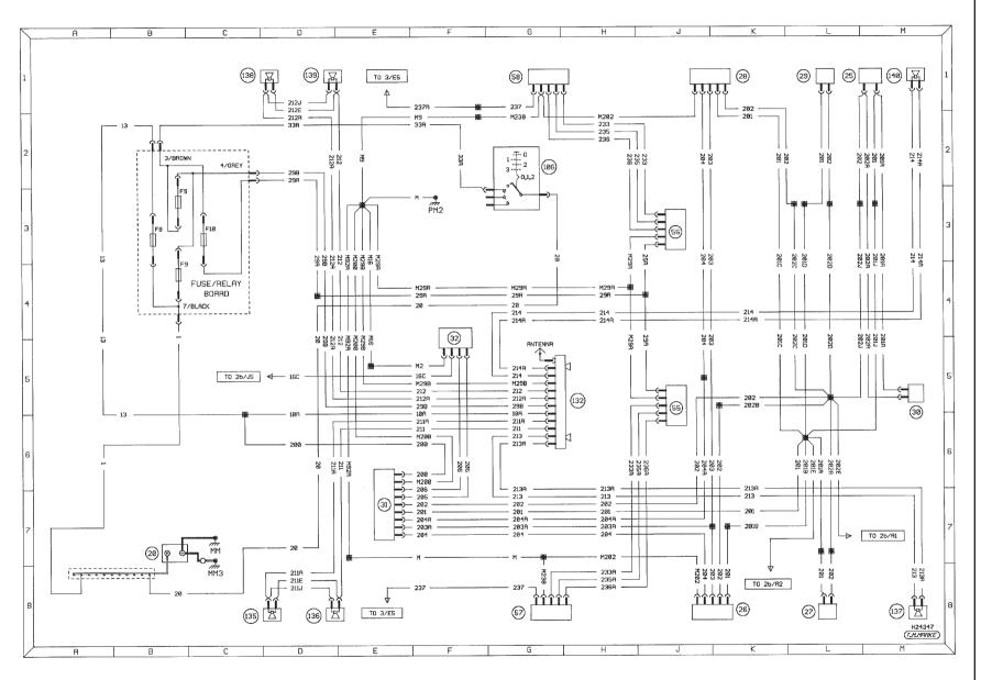
Diagram 3a : Typical ancillary circuits (central locking, electric door mirrors and radio/cassette) - early models
