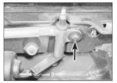
17.8b Windscreen wiper linkage securing nut (arrowed)
