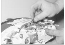
6.27 Removing an instrument panel illumination bulb
