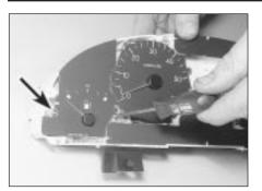
10.10 Remove the gauge securing screws . . .
