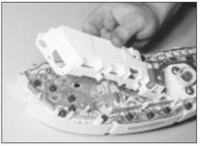
10.8 Removing the cover from the rear of the instrument panel
