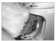
7.8 Outer headlight securing bolts (arrowed)
