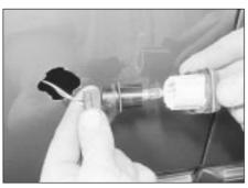
5.20 Removing the bulbholder from the front direction indicator side repeater light
