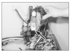
13.3 "Lights on" warning buzzer (arrowed)
