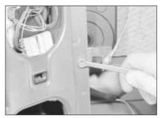
22.18b Unscrew the aerial motor securing bolt . . .
