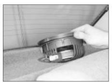
21.13 Removing the rear loudspeaker -Saloon models
