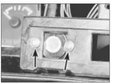
8.10 Headlight adjuster switch securing screws (arrowed)
