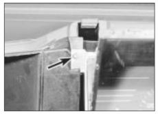
9.8 Instrument panel securing screw (arrowed)
