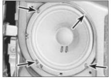
21.3 Door-mounted loudspeaker securing screws (arrowed)
