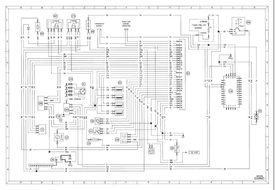
Diagram 1f : Typical fuel injection and ignition (XU9JA/Z M1.3 Motronic) - early models
