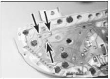
10.9 Fuel gauge securing nuts (arrowed)
