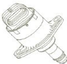
Diagram of Step motor
