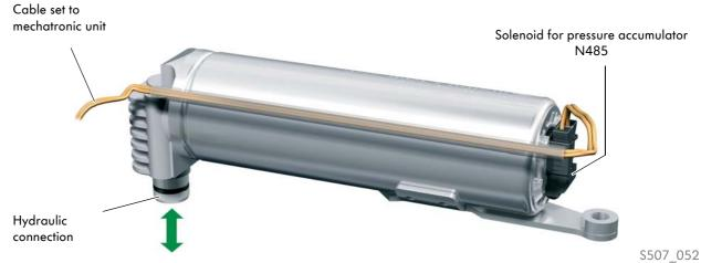
The hydraulic pulse accumulator has a useful volume of about 100 cm<sup>3</sup>.
