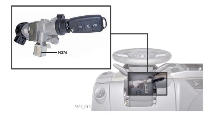
The ignition key removal lock prevents the ignition key from being removed when the parking lock is not engaged. It functions electromechanically and is locked in "P" by the selector lever switch F319.
