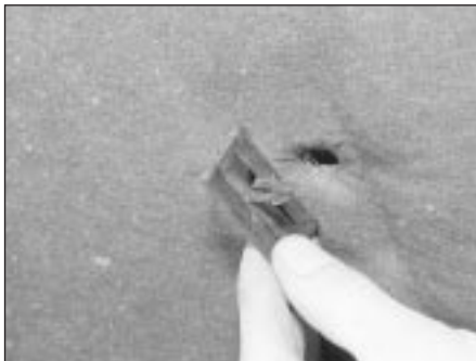
6.1 Remove the sound-deadening material by releasing the clip retainers
