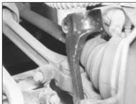
5.5 Removing the front suspension forked member
