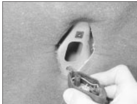
6.2 Remove the under-bonnet illumination light
