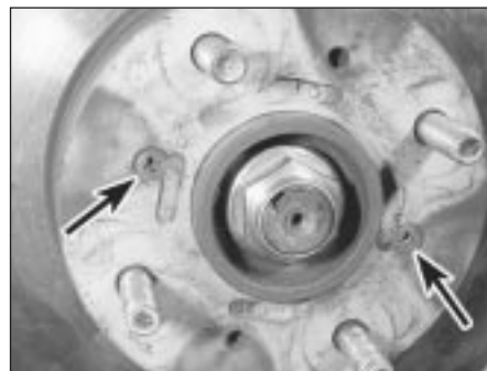
6.9a Undo the two retaining screws (arrowed) . . .
