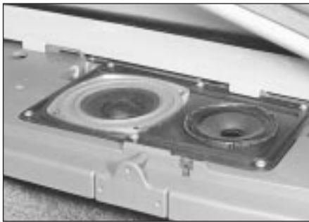
21.6 Undo the six screws and remove the speaker assembly
