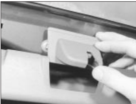
16.3 Remove the plastic cover from the lock
