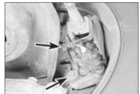
10.2 Carrier bracket-to-rear hub carrier retaining bolts (arrowed)
