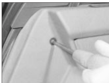
21.8 Undo the screw at the front corner
