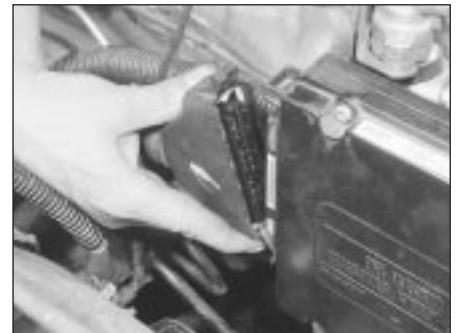
12.47 Disconnect the ECU wiring multiplug
