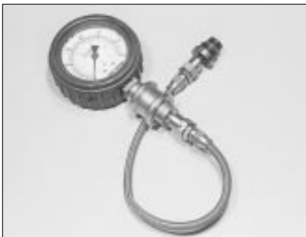
Compression testing gauge
