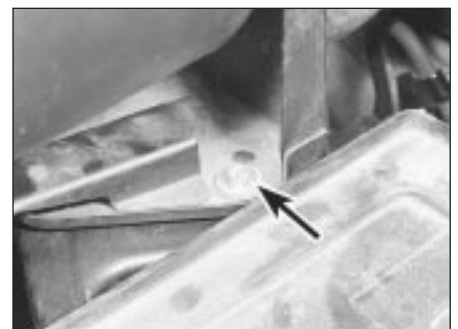
2.5b . . . right-hand retaining bolt . . .
