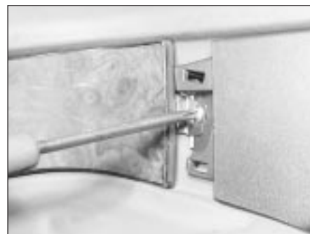
9.3b . . . and undo the screw behind
