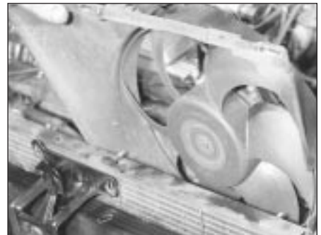
5.10b Removing the cooling fan assembly
