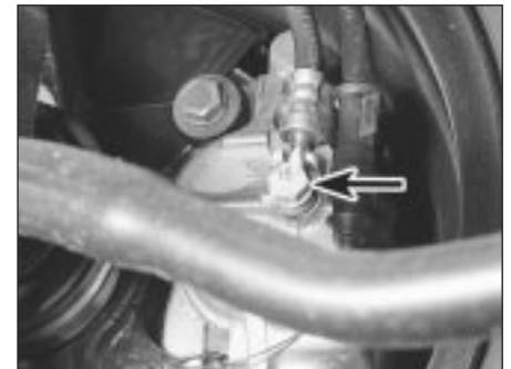
15.10 Front brake hose-to-caliper banjo union bolt (arrowed)
