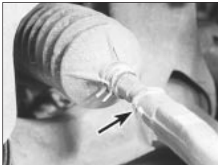
22.2 Steering track rod retaining locknut (arrowed)
