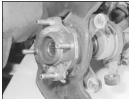
2.13 Withdrawing the steering knuckle from the driveshaft
