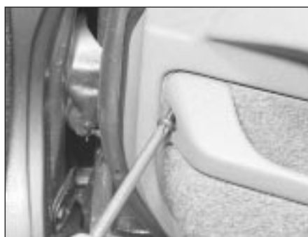
21.9a Undo the storage bin front screw . . .
