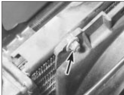
5.10a Cooling fan upper retaining nut (arrowed)
