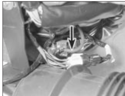
11.7 Solenoid vacuum hose (arrowed)
