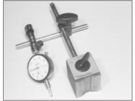
Dial test indicator and magnetic stand
