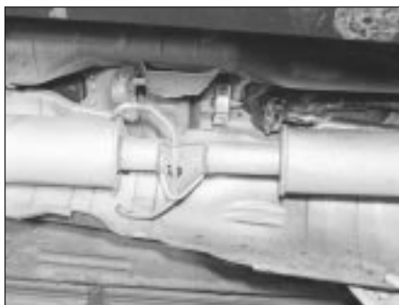
19.3 Removing the front heat shield from the exhaust system
