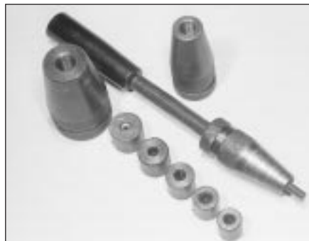
Clutch plate alignment set
