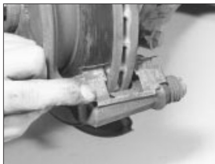
3.4c ... and lower anti-rattle shim
