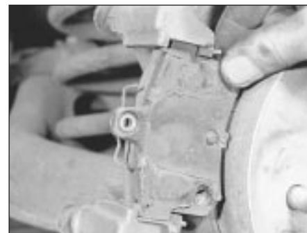
7.6a Lift out the two brake pads . . .
