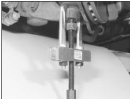
2.11 Using a two-legged puller to release the steering knuckle balljoint
