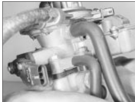
12.35 Breather hose attachments at the throttle body
