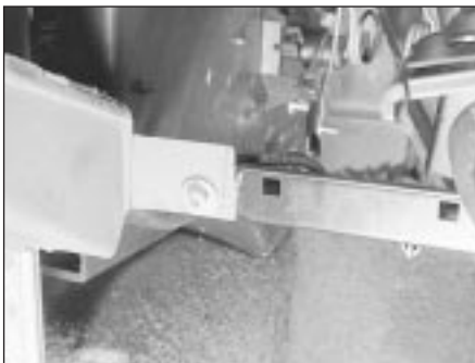
48.13 Undo the cross-brace screws
