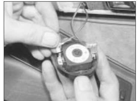
21.16 Disconnect the wiring and remove the tweeter
