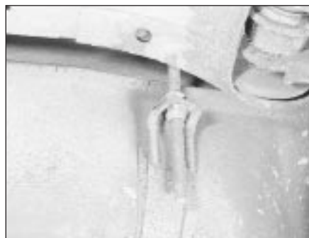
8.12 Fuel tank retaining strap and locknut
