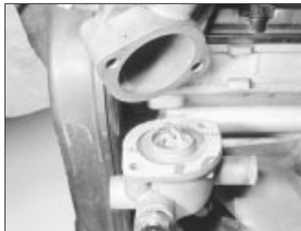
4.3b ... and remove the water outlet elbow
