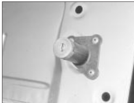
10.4 Boot lid private lock retaining rivets
