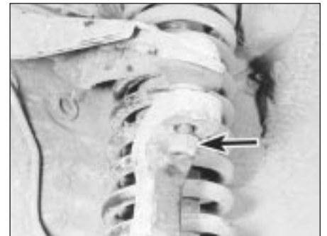
7.2b Undo the nut securing the upper arm balljoint to the steering knuckle (arrowed)
