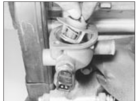
4.4 Withdraw the thermostat from the housing
