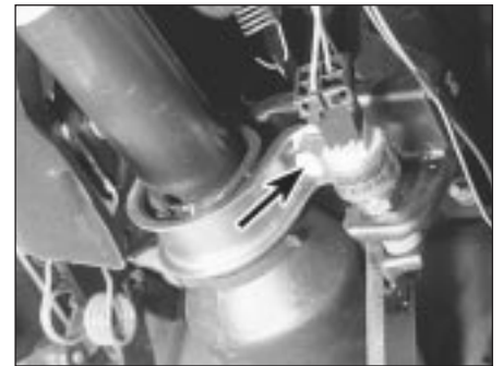
21.11 Steering column lower mounting bolt (arrowed)
